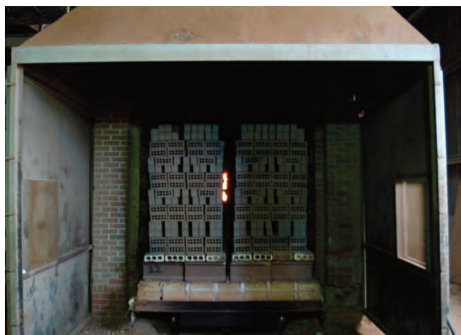
Figure 21 Modern gas-fired tunnel brick kiln (courtesy US Brick Industry Association)
