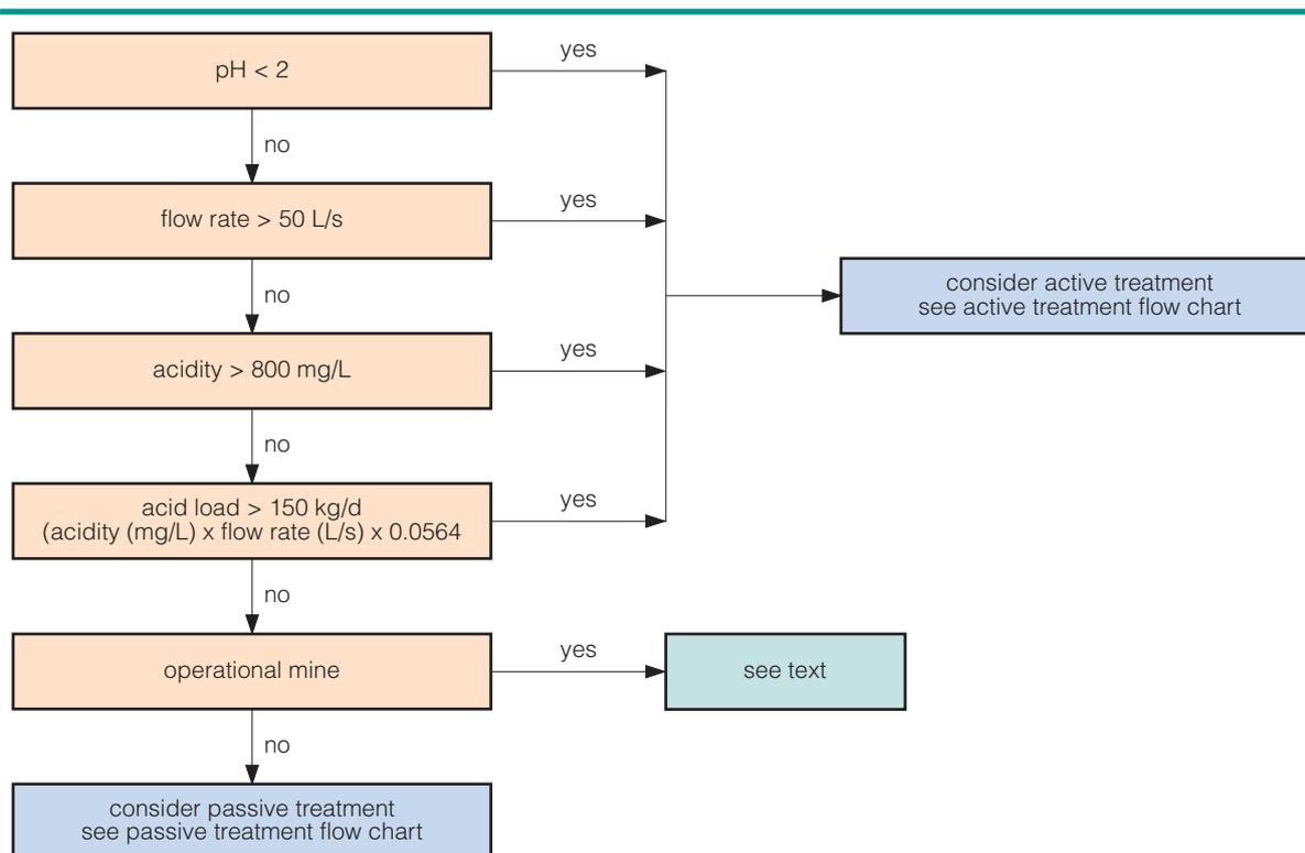
**Figure 12 Flow chart to guide selection between active and passive treatment for AMD**
