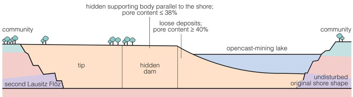
**Figure 20 Hidden dam to secure tipped slopes endangered by liquefaction slumps (Kuyumcu, 2011)**
