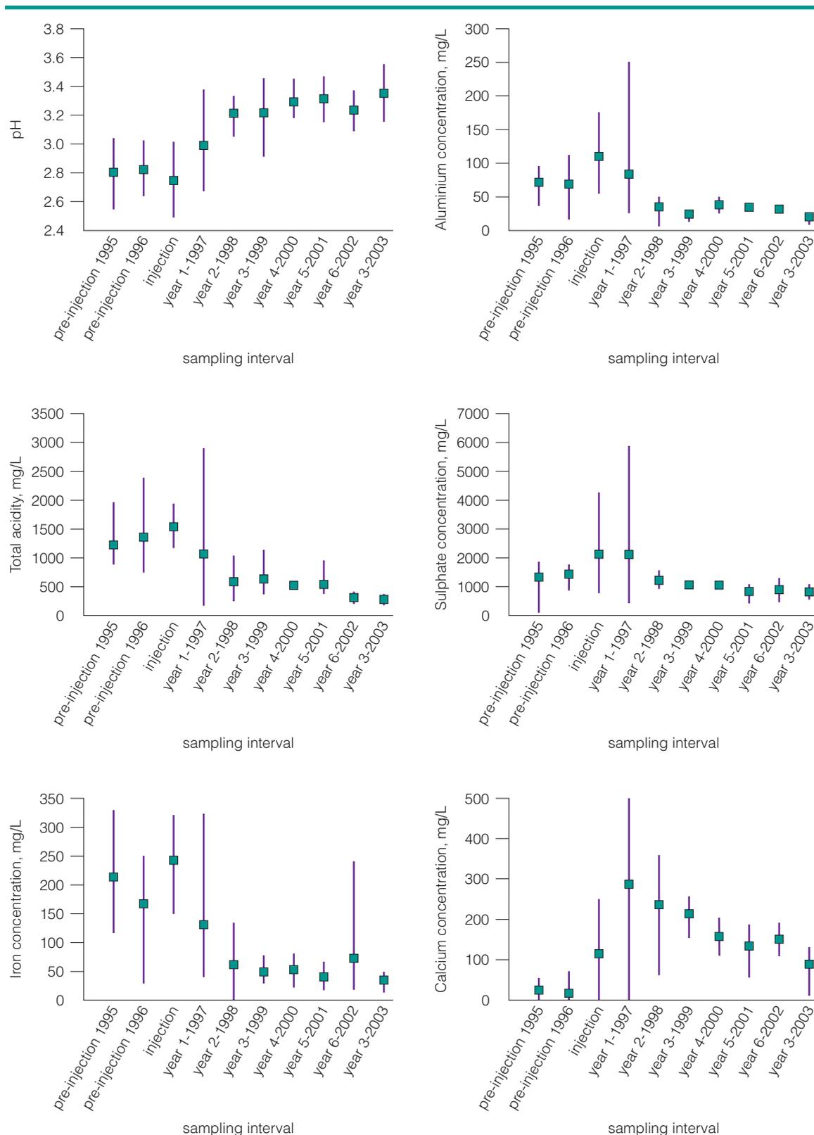
**Figure 14 Concentrations of various acid mine drainage parameters before and after placement of the grout (Bulusu and others, 2005)**
