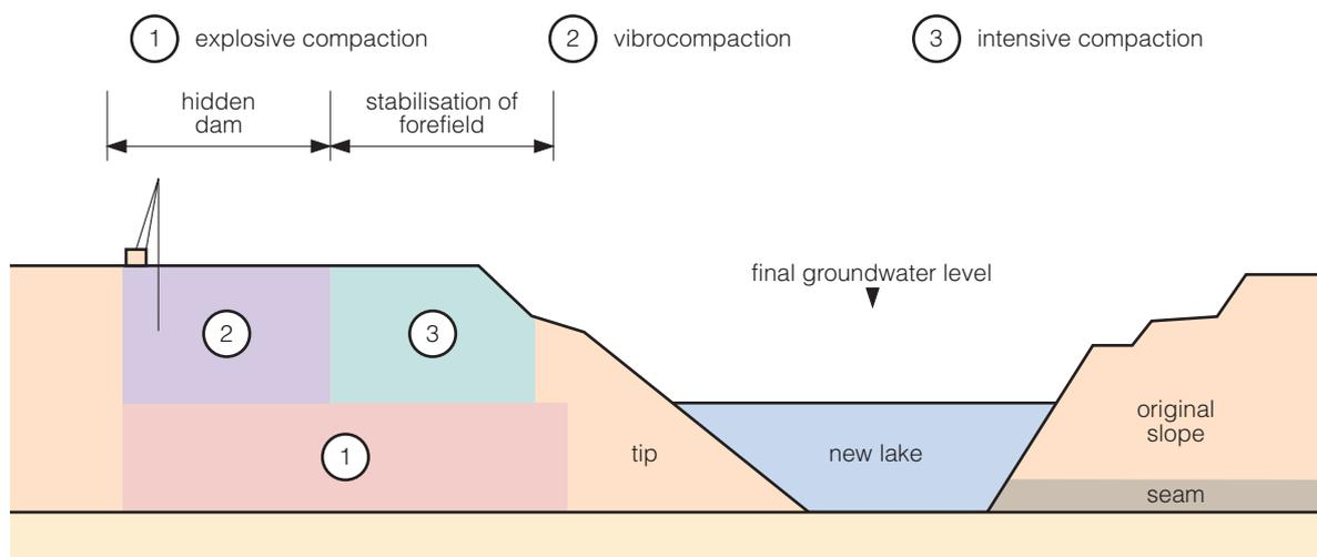
**Figure 21 Combination of methods for compaction (Kuyumcu, 2011)**
