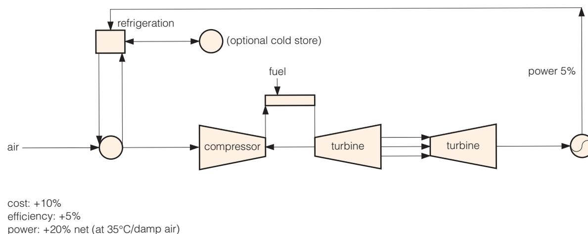
**Figure 12 Principle of inlet chilling by refrigeration (Mee, 1999)**
