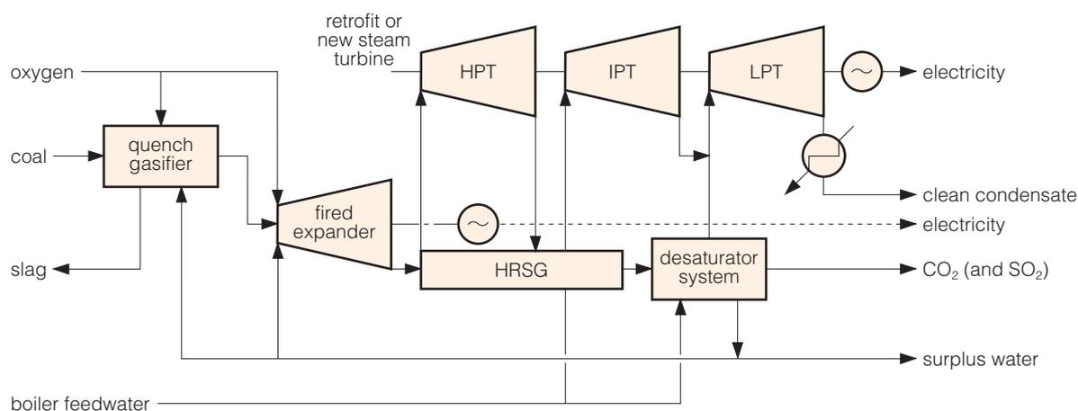
**Figure 32 Schematic of Integrated Gasification Steam Cycle** (Griffiths, 2009)
