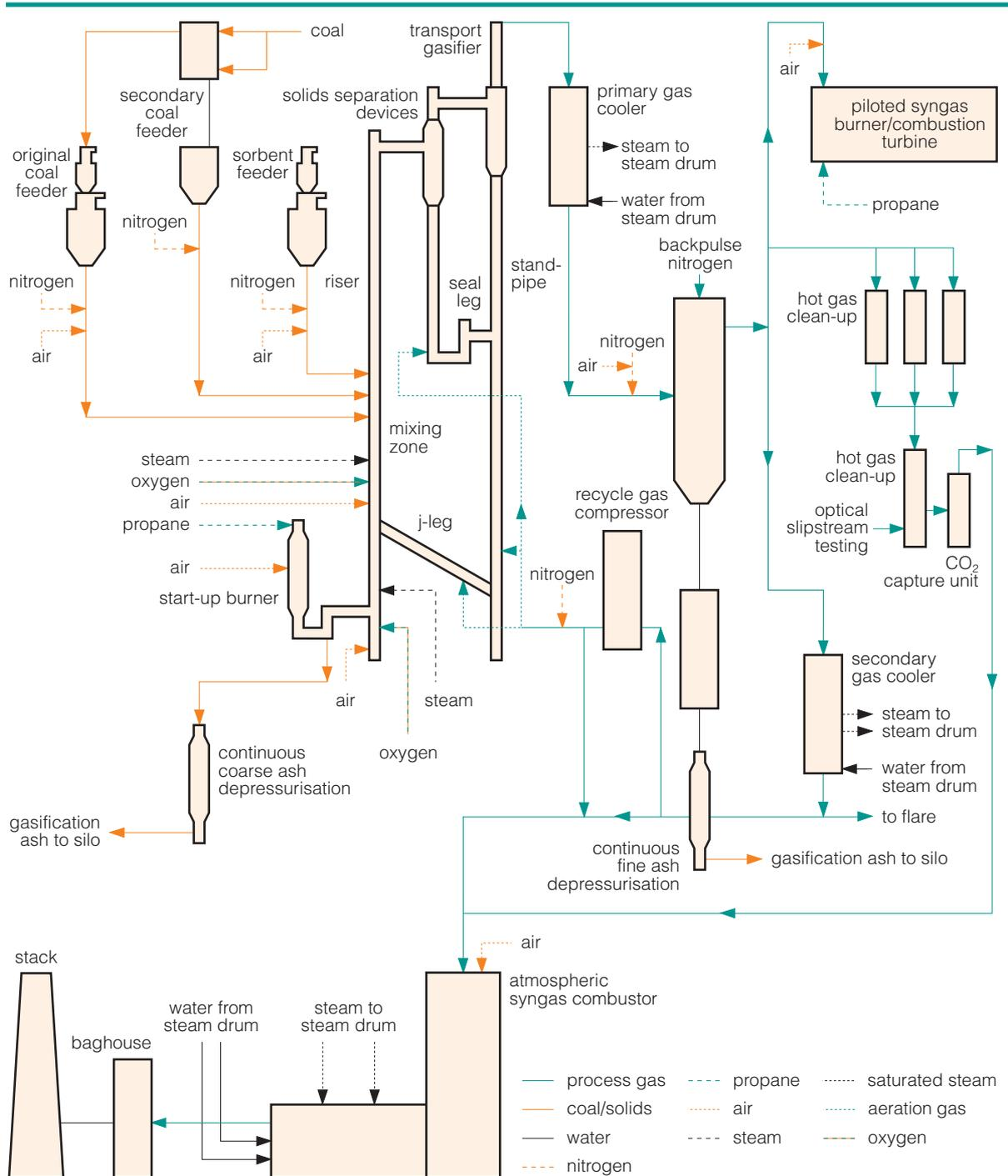
**Figure 38 Transport gasifier gasification process flow diagram**
