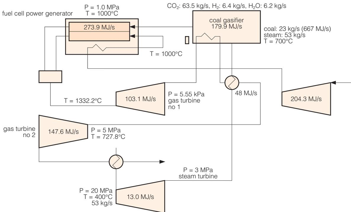
**Figure 17** Schematic drawing of a basic A-IGFC process (Iki and others, 2009)
