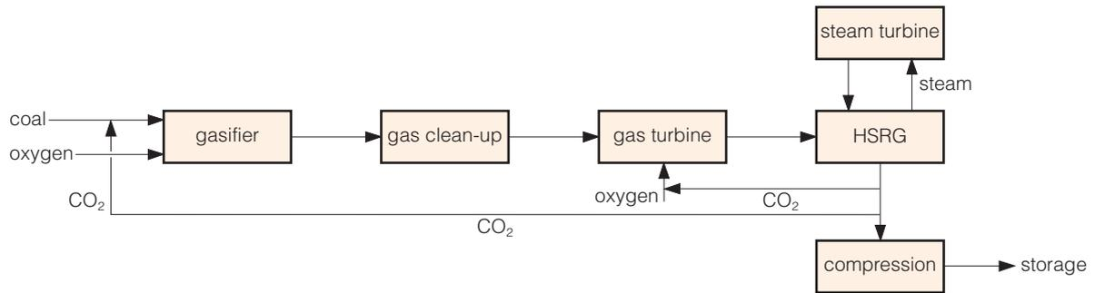
**Figure 24** Concept of newly proposed 'Oxy-fuel IGCC' (Oki and others, 2011)
