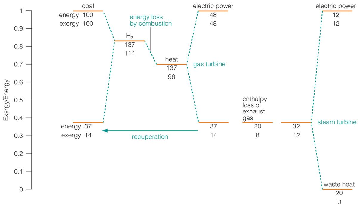
Figure 18 Energy flows in IGCC with recuperation (Iki and others, 2009)
