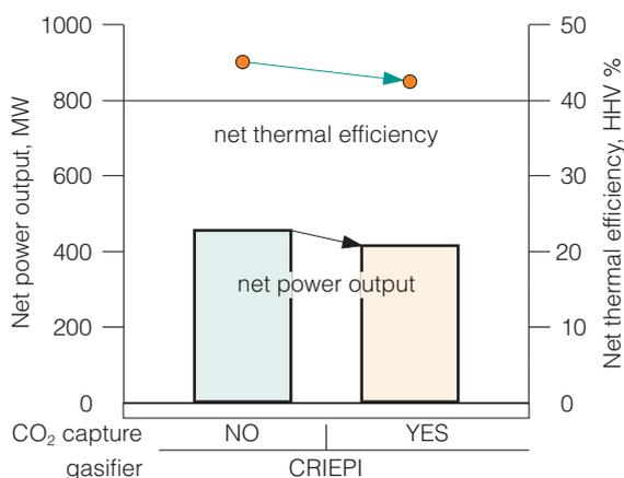
Figure 26 Comparison of thermal efficiency and net power output (Shirai and others, 2007)
