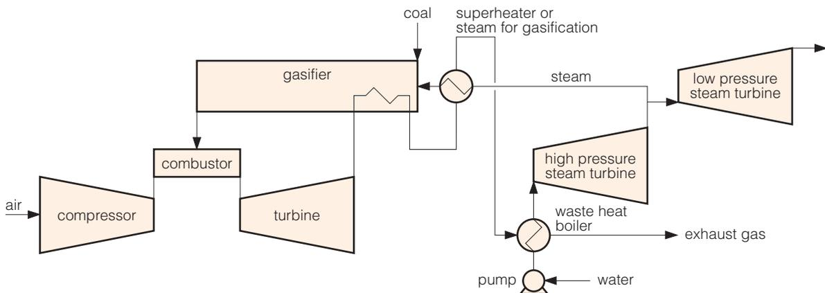
Figure 19 Basic structure of IGCC with chemical recuperation (Iki and others, 2009)
