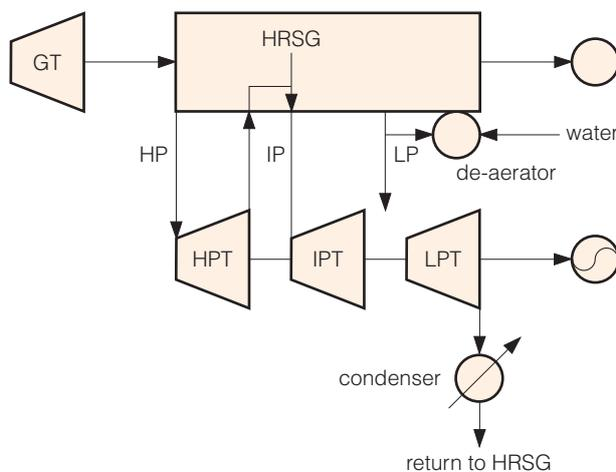
**Figure 7 Three-pressure reheat steam cycle** (Hodrien, 2008)
