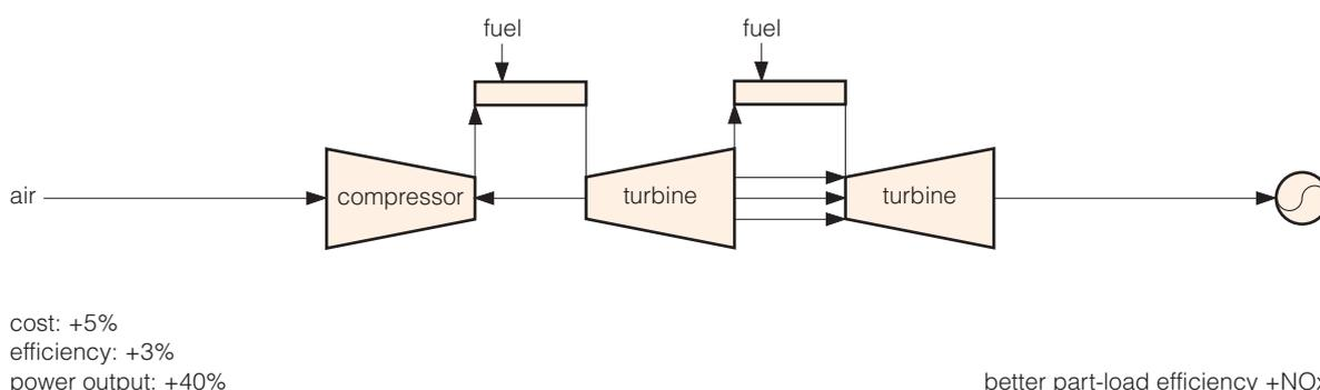
**Figure 9 Principles of gas turbine reheat combustion** (Güthe and others, 2008)
