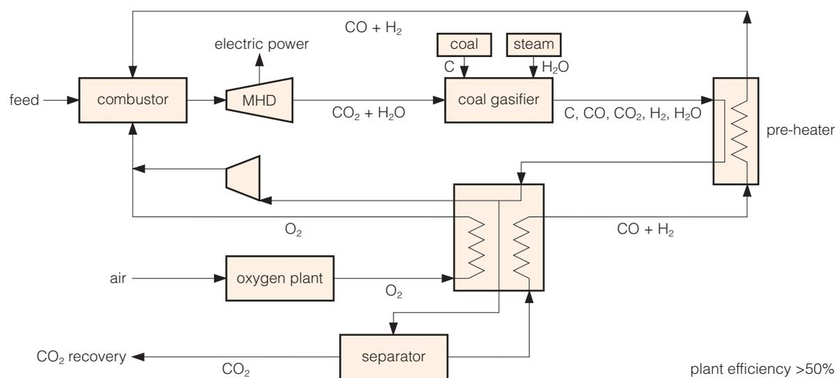
**Figure 41** CO<sub>2</sub> recovery type MHD generator plant (Harada, 2008)
