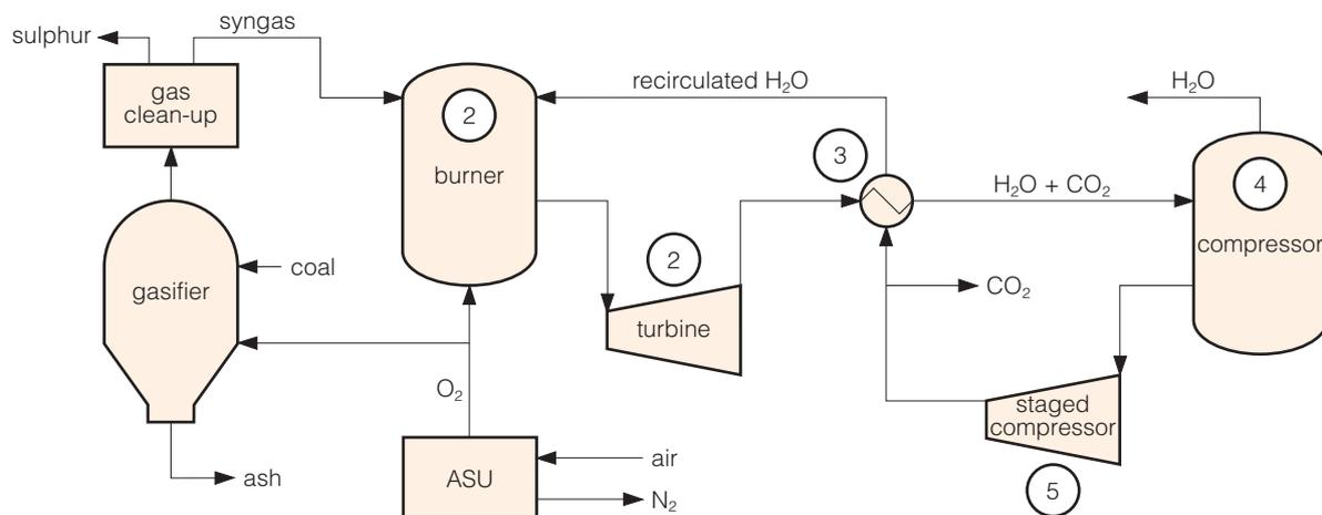
**Figure 5** Example of E-Matiant cycle variant (Houyou and others, 1997)
