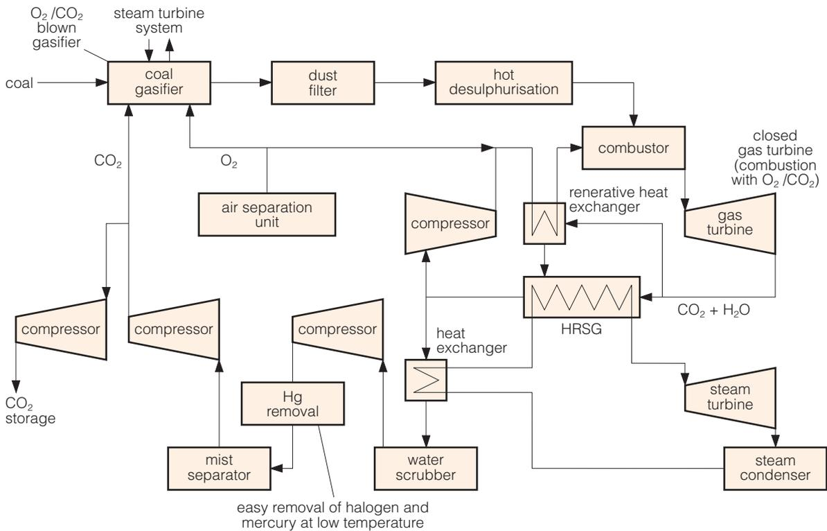
**Figure 25** Detailed schematic diagram of newly proposed 'Oxy-fuel IGCC' (Shirai, and others 2007)
