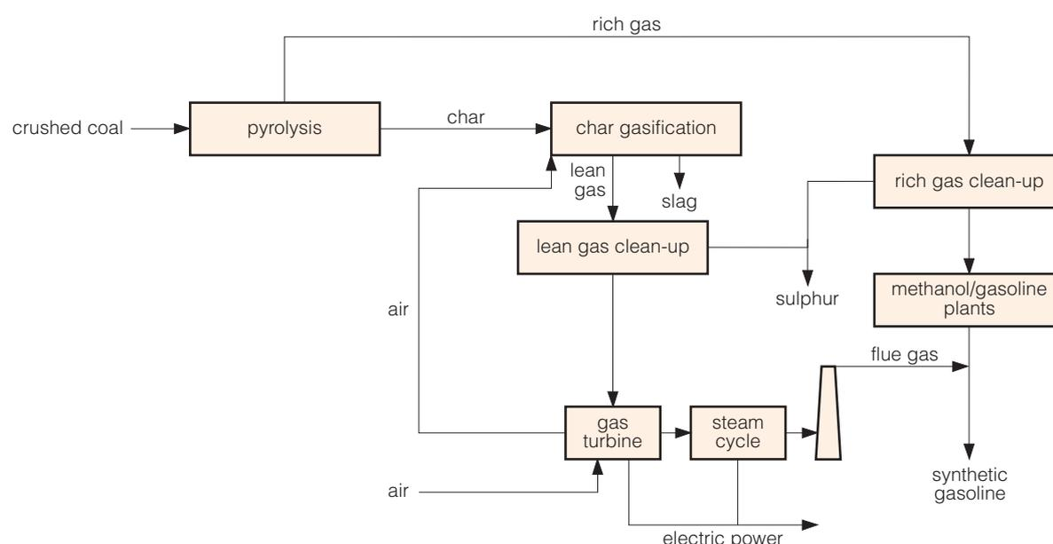
Figure 30 Schematic diagram of the Calderon Process (Calderon, 2007)
