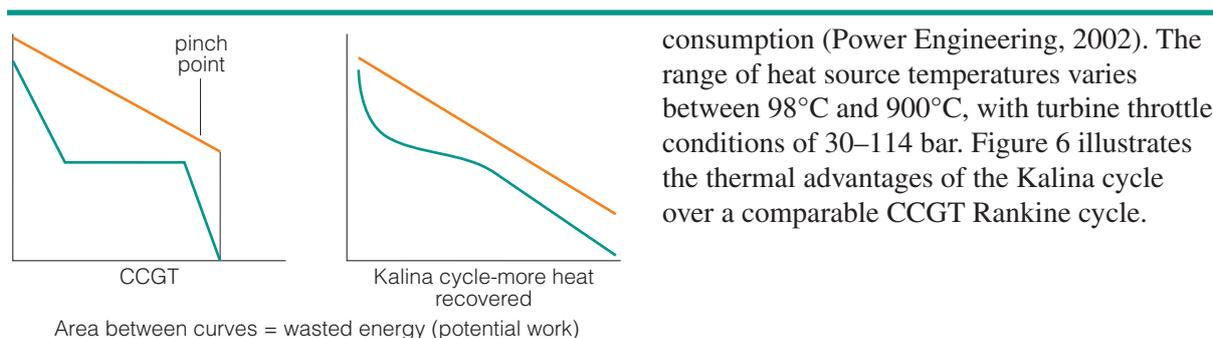
**Figure 6 Kalina versus CCGT Rankine cycle**
