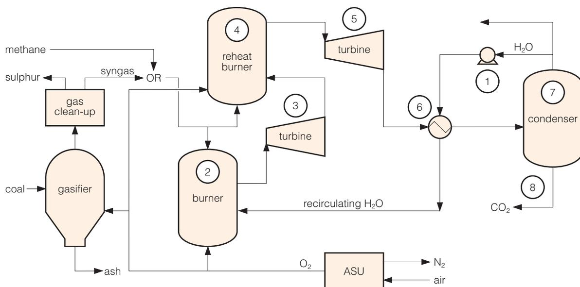
**Figure 3** Water cycle-based coal gasification process (Houyou and others, 1997)
