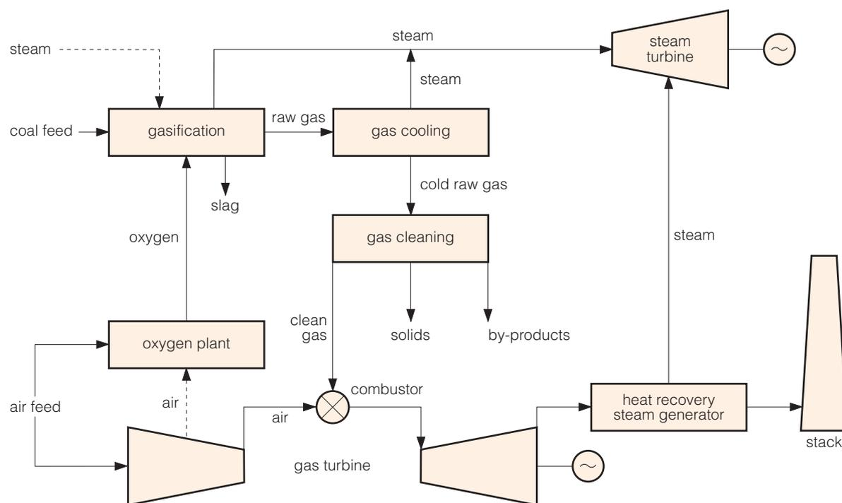
**Figure 1 Integrated gasification combined cycle without CO<sub>2</sub> capture – major component systems** (Henderson, 2008)
