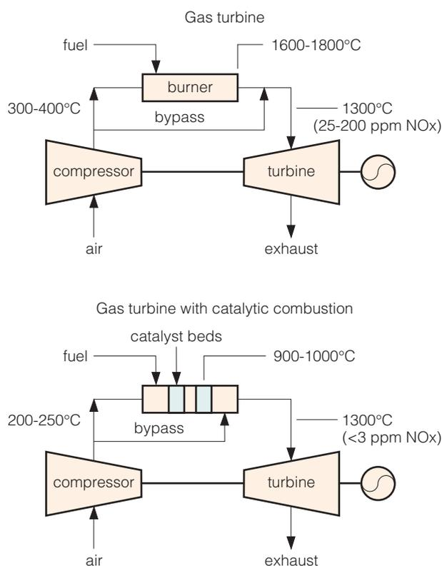
**Figure 8 Catalytic combustion** (NETL, 2006)
