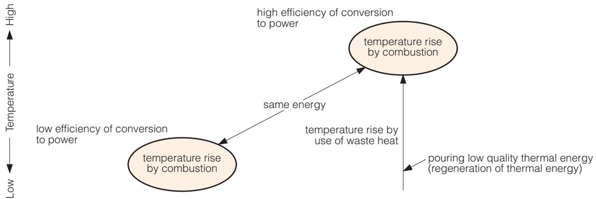
**Figure 16** Concept of recovery of low quality thermal energy (Iki and others, 2009)
