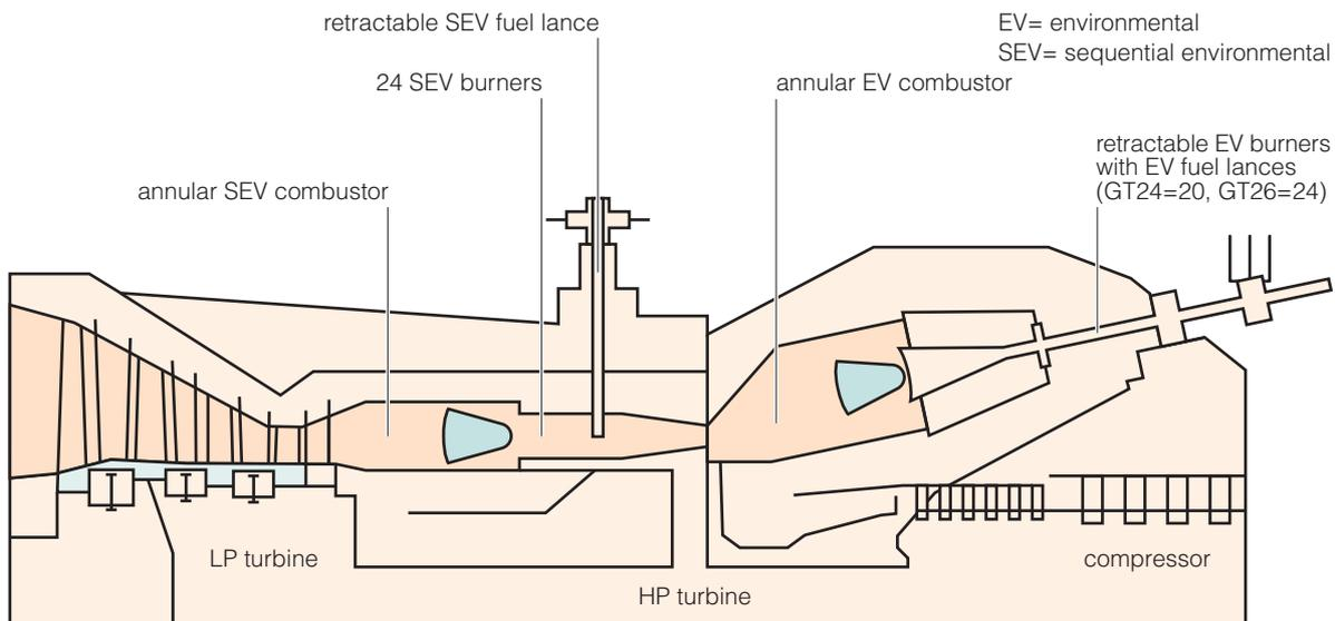
**Figure 10 Alstom GT26 reheat combustion gas turbine** (Henderson, 2007)
