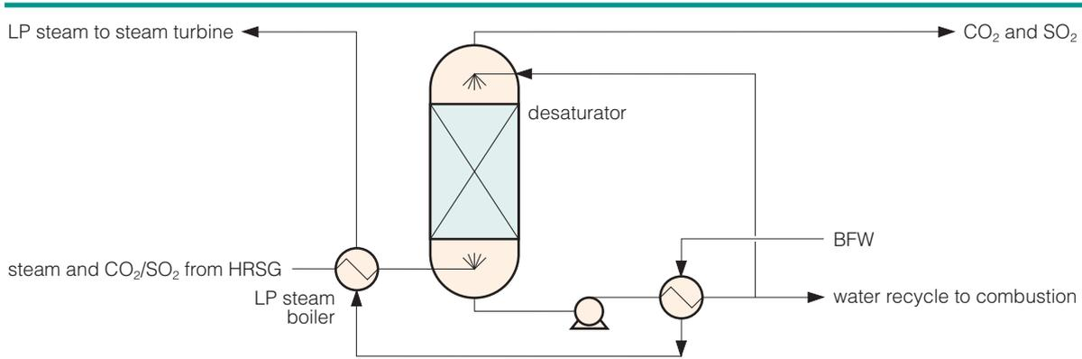
**Figure 34 Jacobs desaturator** (Griffiths, 2009)
