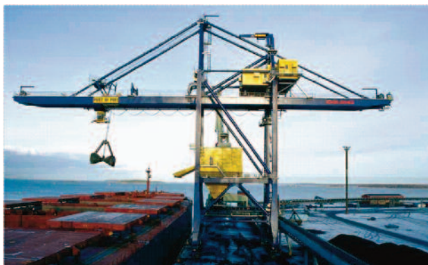
Figure 14 Bulk unloader using gantry mounted grab system (gantry type ) (Thyssenkrupp, 2012)
