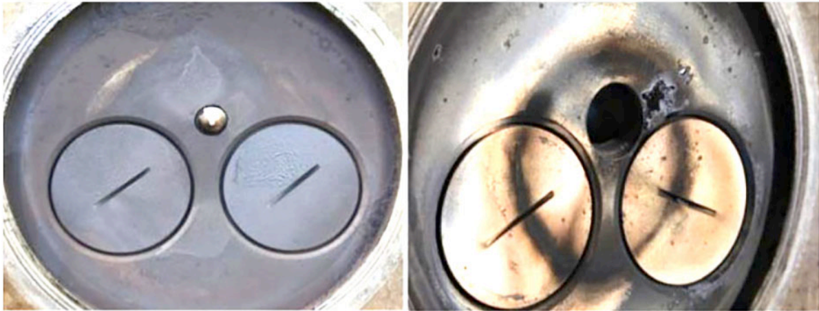
Figure 39 Cylinder head deposits from diesel (left) and UCC-MRC (right) (Wibberley, 2014c)
