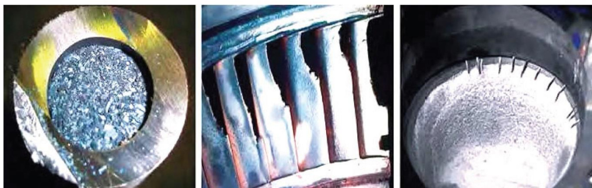
Figure 15 Oxide deposits on boiler tubes (left), solid particle erosion on turbine blades (centre) and bypass valve plug (right) (Feng, 2015)
