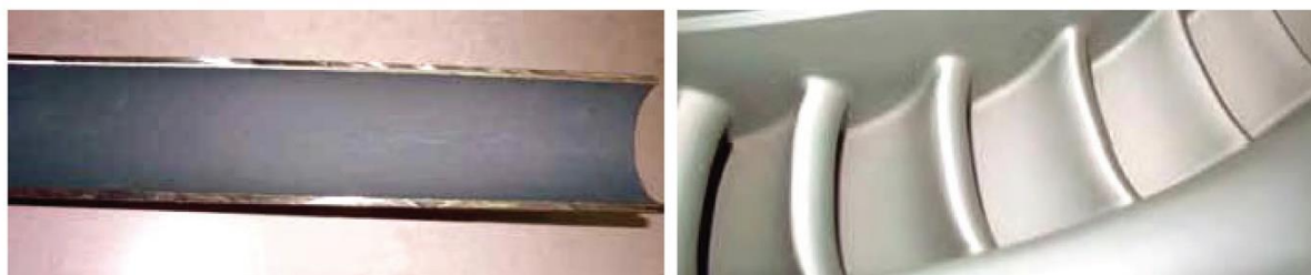
Figure 16 Pipe from the second reheater tube (left) first blading of an IP turbine (right) after 30 months of operation (Feng, 2015)
