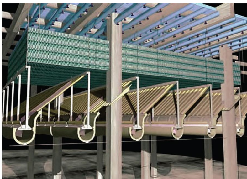
Figure 19 Internal structure of the high-yield wet cooling tower (Liu, 2015a)
