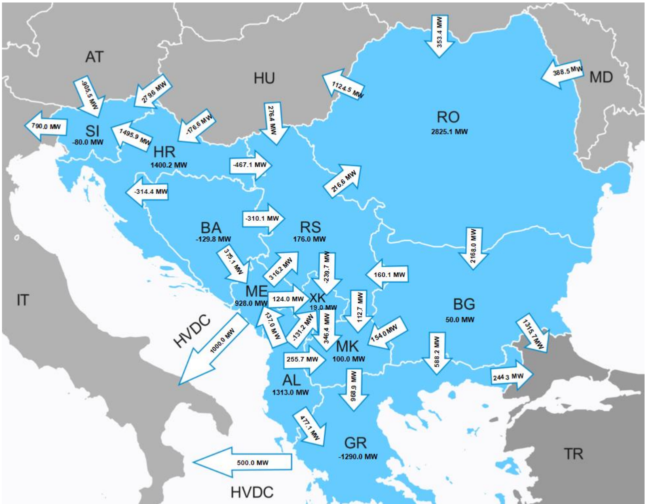
Figure 167: Cross-border exchanges (MW) and directions between the countries in scenario: high RES, low demand growth, referent CO 2 and maximum WPP and HPP
