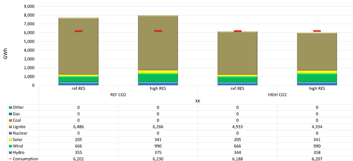
Figure 105: Generation mix in KOSTT market area in 2030 - ref. RES vs high RES, ref. CO 2 and high CO 2 emission tax
