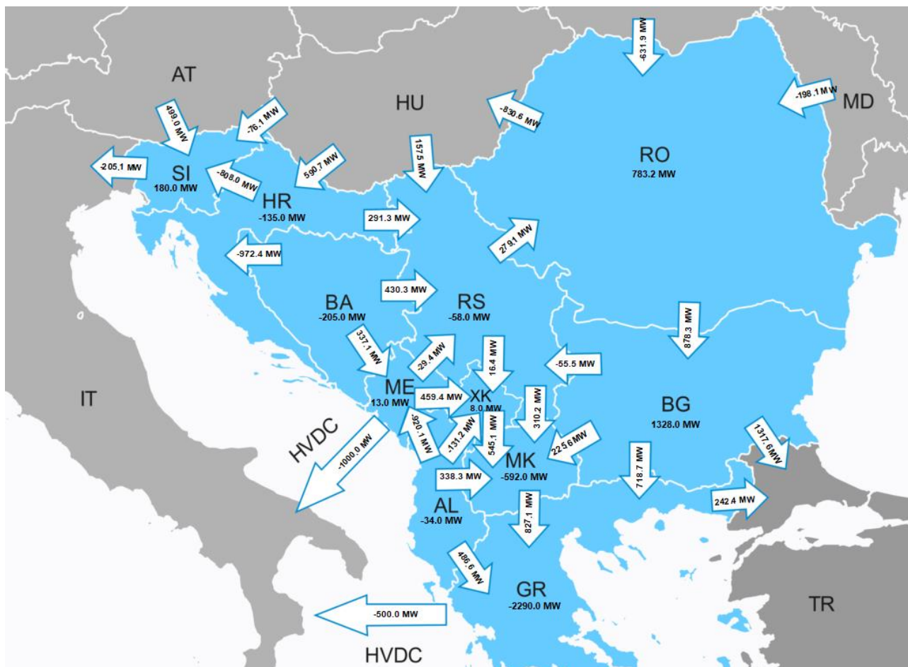
Figure 155: Cross-border exchanges (MW) and directions between the countries in scenario 2: high RES, low demand growth, referent CO 2 and minimum load
