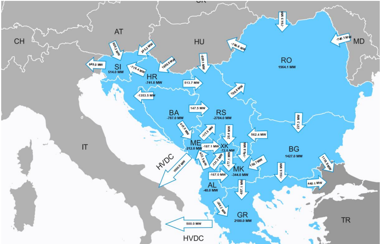
Figure 173: Cross-border exchanges (MW) and directions between the countries in scenario: high RES, low demand growth, referent CO 2 and maximum SPP
