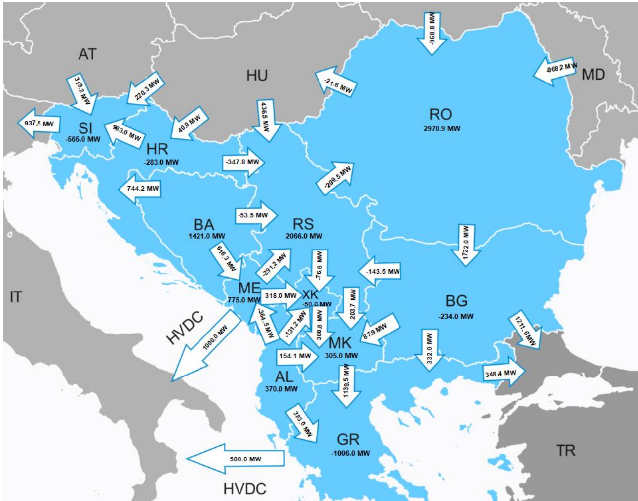
Figure 202: Cross-border exchanges (MW) and directions between the countries in gas integration scenario
