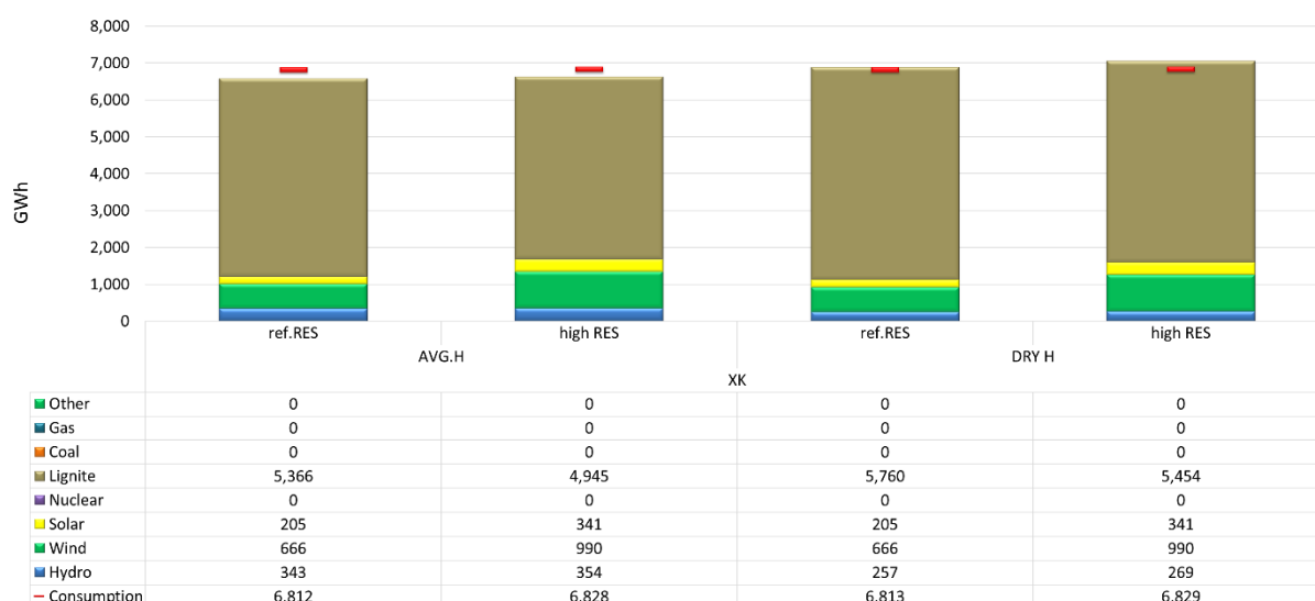
Figure 77: Generation mix in KOSTT market area in 2030 - ref. RES vs high RES, dry and average hydrology – Alternative CO 2 emission tax
