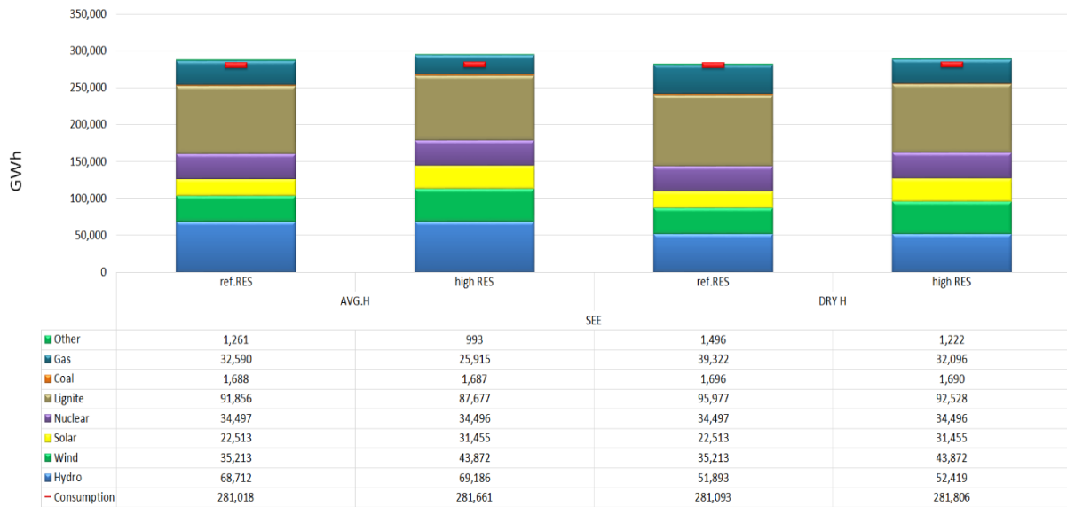
Figure 22: Generation mix in EMI region in 2030 - ref. RES vs high RES, dry and average hydrology
