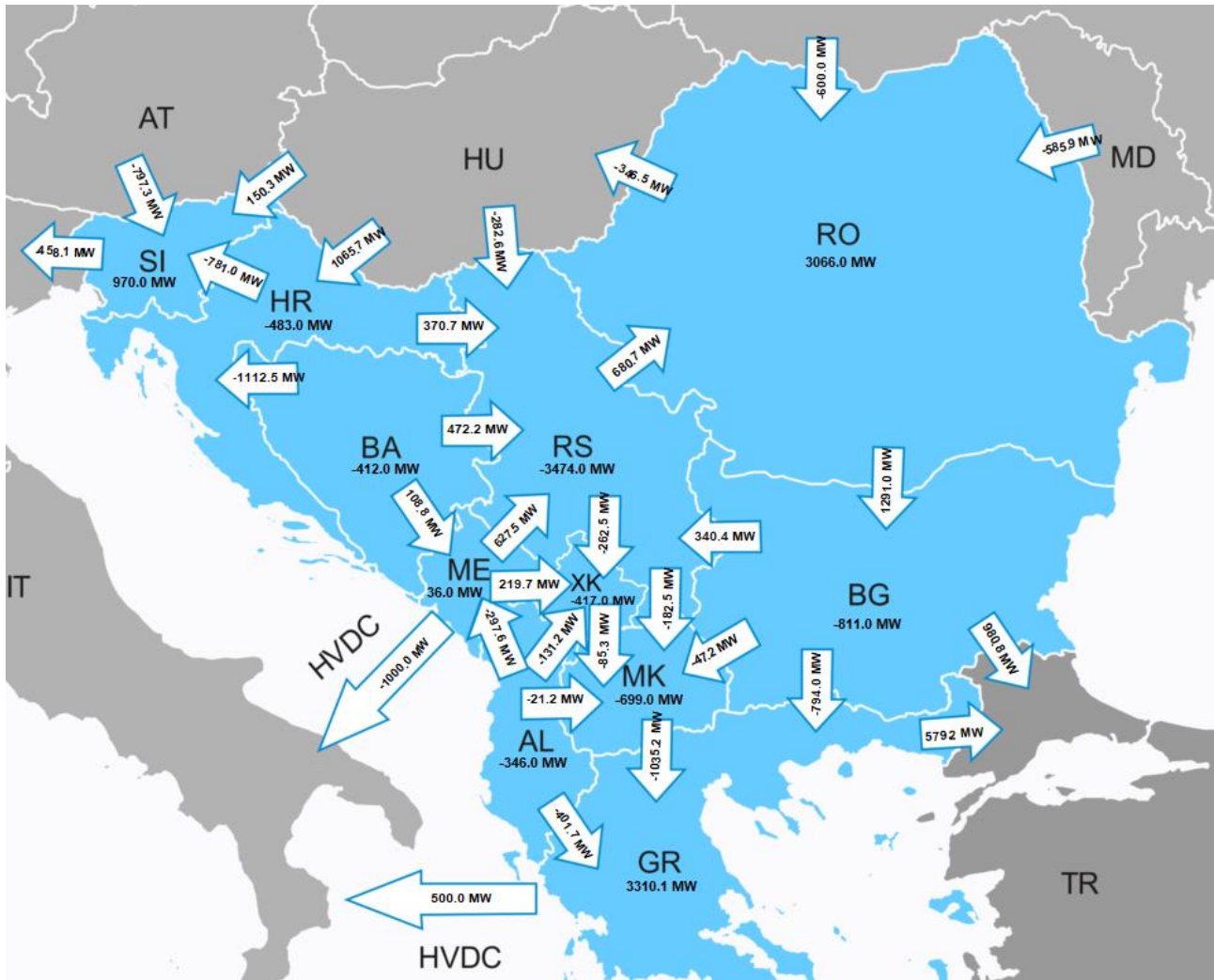
Figure: Cross-border exchanges (MW) and directions between the countries in scenario: high RES, low demand growth, alternative CO 2 and maximum RES
