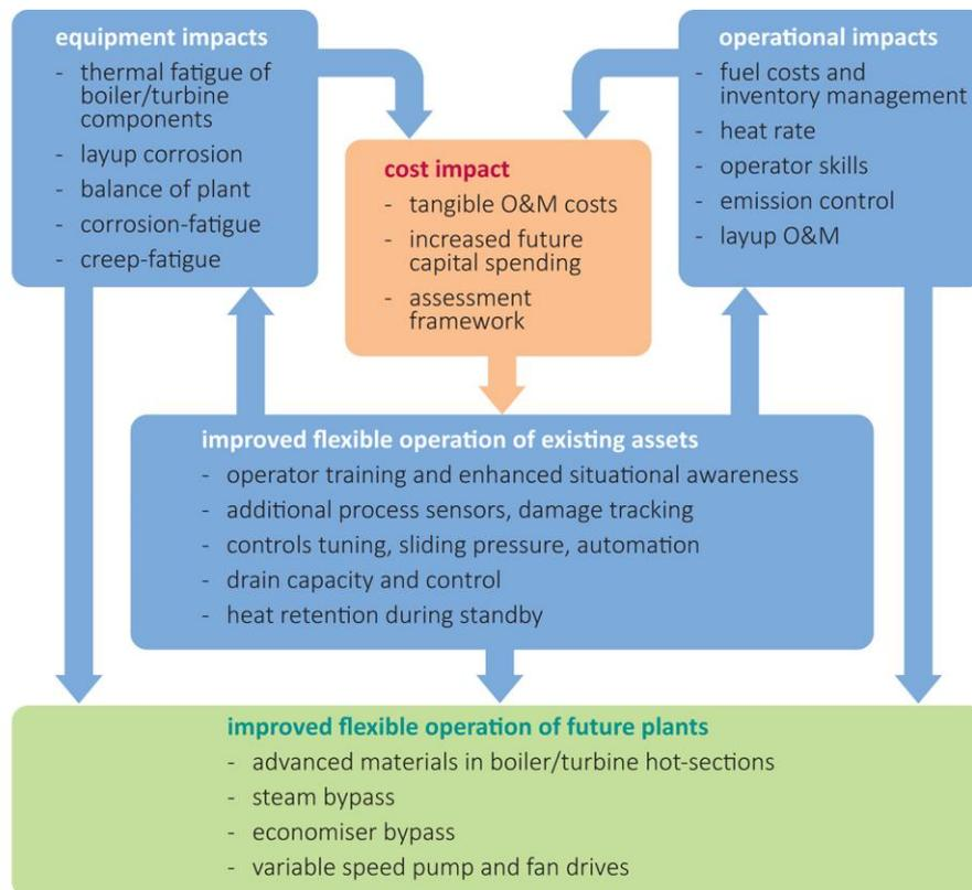
Figure 12 Impacts of cycling and key steps for improving flexible operations in coal-fired plants (EPRI, 2016)
