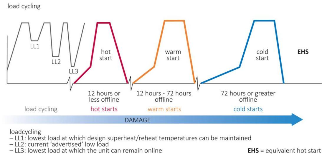
Figure 19 Power generating unit cycling definitions and effect (that is, relative damage) of load cycling (Lefton, 2012)
