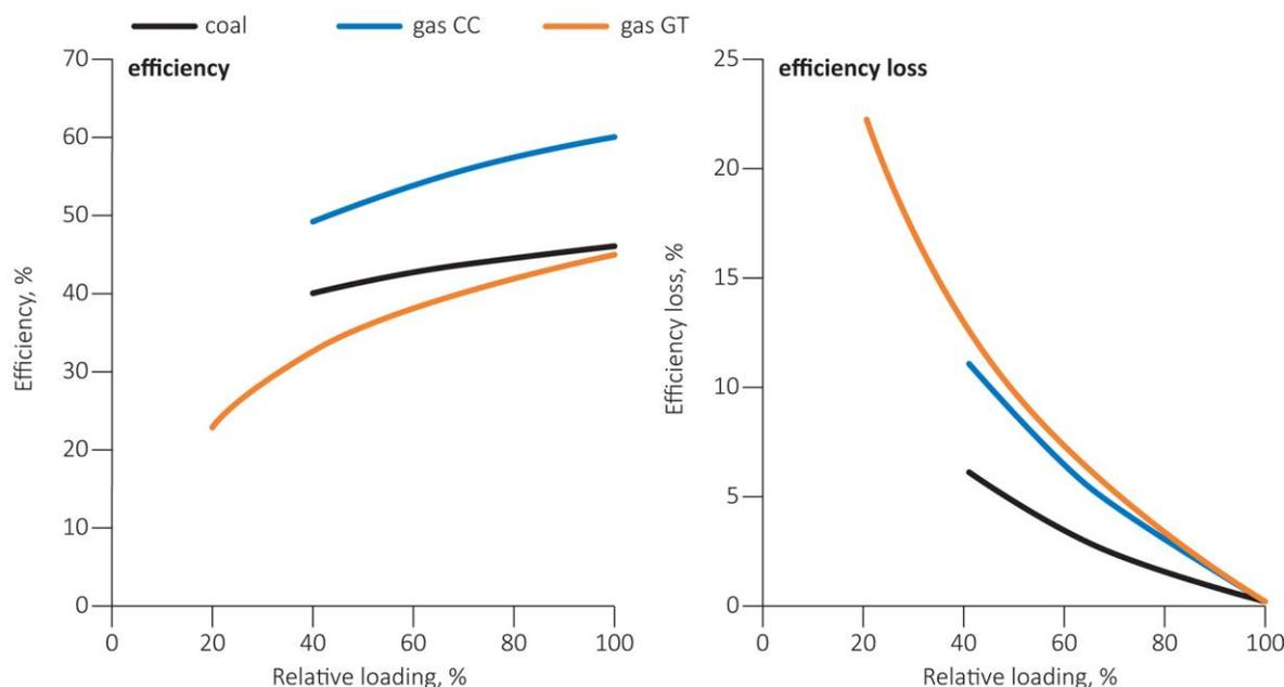
**Figure 13** The relationship between plant loading, efficiency and efficiency-loss) (Schröder and others, 2013)
