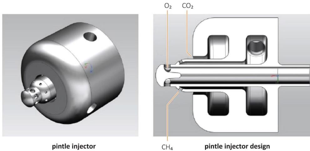
**Figure 19** Design concept for a pintle injector and a pintle injector design (Chowdhury and others, 2016)
