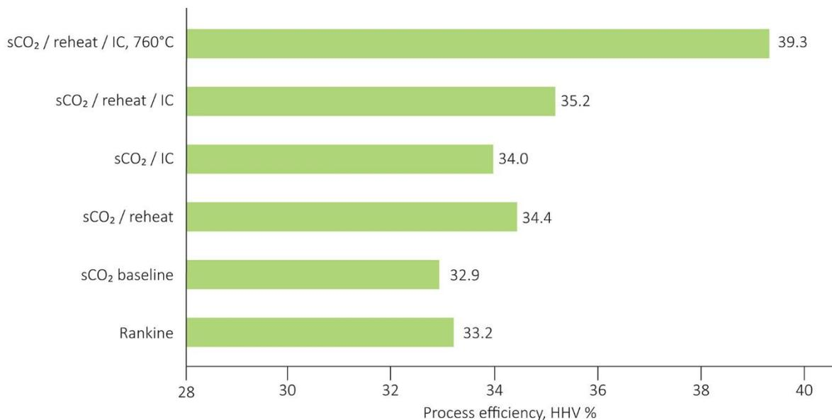
**Figure 23 Efficiency comparison of coal oxyfired ACFB power plants with Rankine cycle and with closed-loop sCO<sub>2</sub> Brayton cycles** (Shelton and others, 2016)
