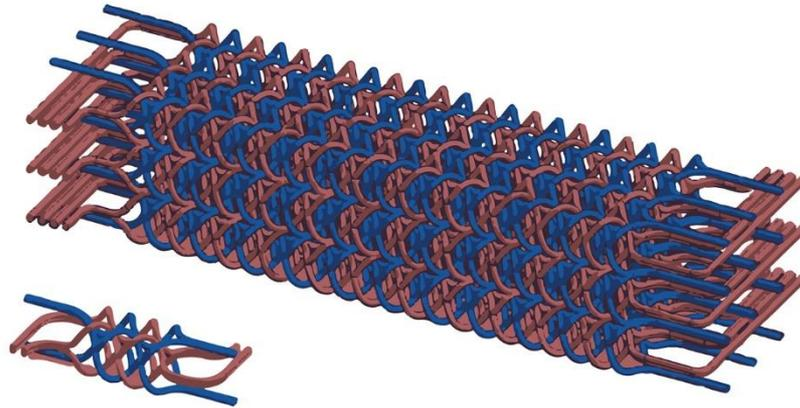
**Figure 14** A counter-rotating double-helical geometry proposed for use in a CMHE between two similar fluids: red channels for hot flow and blue for cold flow (Carlson and others, 2014a)
