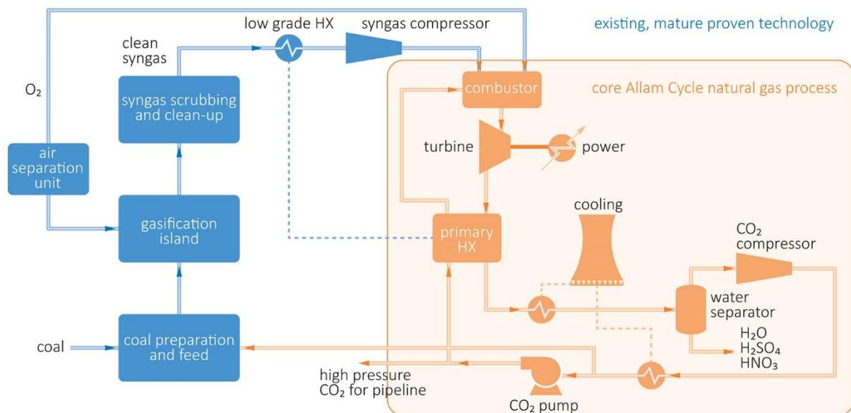
Figure 30 A simplified block flow diagram of the Allam Cycle couple with a coal gasification system (Lu, 2016)
