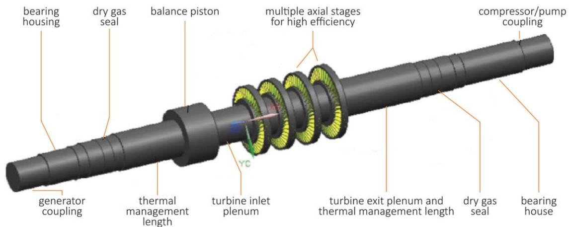
Figure 7 The 10 MWe high-pressure, high-temperature turbine rotor design developed for CSP (Kalra and others, 2014)
