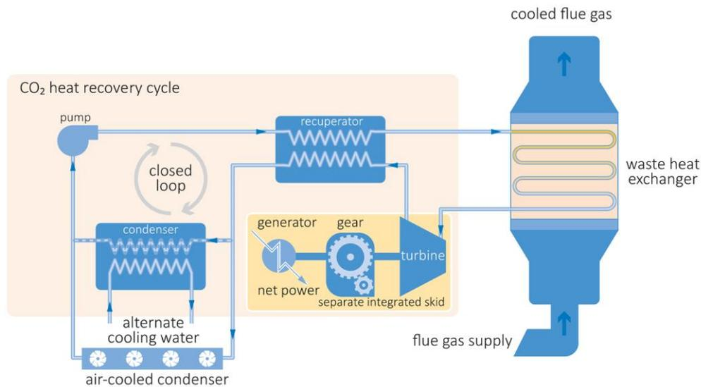
Figure 34 The EPS100 sCO<sub>2</sub> heat recovery cycle (<http://www.echogen.com/>)
