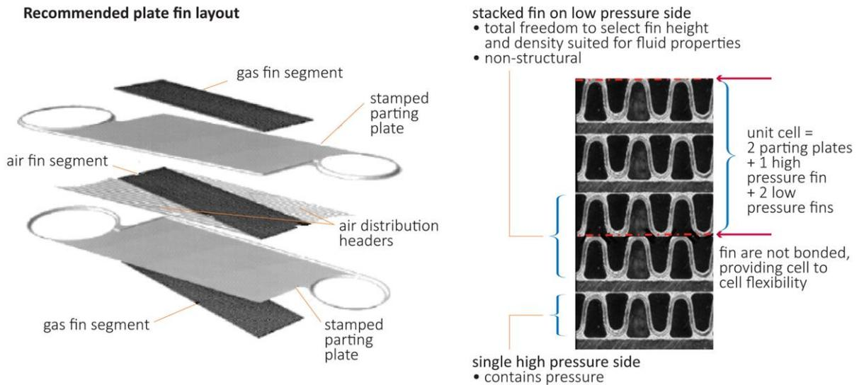
**Figure 11 Recommended PFHE design for recuperator services in sCO<sub>2</sub> cycles** (Kesseli and others, 2007)
