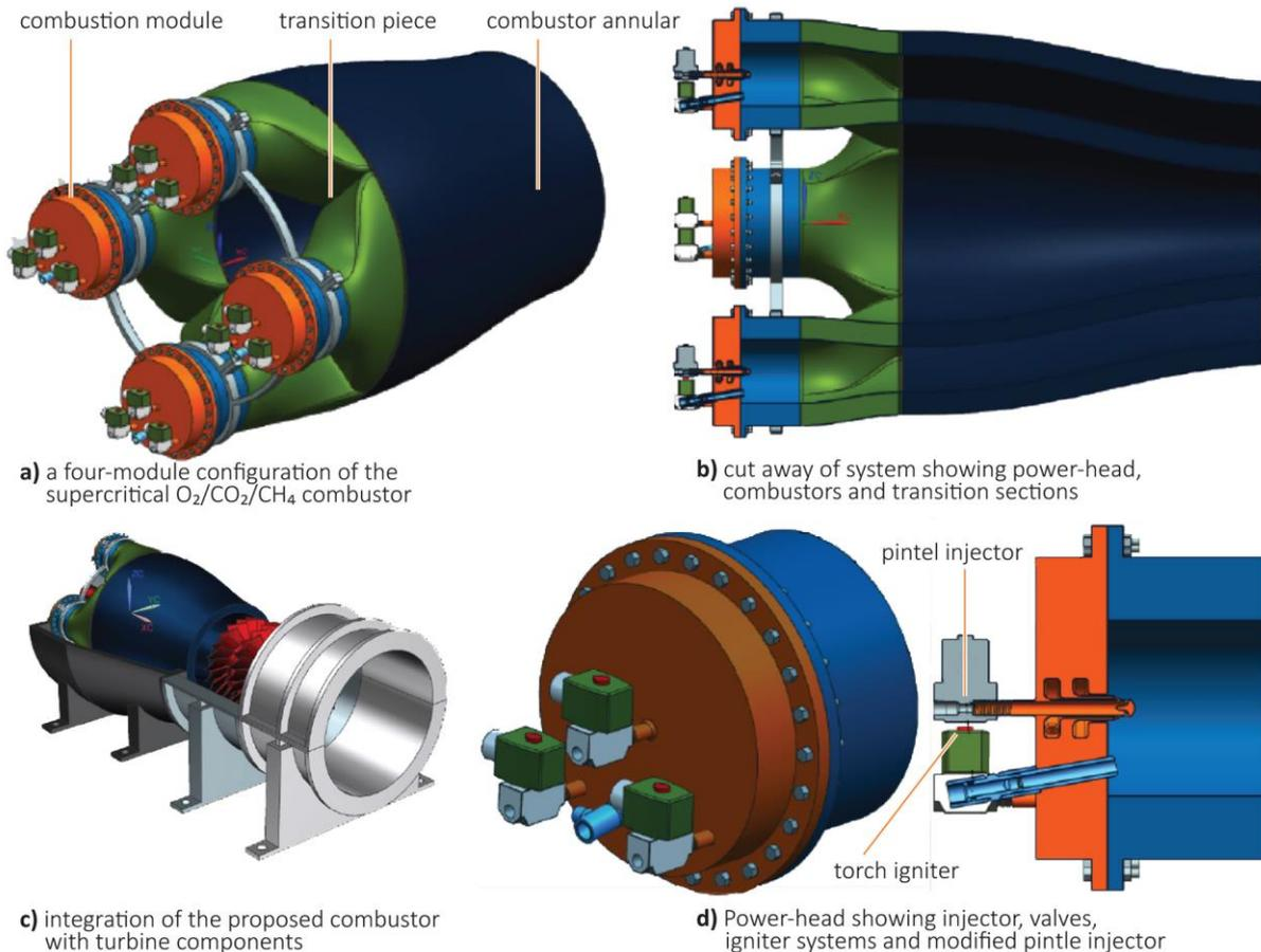
**Figure 18 Oxyfuel combustor design developed by the University of Texas** (modified from Chowdhury and others, 2015)
