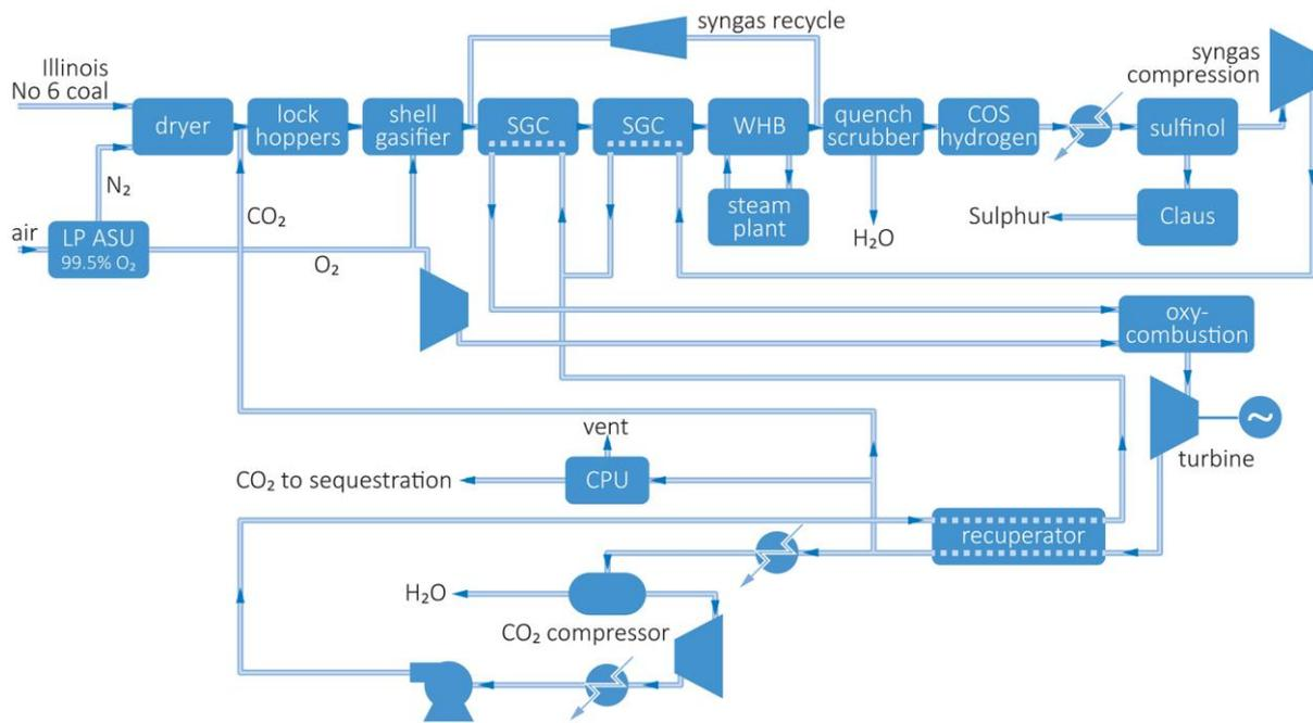
Figure 29 Block flow sheet of the syngas-fired, semi-closed oxy-combustion sCO<sub>2</sub> power plant (Weiland and others, 2016)
