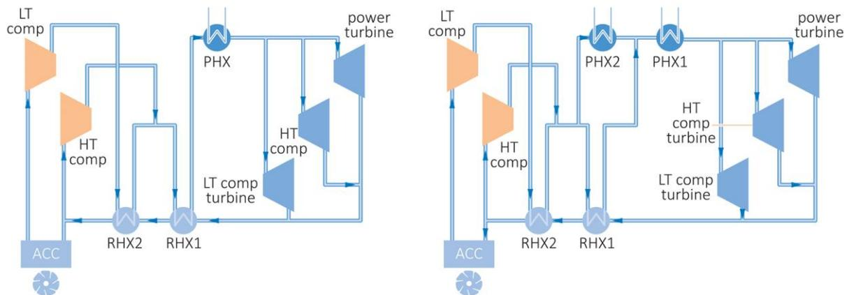
**Figure 22** The layout of baseline RC cycle (left) and RC-LG cycle (Miller and others, 2017)
