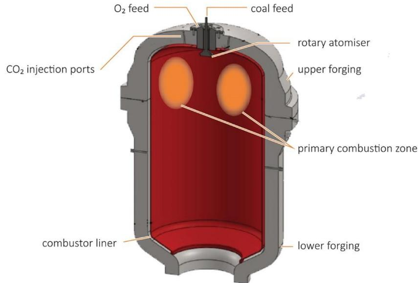
**Figure 20** The swirl type supercritical oxy-combustor for solid fuel (McClung and others, 2014)
