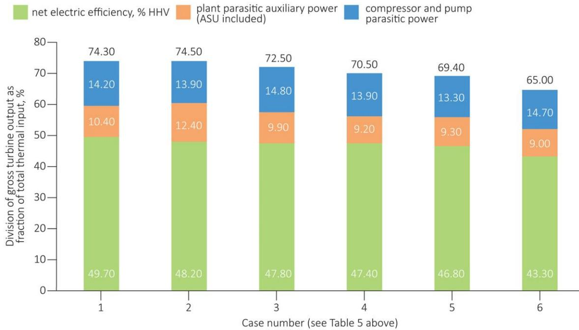
Figure 31 Comparison of optimised coal Allam Cycle configurations (Lu and others, 2016)
