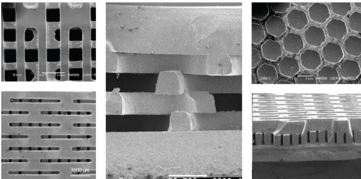
**Figure 16** Examples of features available in microchannel designs (Lewinsohn and others, nd)
