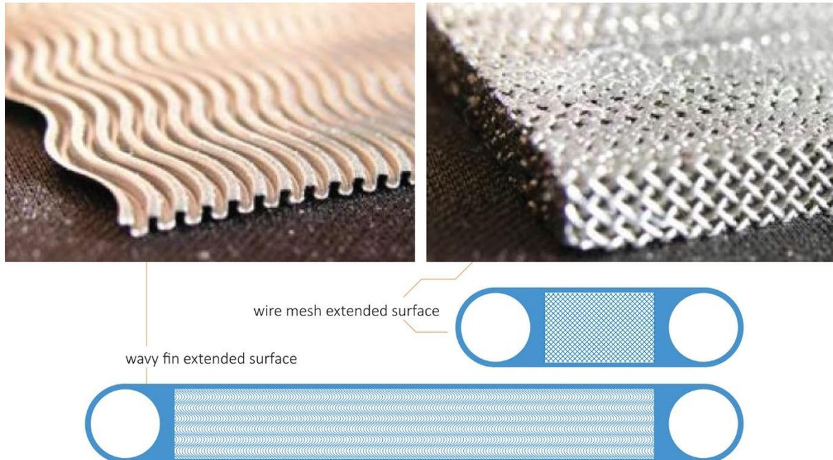
**Figure 13** Comparison of a wire-mesh heat exchanger unit-cell and a wavy-fin unit-cell with same capacity (Musgrove and others, 2014; Fourspring and others, 2014)
