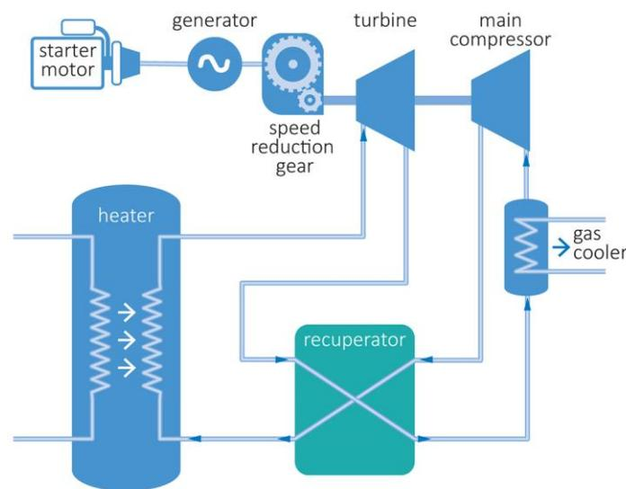
Figure 2 An indirectly-fired, recuperated, closed Brayton cycle (US DOE, 2015)
