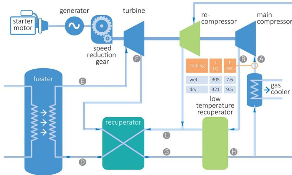
**Figure 3** An indirectly-fired, recuperated, recompression, closed Brayton cycle (US DOE, 2015)
