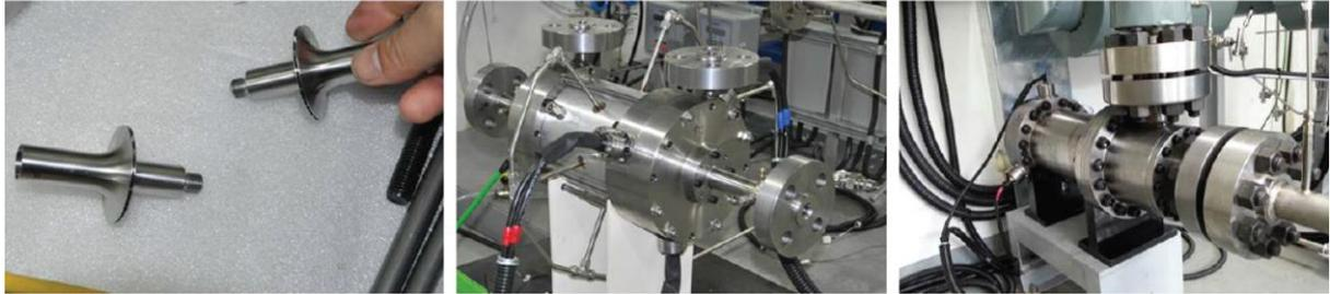
**Figure 6 Laboratory-scale sCO<sub>2</sub> turbomachinery and subcomponents**
