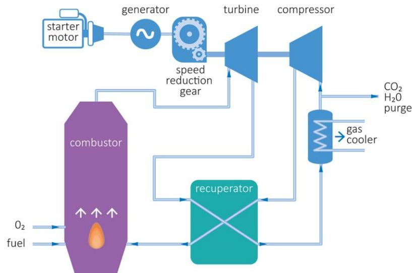
Figure 4 A simplified directly-fired, semi-closed, oxyfuel Brayton cycle (US DOE, 2015)
