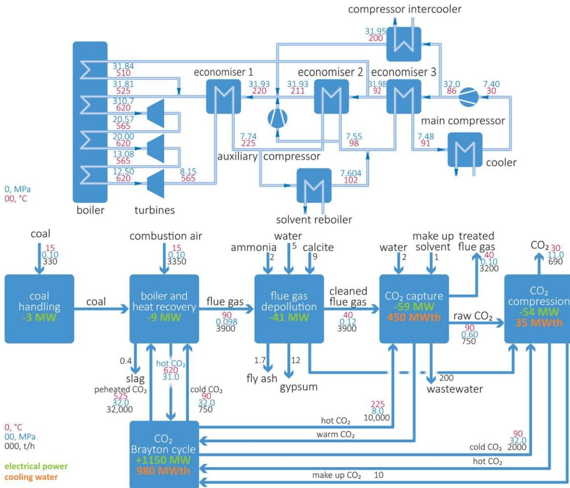
Figure 26 sCO<sub>2</sub> power cycle adapted for coal-fired boiler with carbon capture (top) and a simplified block flow diagram of the power plant built around a sCO<sub>2</sub> Brayton cycle (bottom) (Le Moulllec, 2013)
