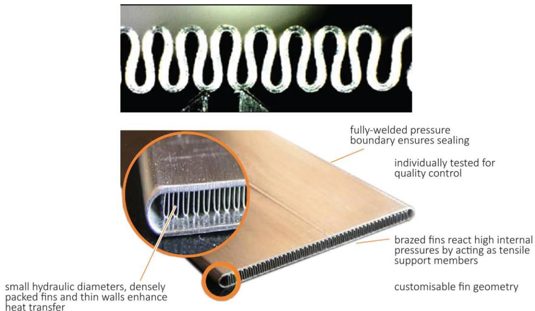
**Figure 12 The geometry of densely-packed folded fin (top) and the basic sCO<sub>2</sub> solar absorber panel design (bottom)** (Sullivan and others, 2016)
