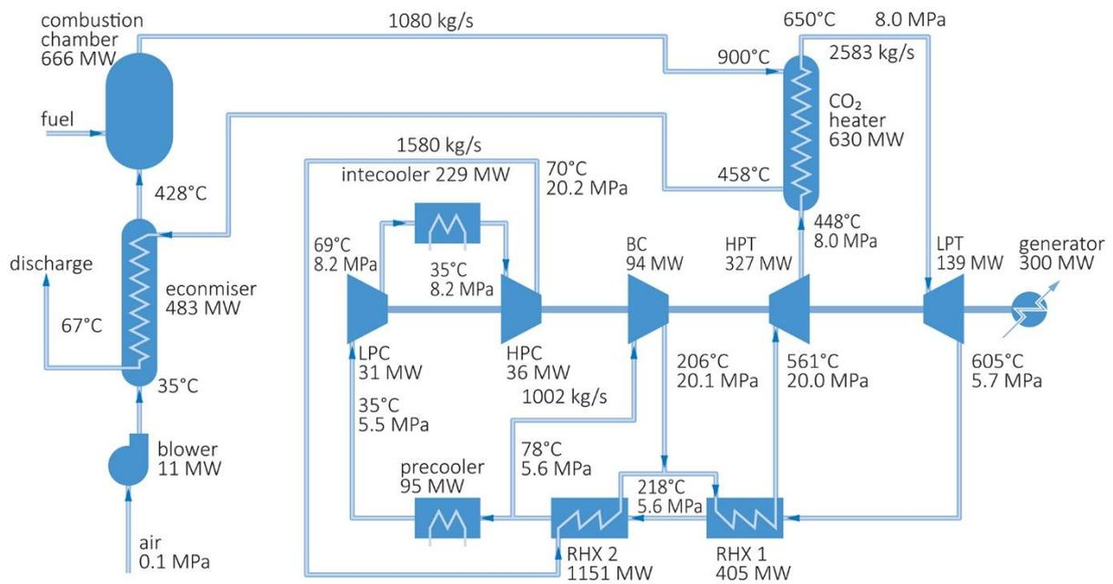
Figure 24 The layout of the 300 MWe fossil-fired sCO<sub>2</sub> cycle power plant (Muto and others, 2010)
