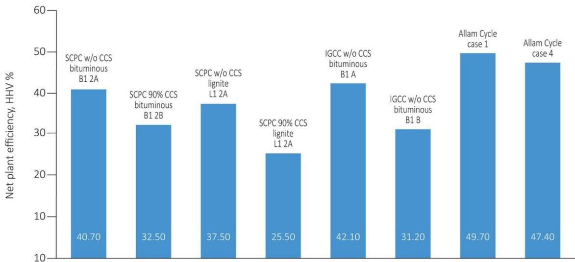
Figure 32 Comparison of coal-based Allam Cycles with NETL baseline plants
