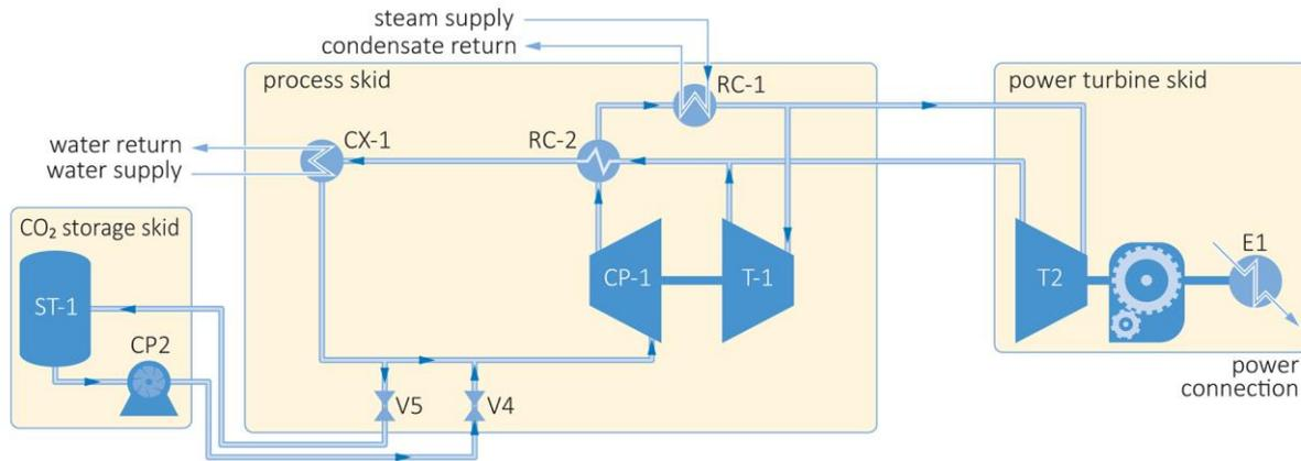
Figure 35 Process flow diagram of the EPS100 test facility (Held, 2014)
