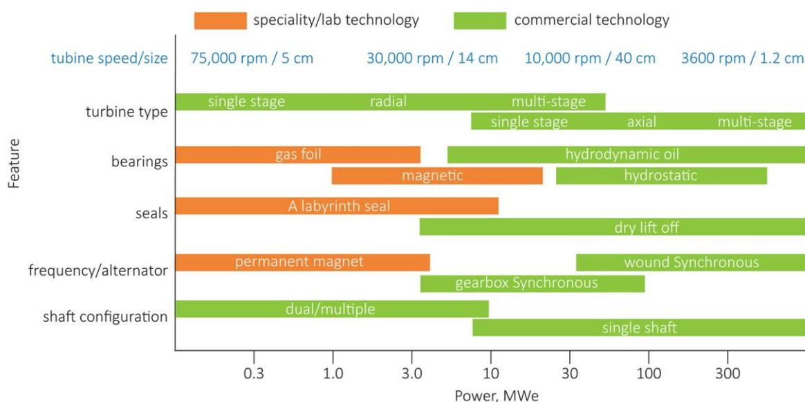
**Figure 5 Ranges of application for key Brayton cycle turbomachinery components and features**
