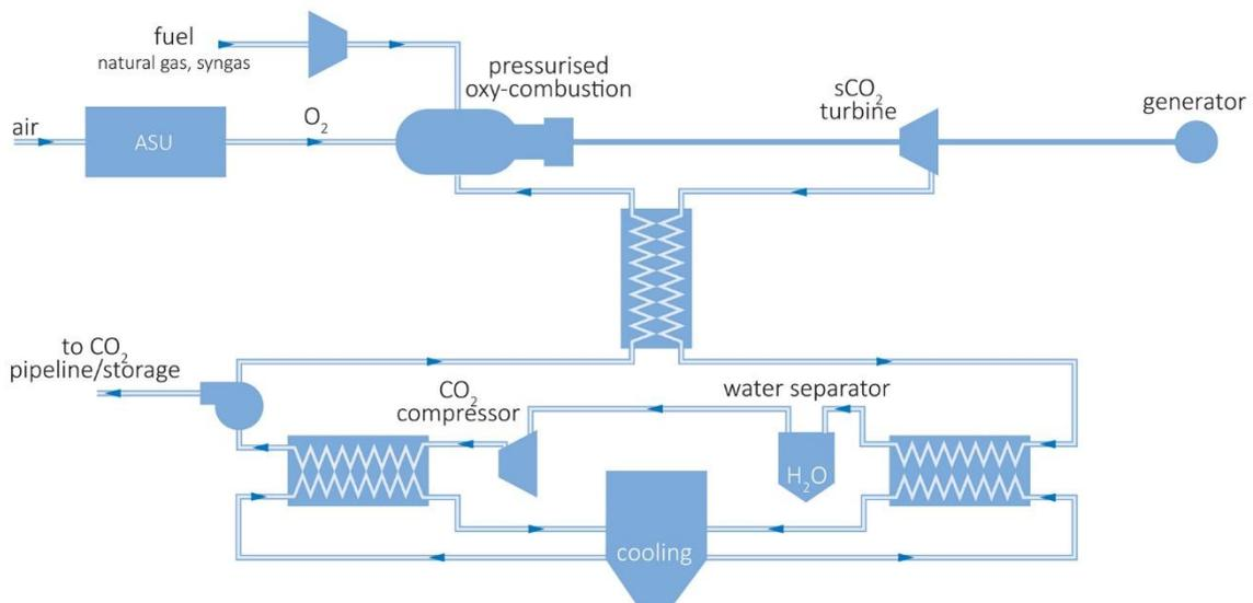
Figure 28 A potential configuration of oxygen-fuelled directly-heated sCO<sub>2</sub> cycle (NETL, 2017)
