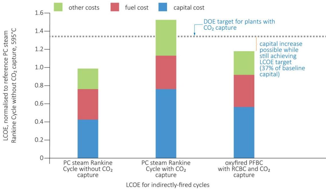
Figure 27 Comparison of LCOE of PCFB closed sCO<sub>2</sub> power cycle plant with NETL baseline plants (Eastland and others, 2014)
