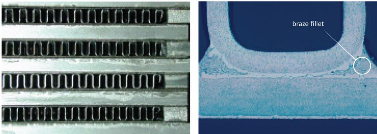
**Figure 10** Components of brazed plate fin-heat exchanger (Modified from Kesseli and others, 2007)
