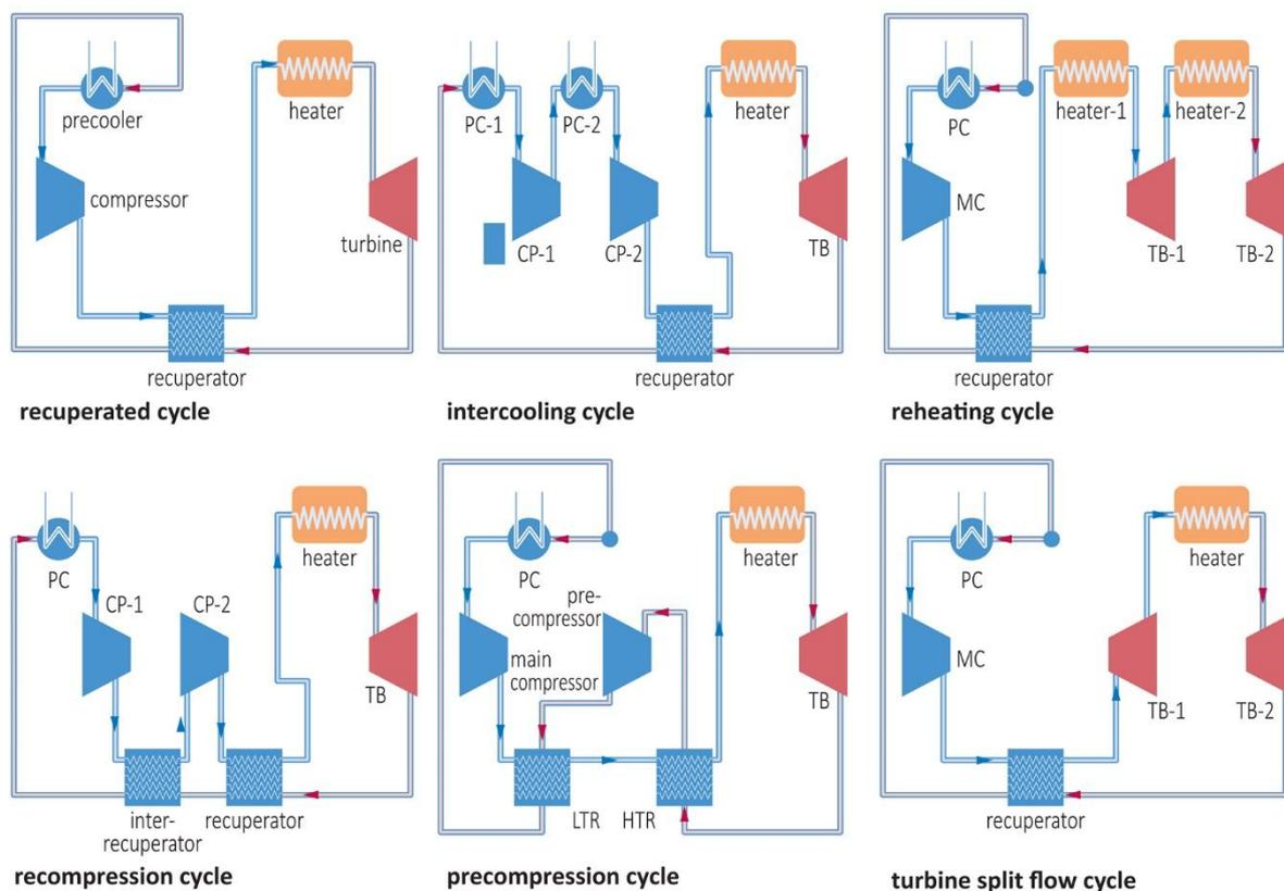
Figure 21 Examples of the proposed sCO<sub>2</sub> Brayton cycles (Ahn and others, 2015)
