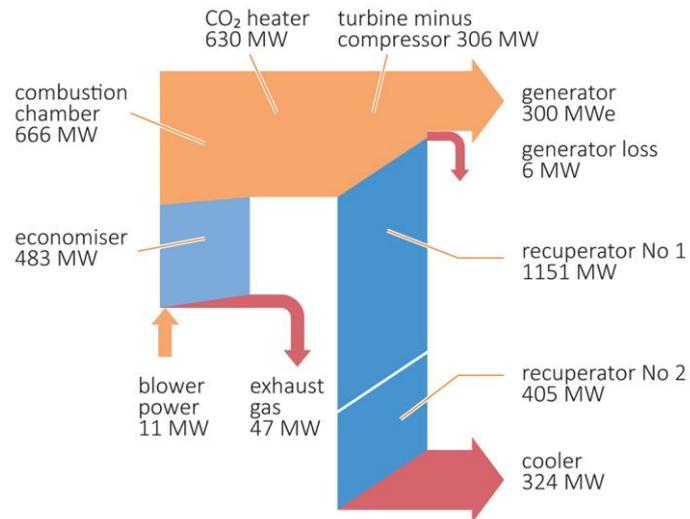
Figure 25 Energy flow diagram of the system (Muto and others, 2010)
