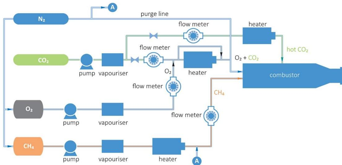
**Figure 17** Toshiba's 30 MPa oxy-combustion test system (Iwai and others, 2015)
