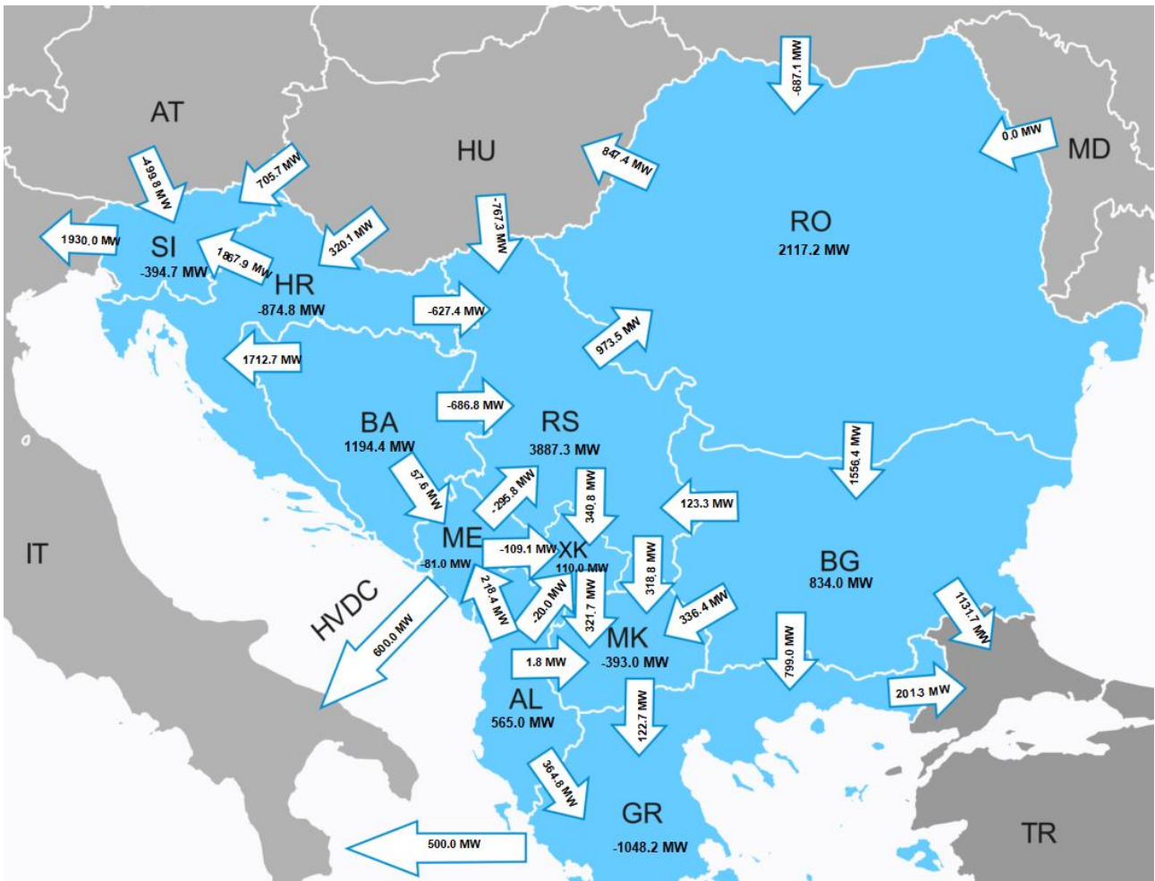
Figure 8.17: Cross-border exchanges (MW) and directions between the countries for Highest export regime 2025 (high RES, referent CO2)
