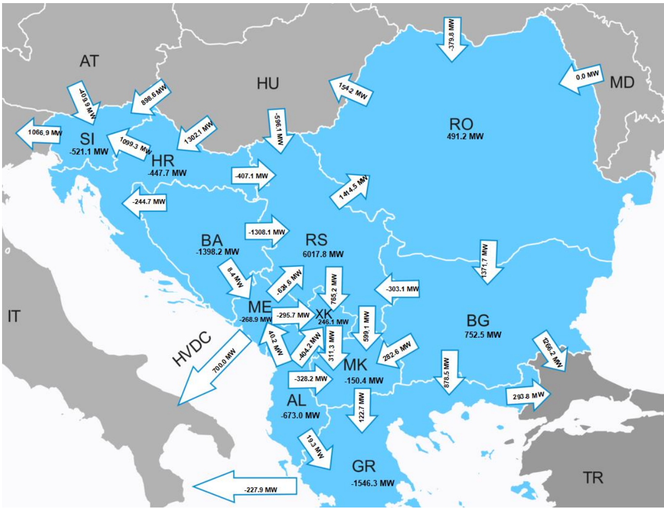
Figure 8.40: Cross-border exchanges (MW) and directions between the countries for Highest wind+solar generation regime 2030 (high RES, referent CO 2 )
