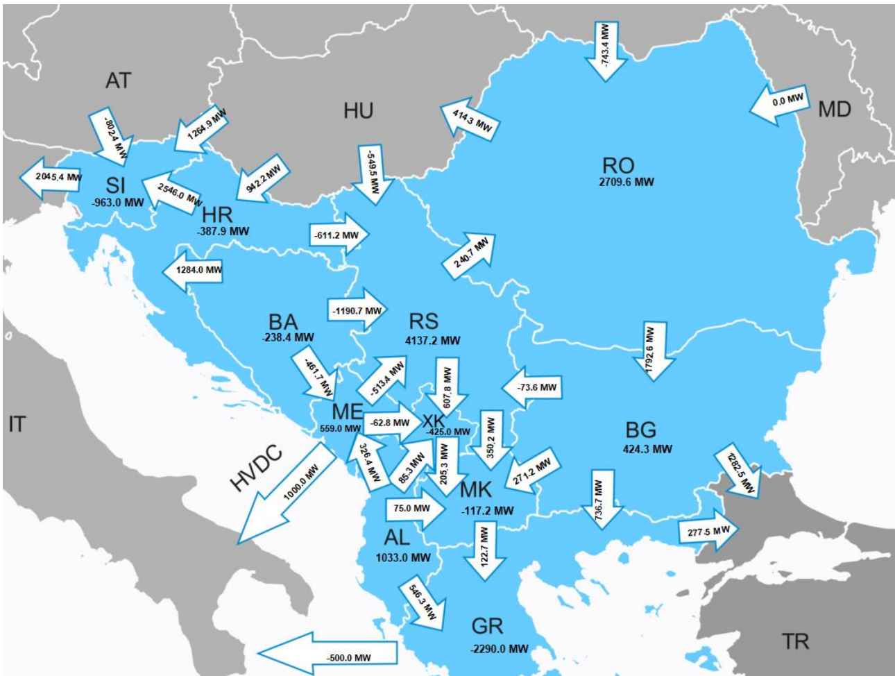
Figure 8.29: Cross-border exchanges (MW) and directions between the countries for Summer regime with the highest generation 2030 (referent RES, referent CO 2 )
