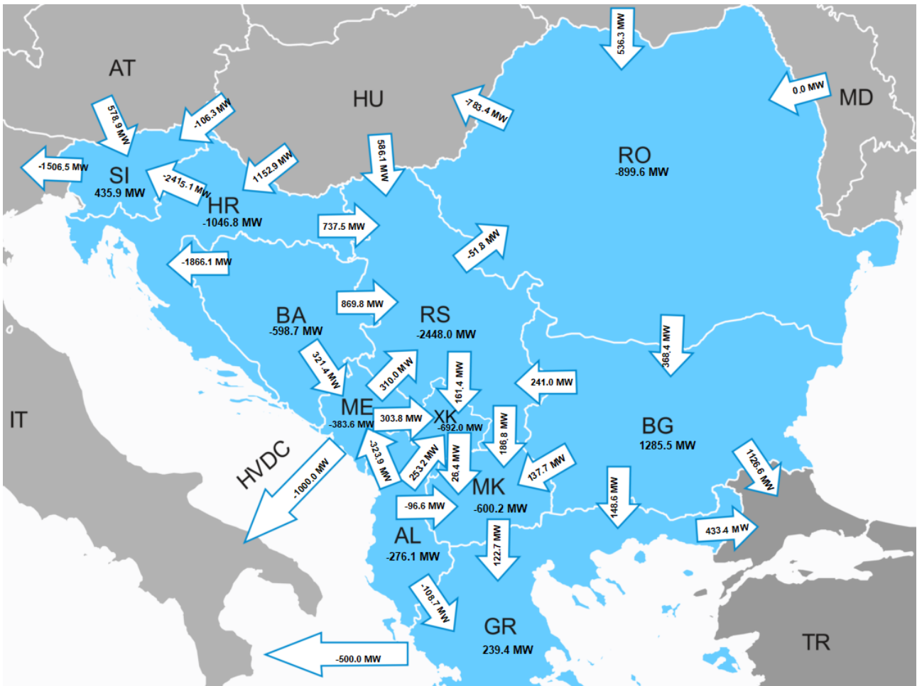
Figure 8.31: Cross-border exchanges (MW) and directions between the countries for Highest import regime 2030 (referent RES, referent CO2)
