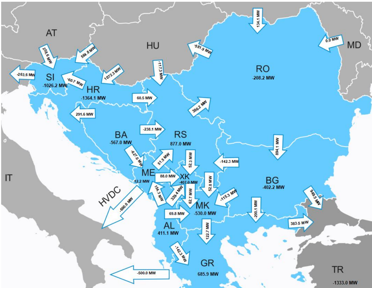
Figure 8.19: Cross-border exchanges (MW) and directions between the countries for Summer regime with the highest generation 2025 (high RES, high CO2 )
