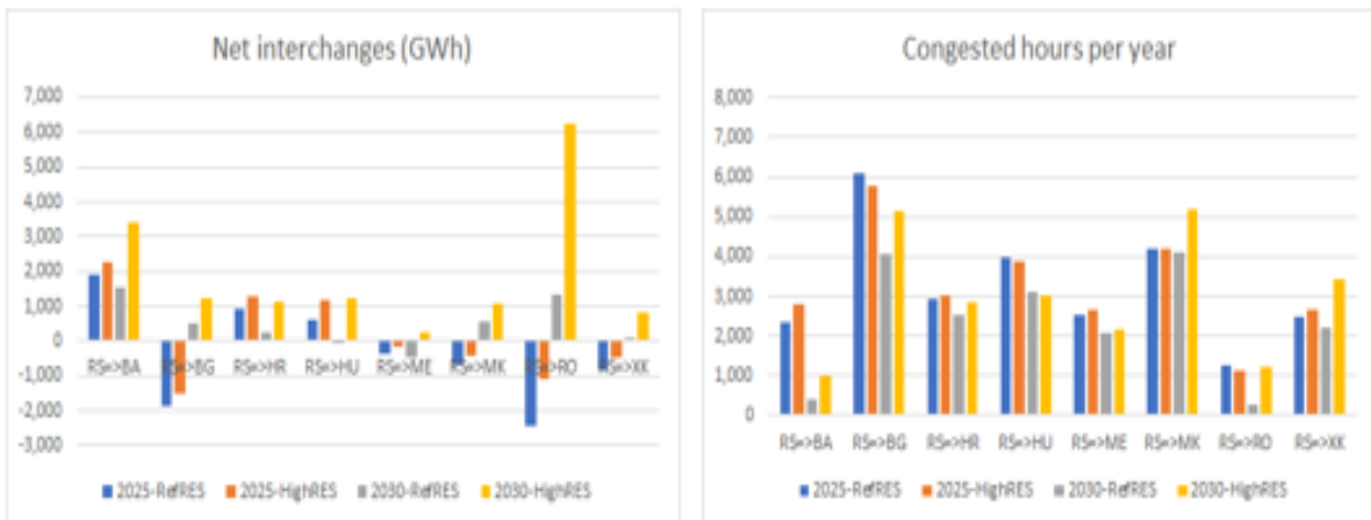
Figure 3.20: Annual net interchanges and congestions in the EMS market area – high CO2 scenario
