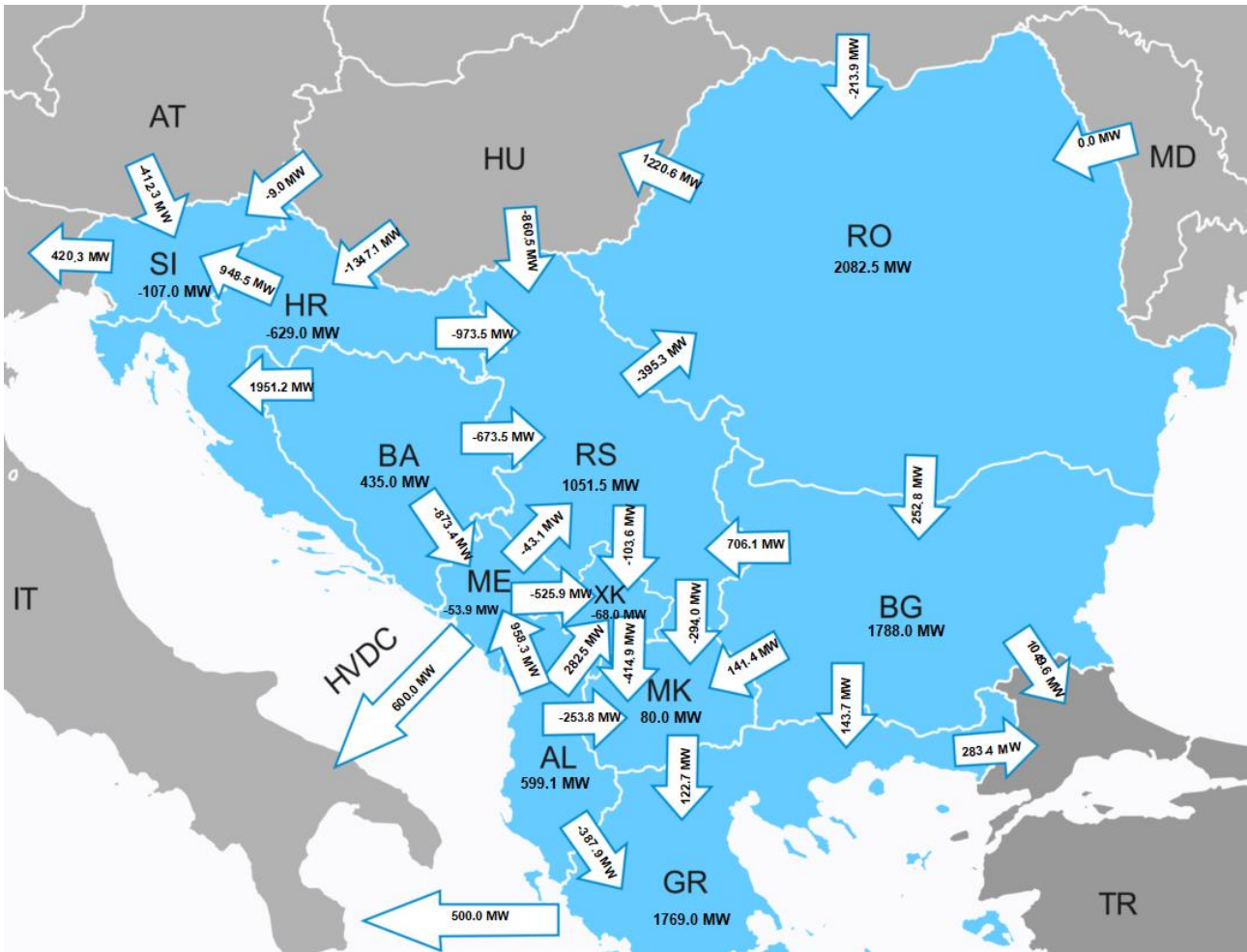
Figure 8.13: Cross-border exchanges (MW) and directions between the countries for Winter Peak regime 2025 (high RES, referent CO2)
