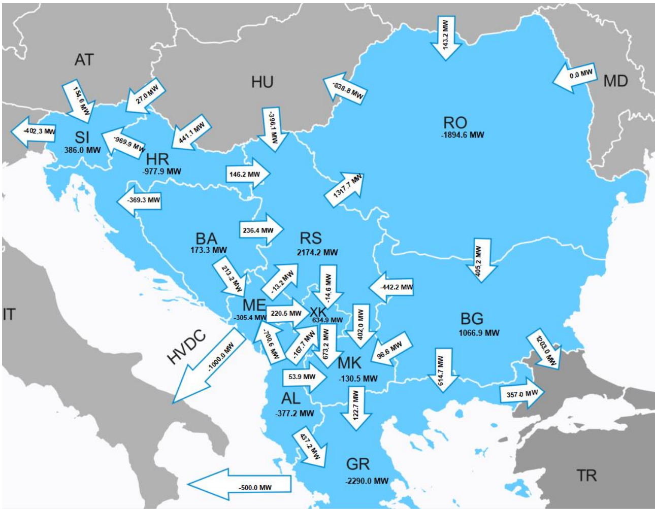
Figure 8.39: Cross-border exchanges (MW) and directions between the countries for Summer Off-Peak regime 2030 (high RES, referent CO2)
