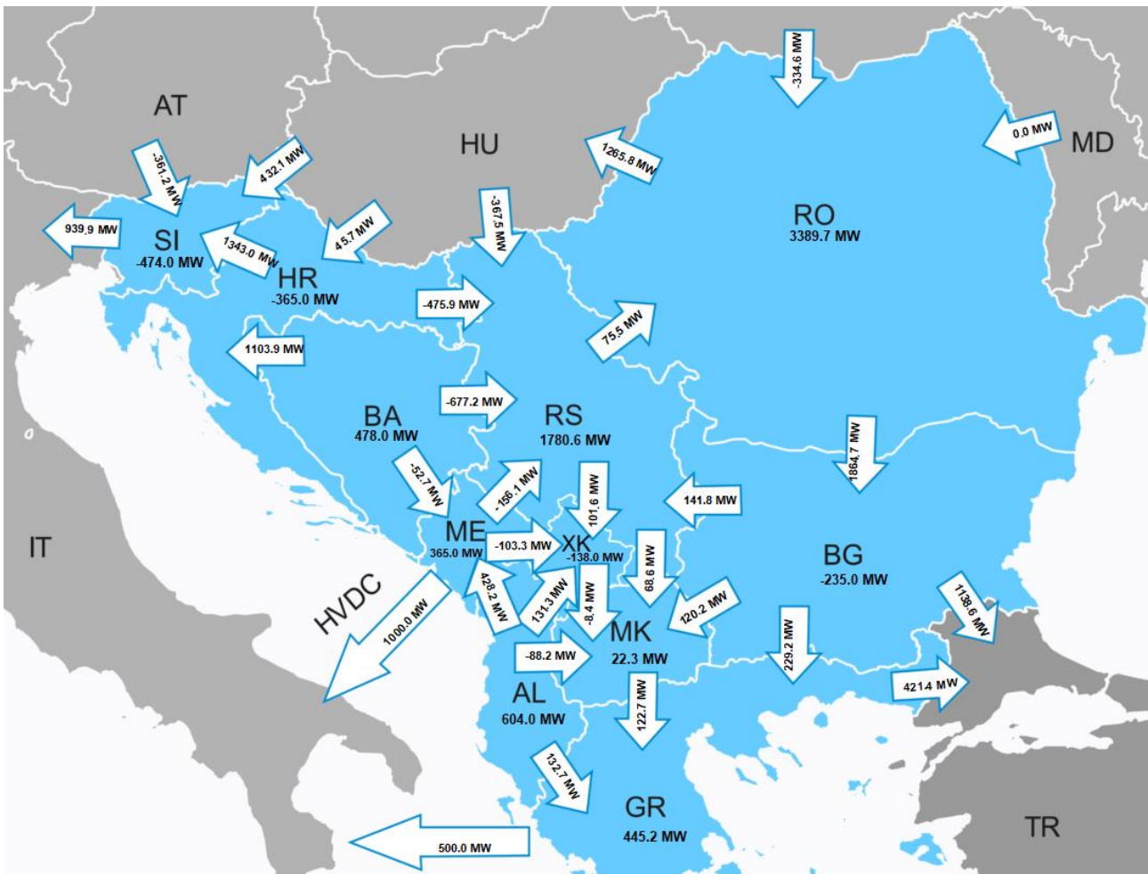
Figure 8.26: Cross-border exchanges (MW) and directions between the countries for Winter Peak regime 2030 (referent RES, referent CO2)
