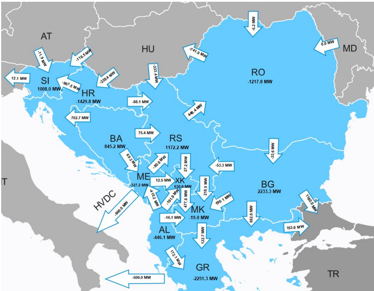
Figure 8.2: Cross-border exchanges (MW) and directions between the countries for Summer Off-Peak regime 2025 (referent RES, referent CO2)
