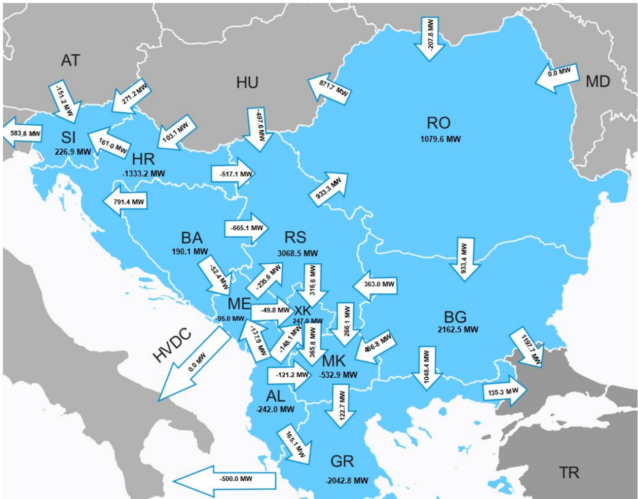
Figure 8.3: Cross-border exchanges (MW) and directions between the countries for Highest wind+solar generation regime 2025 (referent RES, referent CO2)
