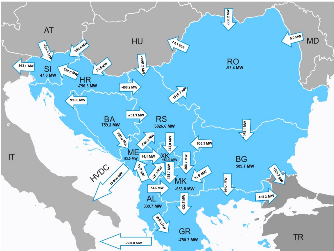
Figure 8.30: Cross-border exchanges (MW) and directions between the countries for Highest export regime 2030 (referent RES, referent CO2)
