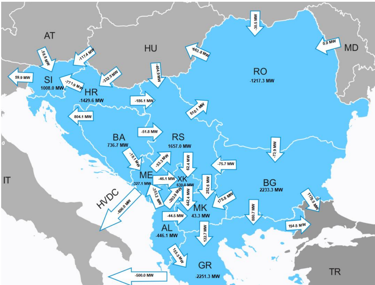
Figure 8.14: Cross-border exchanges (MW) and directions between the countries for Summer Off-Peak regime 2025 (high RES, referent CO2)
