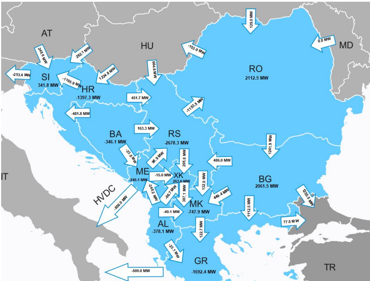
Figure 8.6: Cross-border exchanges (MW) and directions between the countries for Highest import regime 2025 (referent RES, referent CO2)
