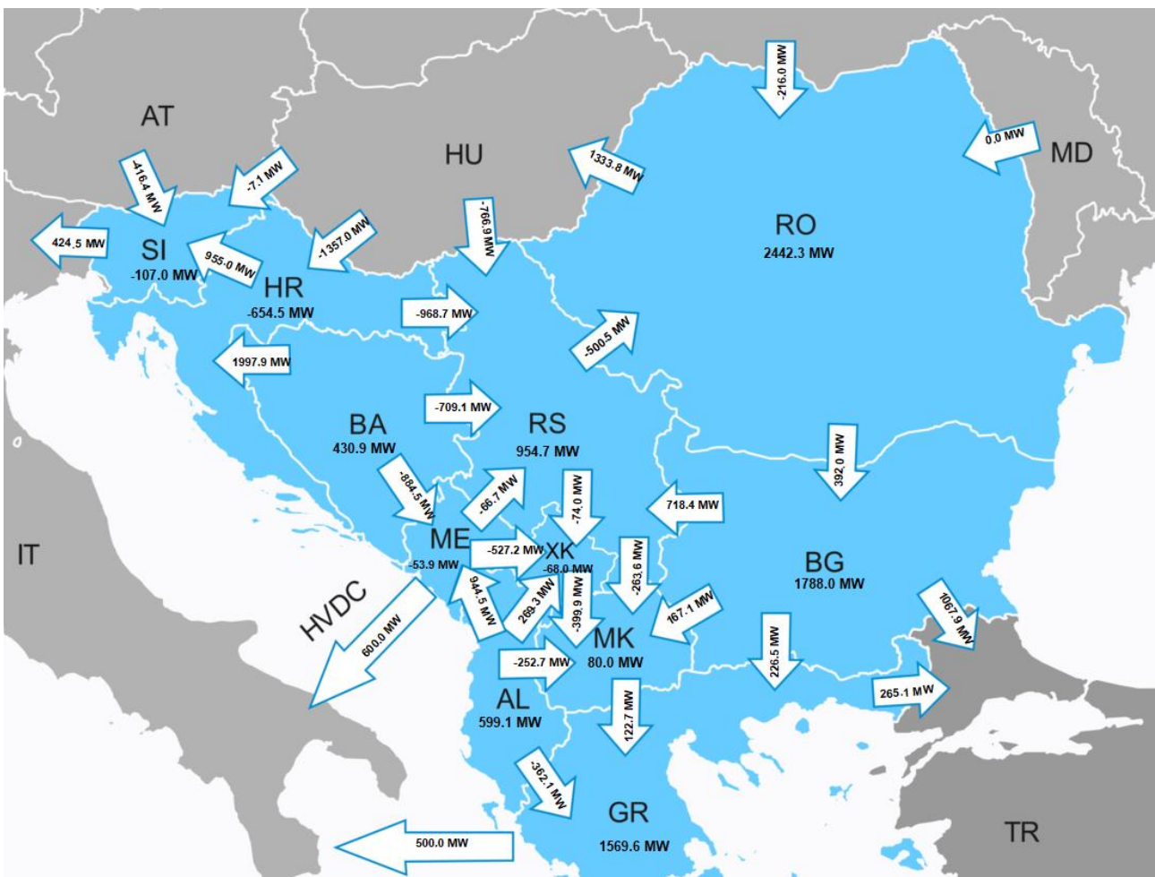
Figure 8.1: Cross-border exchanges (MW) and directions between the countries for Winter Peak regime 2025 (referent RES, referent CO2)
