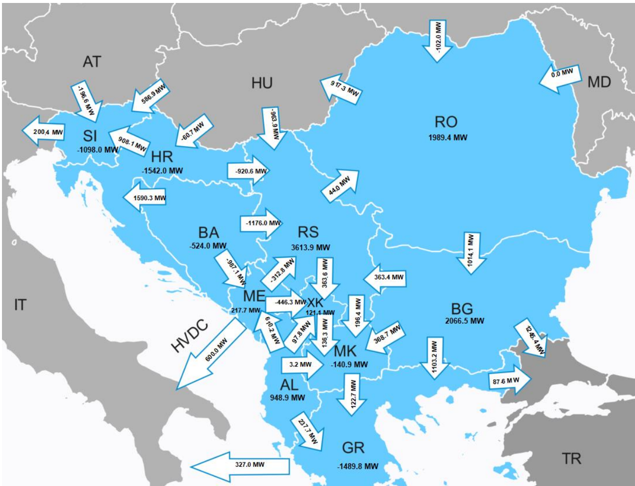
Figure 8.16: Cross-border exchanges (MW) and directions between the countries for Summer regime with the highest generation 2025 (high RES, referent CO2)
