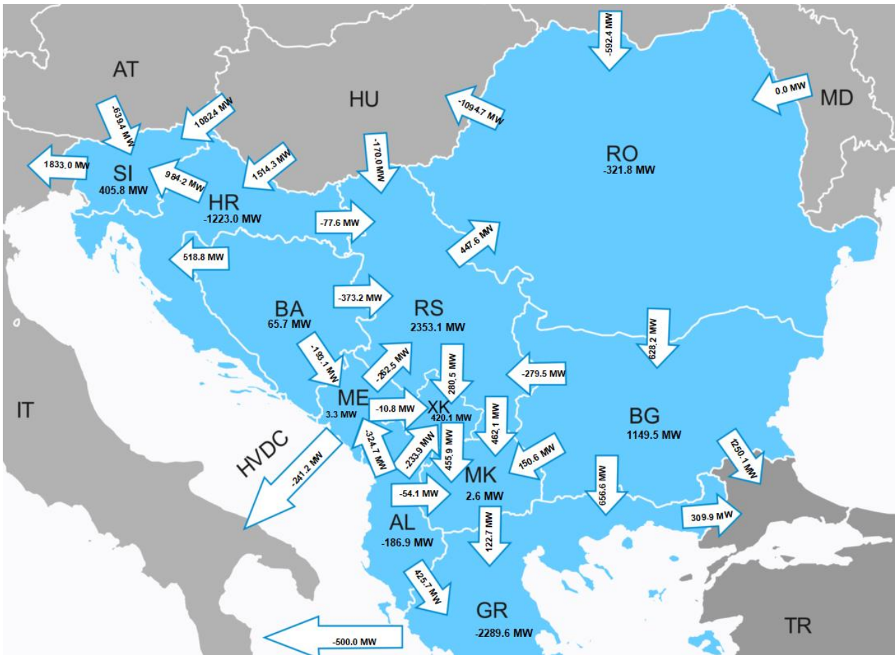
Figure 8.27: Cross-border exchanges (MW) and directions between the countries for Summer Off-Peak regime 2030 (referent RES, referent CO2)
