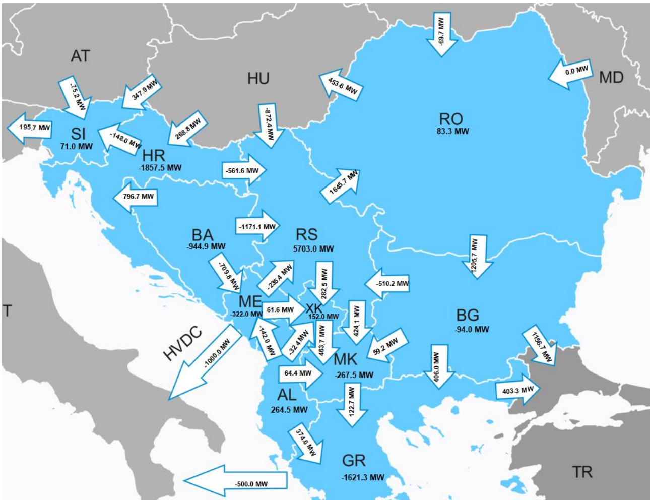
Figure 8.41: Cross-border exchanges (MW) and directions between the countries for Summer regime with the highest generation 2030 (high RES, referent CO 2 )
