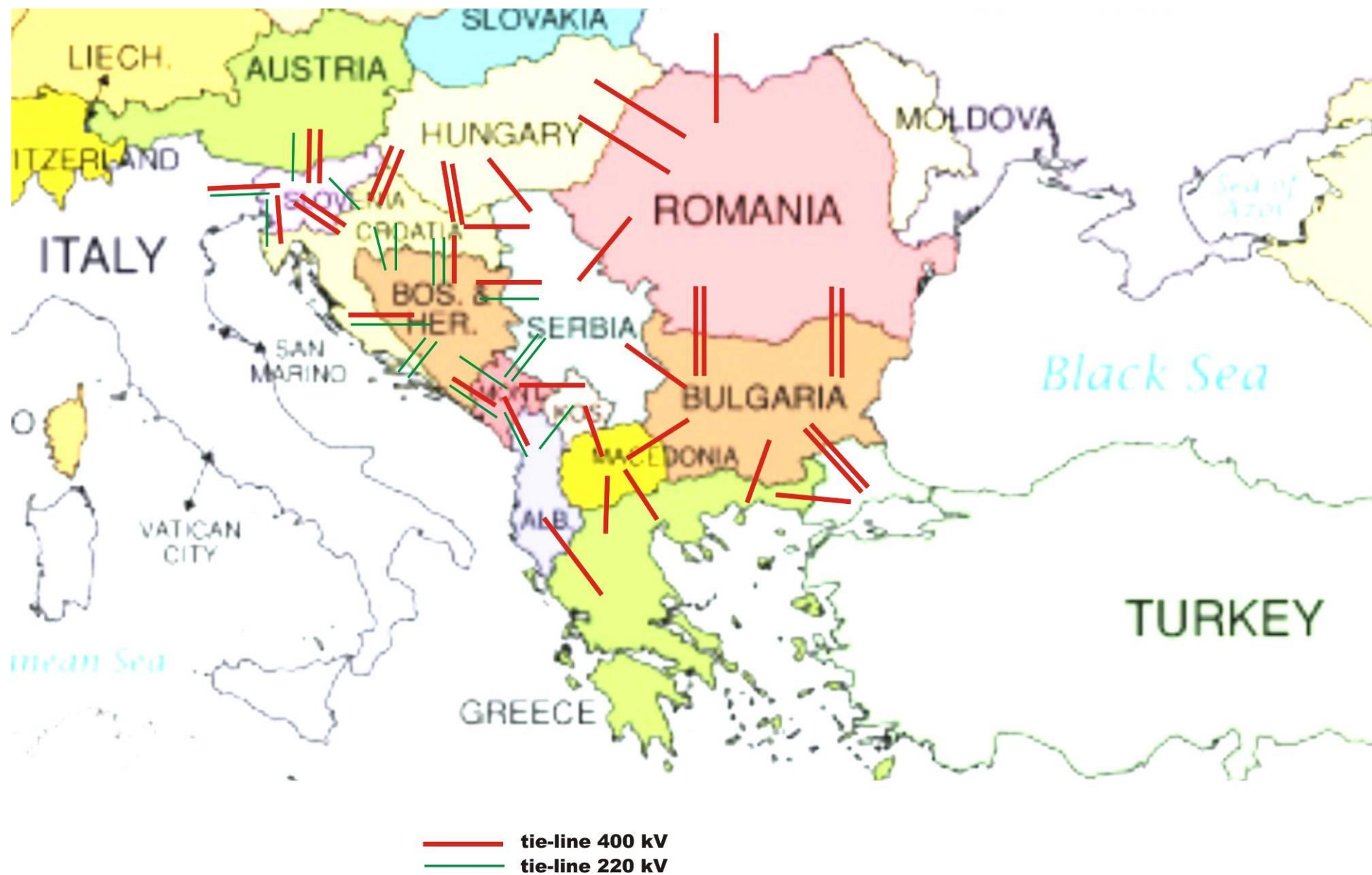
Figure 7.1 Existing tie-lines 400 kV and 220 kV in the SEE region
