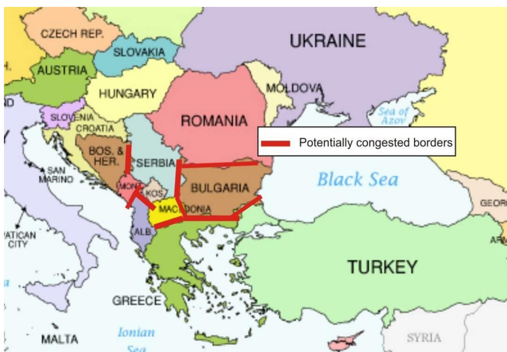
Figure 5.1 Borders with small cross-border capacity (NTC < 300 MW, based on calculations using PSS/E model in 2012, and evaluating all network elements 400 kV, 220 kV and 110 kV)
