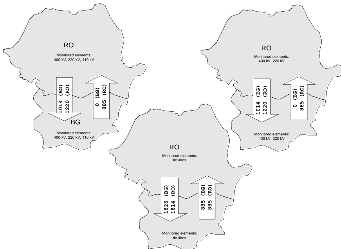
Figure 6.7 Calculated NTC values for Bulgaria/Romania border depending on the monitored elements (model 2012)
