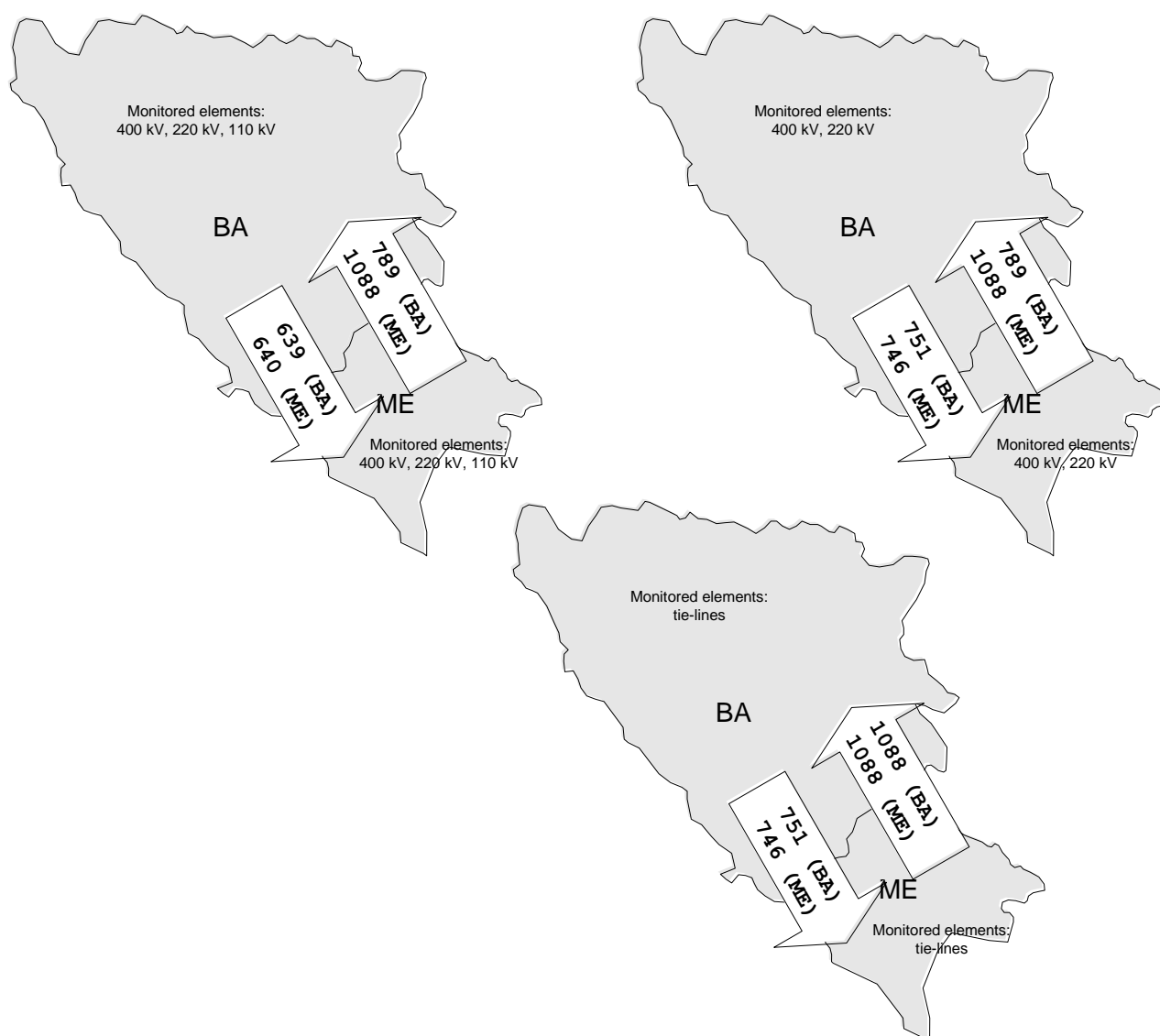
Figure 6.6 Calculated NTC values for BiH/Montenegro border depending on the monitored elements (model 2012)
