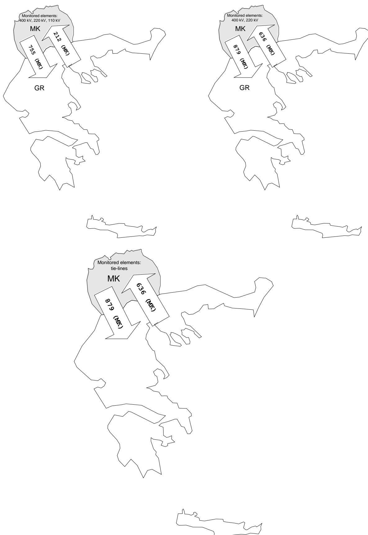
Figure 6.17 Calculated NTC values for the Macedonia/ Greece border depending on the monitored elements (model 2012)
