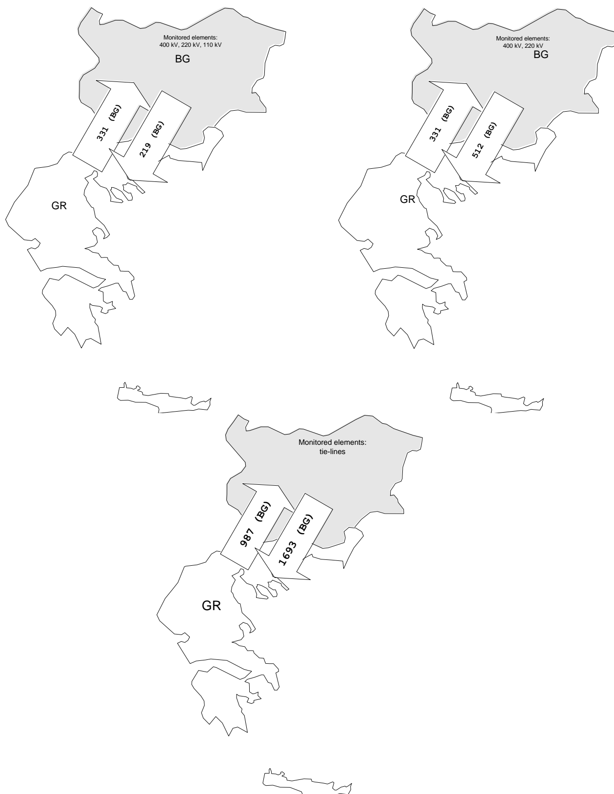
Figure 6.10 Calculated NTC values for the Bulgaria/Greece border depending on the monitored elements (model 2012)
