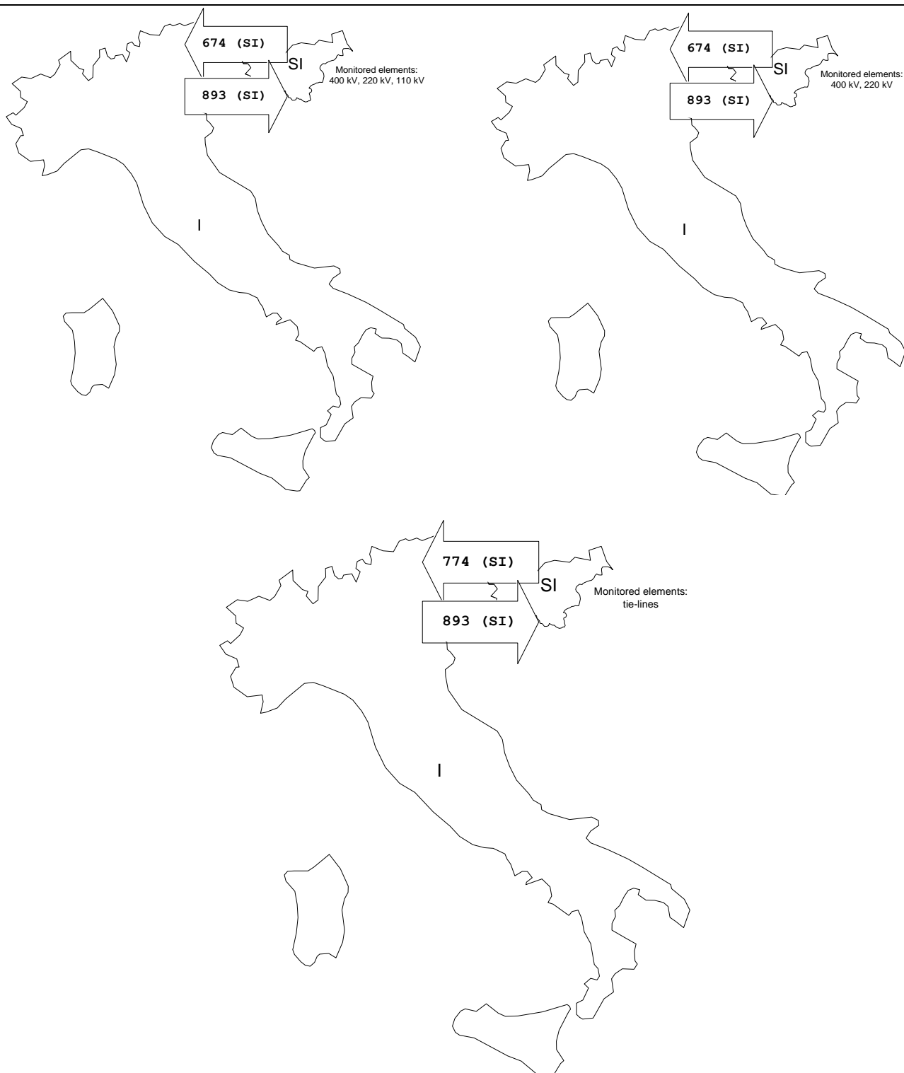
Figure 6.22 Calculated NTC values for the Slovenia/ Italy border depending on the monitored elements (model 2012)
