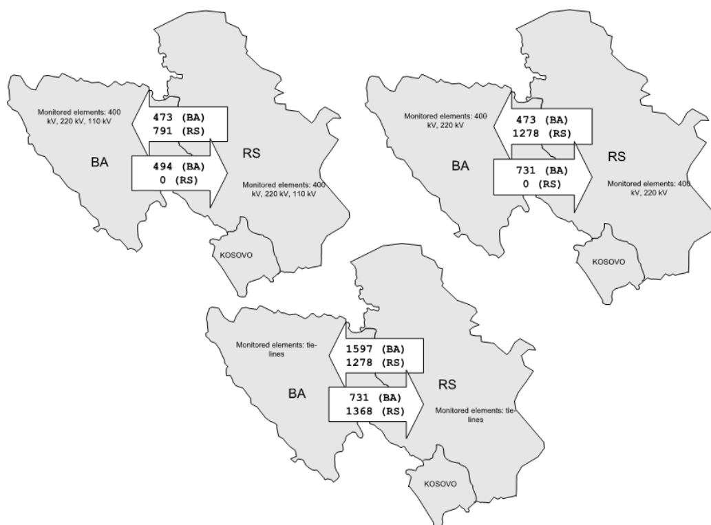
Figure 6.5 Calculated NTC values for BiH/Serbia border depending on the monitored elements (model 2012)
