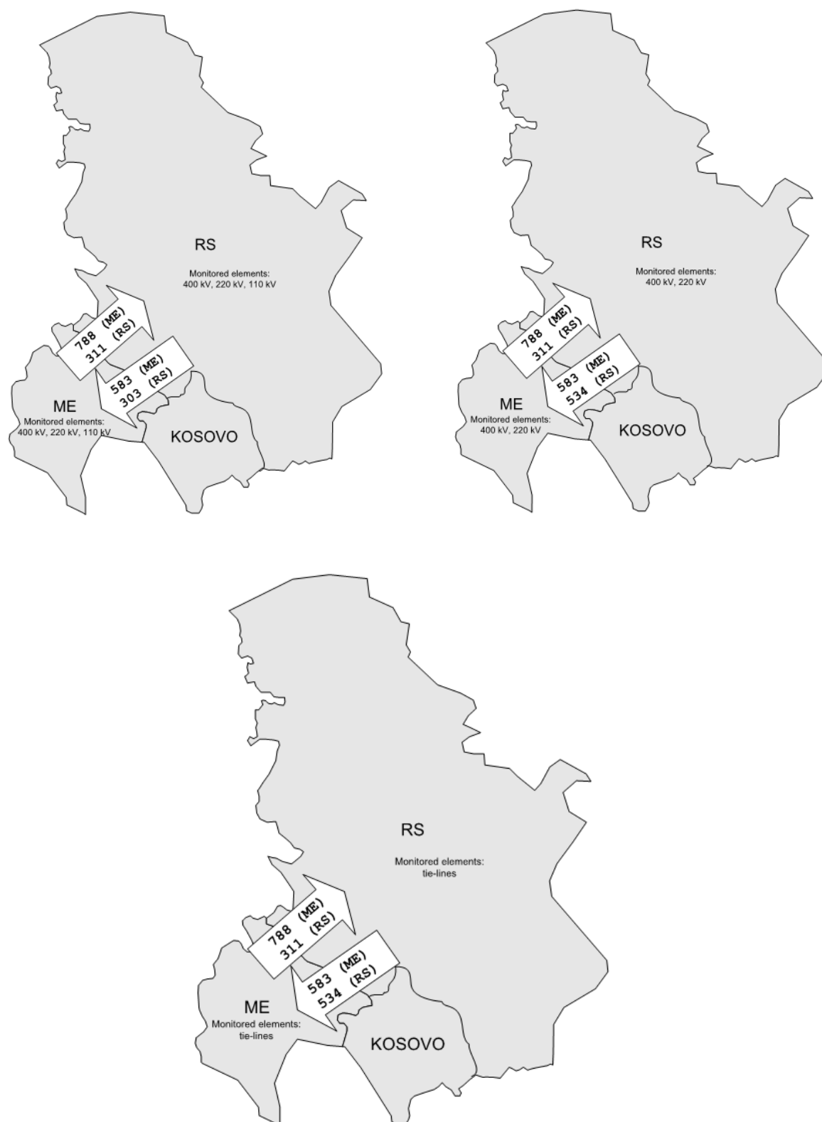
Figure 6.15 Calculated NTC values for the Montenegro/Serbia & Kosovo border depending on the monitored elements (model 2012)
