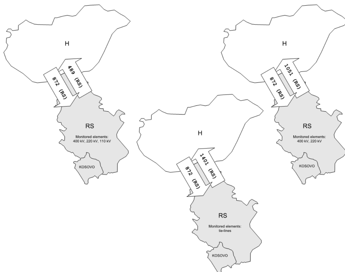
Figure 6.21 Calculated NTC values for the Serbia/ Hungary border depending on the monitored elements (model 2012)
