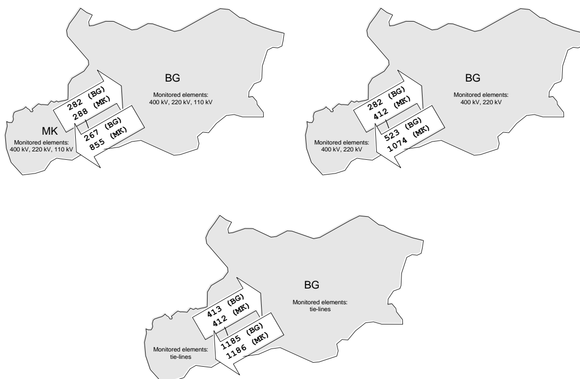
Figure 6.9 Calculated NTC values for the Bulgaria/Macedonia border depending on the monitored elements (model 2012)
