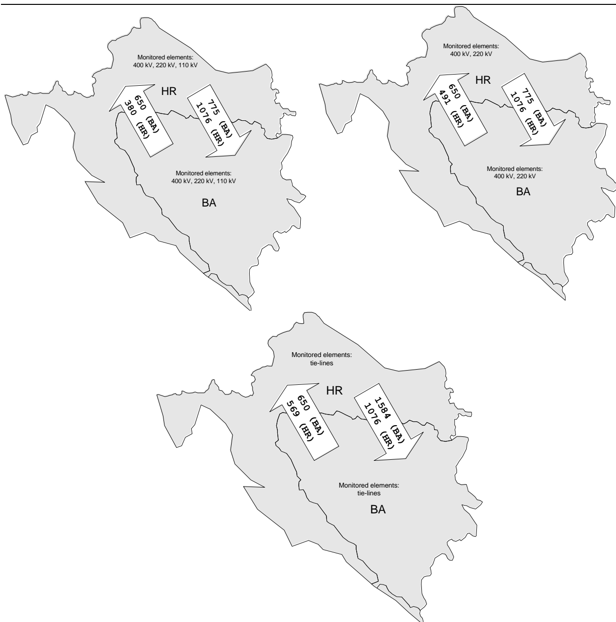
Figure 6.4 Calculated NTC values for BiH/Croatia border depending on the monitored elements (model 2012)
