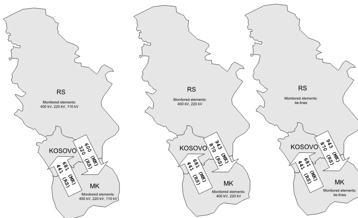
Figure 6.16 Calculated NTC values for the Macedonia/ Kosovo border depending on the monitored elements (model 2012)
