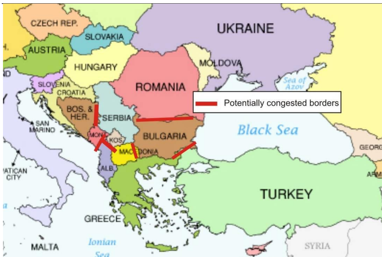
Figure 5.3 Borders with small cross-border capacity (NTC < 300 MW, based on calculations using PSS/E model in 2012, and evaluating all network elements 400 kV and 220 kV)
