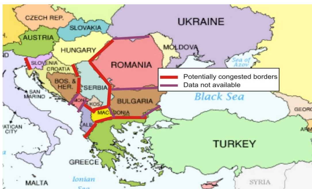
Figure 5.2 Borders with small cross-border capacity (NTC < 300 MW, based on the ENTSO-E data on indicative annual NTC values for 2012)
