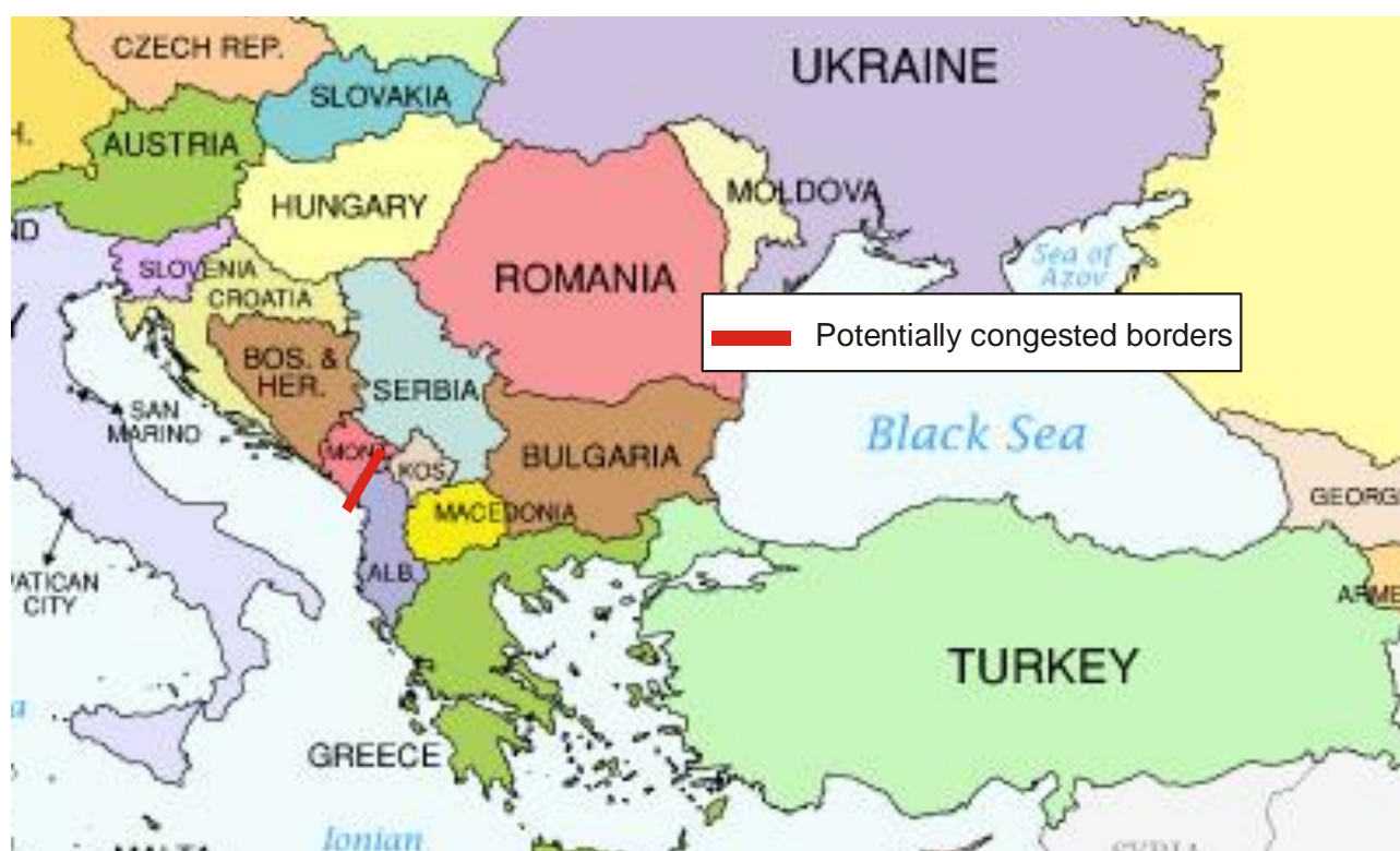
Figure 5.4 Borders with small cross-border capacity (NTC < 300 MW, based on calculations using PSS/E model in 2012, and observing interconnection lines 400 kV and 220 kV only)
