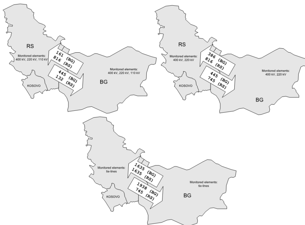
Figure 6.8 Calculated NTC values for Bulgaria/Serbia border depending on the monitored elements (model 2012)
