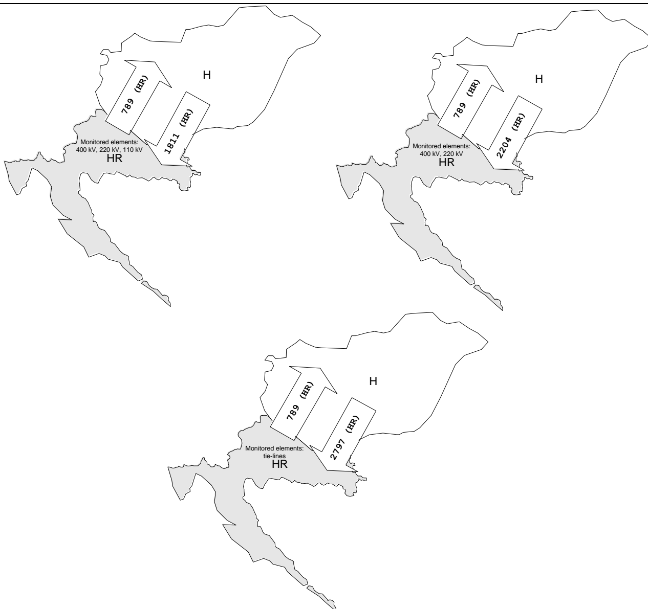
Figure 6.13 Calculated NTC values for the Croatia/Hungary border depending on the monitored elements (model 2012)
