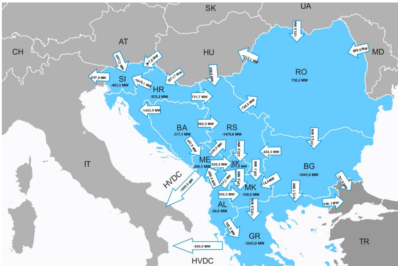
Figure 53: Cross-border exchanges (MW) and directions between the countries in the scenario: Moderate decarbonization - Average hydrology – maximum EMI regional electricity exchange 2030
