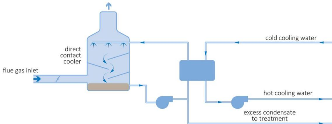
**Figure 9 Direct contact flue gas condensing system** (Foster Wheeler Italiana, 2011)
