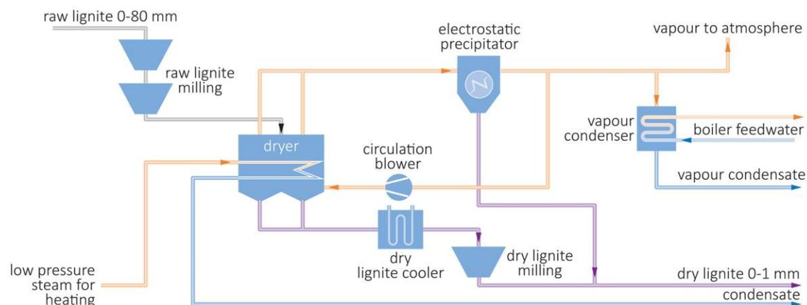
**Figure 4** WTA™ lignite drying process as used in the prototype at Niederaussem (Henderson, 2013)
