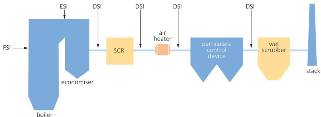
**Figure 7 Possible sorbent injection points** (Carpenter, 2012)
