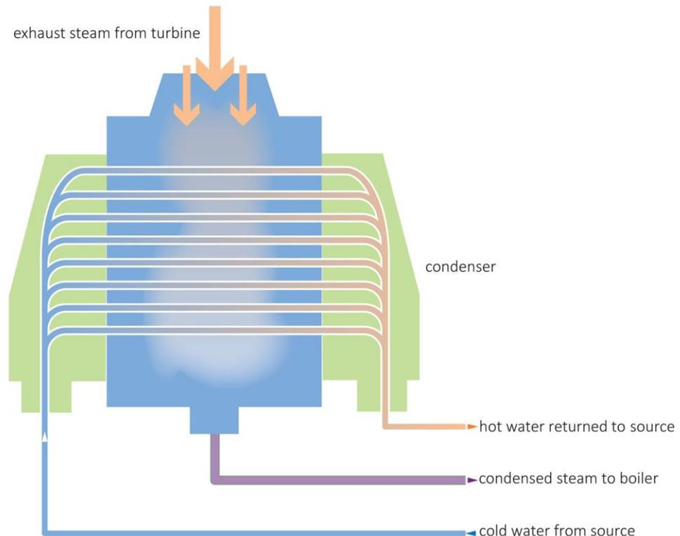
**Figure 11** Water flow in a steam condenser (Bushart, 2014)
