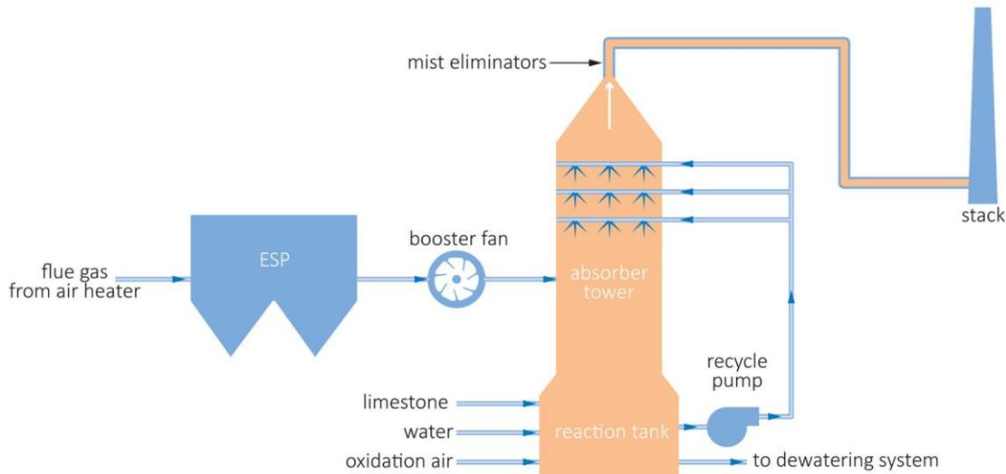
**Figure 6** A typical limestone wet scrubber system (Carpenter, 2012)
