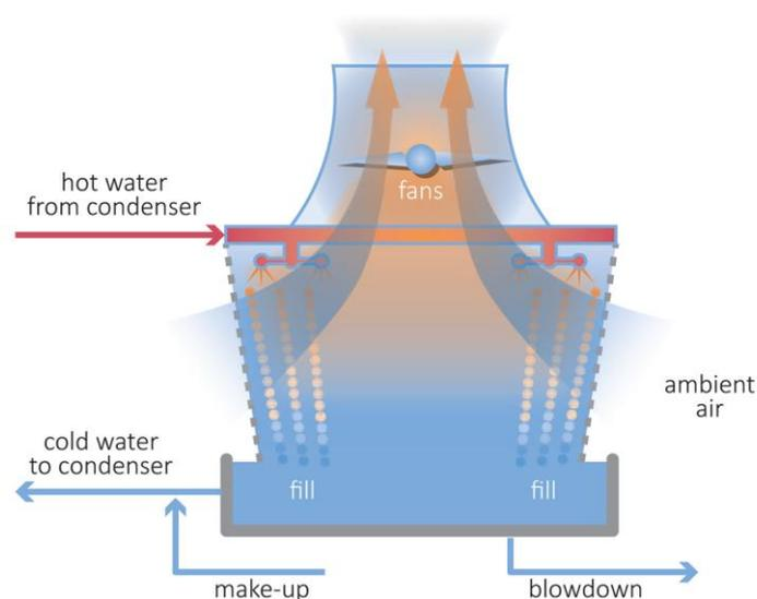
Figure 12 Water flow in an induced draught cooling tower (Bushart, 2014)
