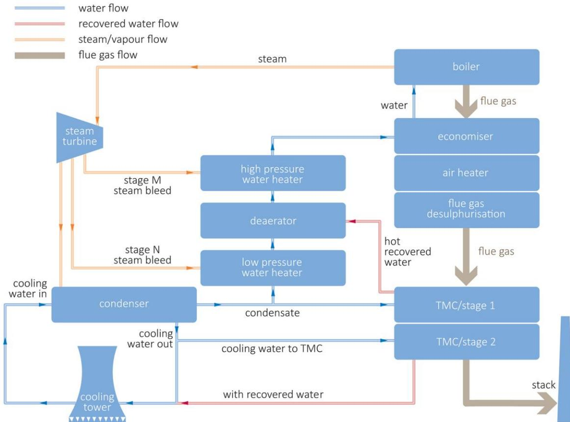
Figure 10 Two-stage TMC integration in a coal-fired power plant (Wang and others, 2016b)
