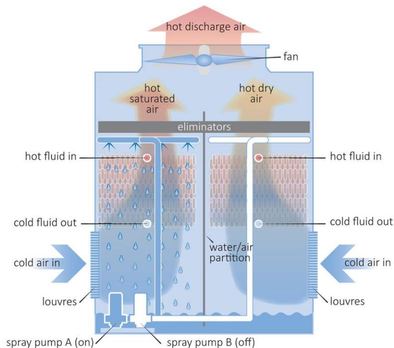
**Figure 16** A dual coil closed-circuit cooling system (Libert and Nevins, 2011)
