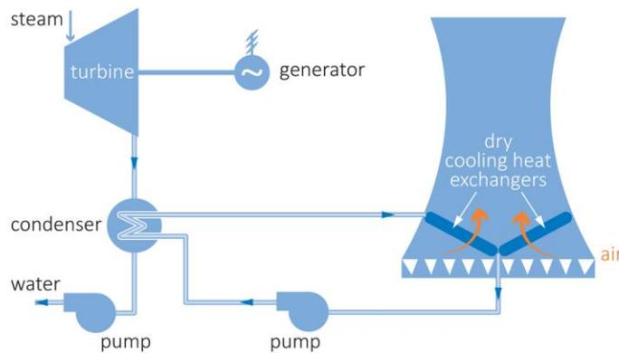
**Figure 15 Indirect dry cooling** (Couch, 2005)
