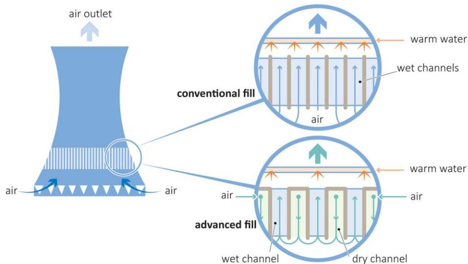
**Figure 13 Schematic of proposed fill arrangement** (EPRI and Maulbetsch Consulting, 2012)
