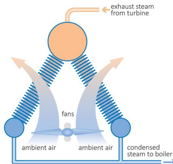
Figure 14 Direct dry cooling with mechanical draught ACC (Bushart, 2014)
