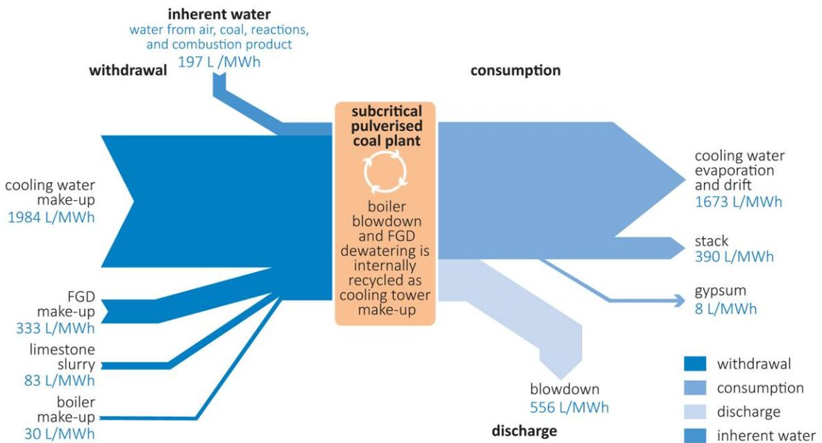
Figure 2 Water balance on a subcritical 500 MW power plant (Carney and Shuster, 2014)
