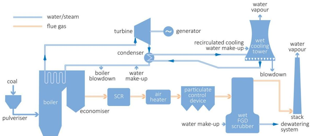
Figure 1 Schematic of a power plant showing where water is lost and added
