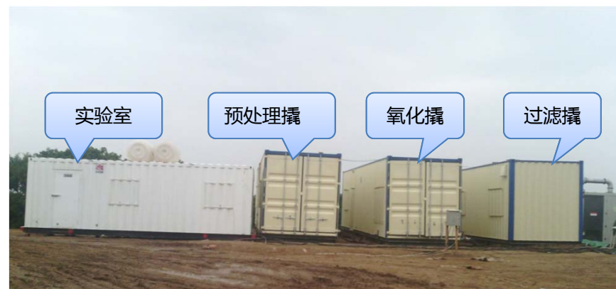
延页平1井压裂返排液处理装置及处理现场 The site of recycling and utilizing
