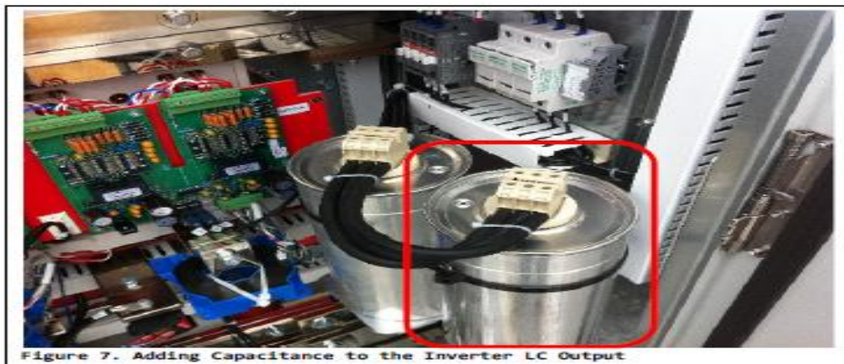
Figure 7. Adding Capacitance to the Inverter LC Output
