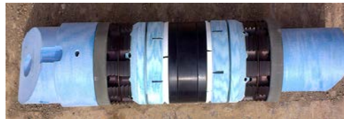
Drillable plug (cost reduced from 200,000RMB to 25,000 RMB)
