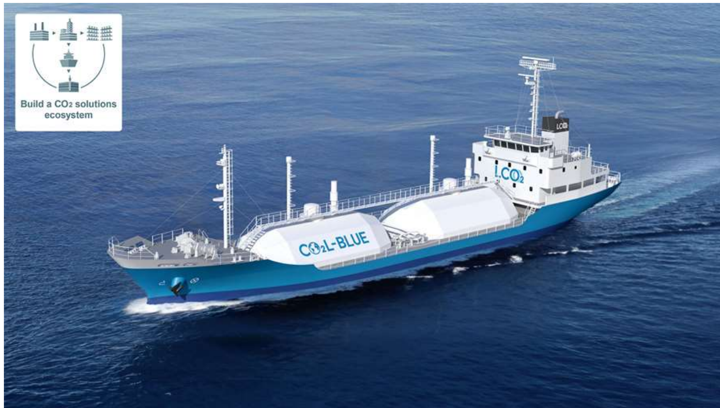
Conceptual image of Mitsubishi Shipbuilding Co.'s liquefied CO2 demonstration test ship Source: Mitsubishi Shipbuilding Co. & Bloomberg.com
