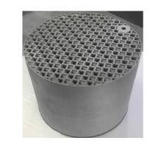
ORNL prints intensified devices with heat exchanger integrated into pack ION uses 3D Printing to develop internal absorber mass transfer and heat exchange
