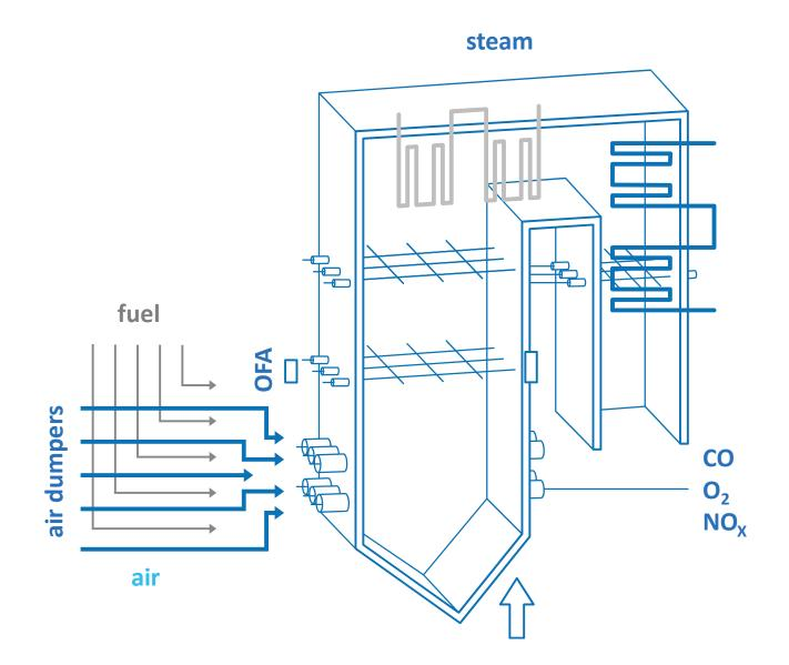
Coal fired boilers – emission problems – "hard" solution redesign and modernization of burners, dumpers, combustion chamber
