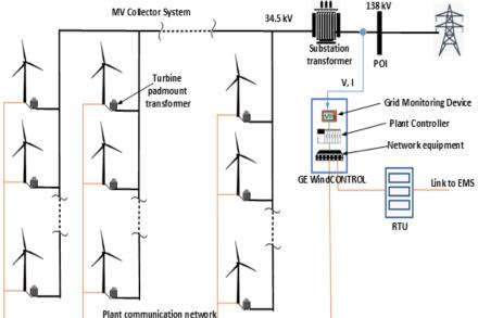
Each inverter performs its own energy production based on local wind speed, however the PPC coordinates the output to provide typical large power-plant services
