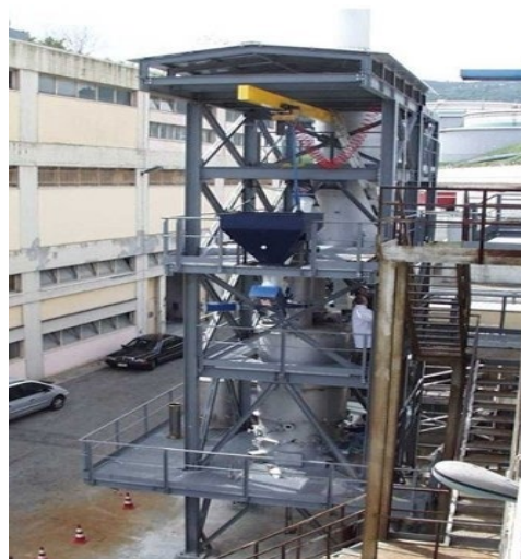
The University of Alaska-Fairbanks is testing a modular gasification system design for producing syngas from local coal resources in challenging environments. Photo: NETL
