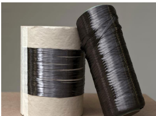
Carbon fibers (shown on spools) are lighter and stronger in comparison to traditional metals.
