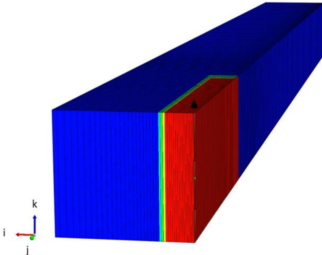
To capture the impact of hydraulic stimulation on the performance of the Mowry Shale horizontal well, a Stimulated Reservoir Volume (SRV) was established in the model (shown as the red grid blocks in Figure 4-12). Figure 4-13 provides information on the SRV dimensions and enhanced permeability value derived from the history match of the Central Basin Study Area Mowry Shale type well.
