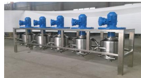
1m 3 /h超重力萃取脱酚中试 1m 3 / h super gravity extraction phenol removal test
