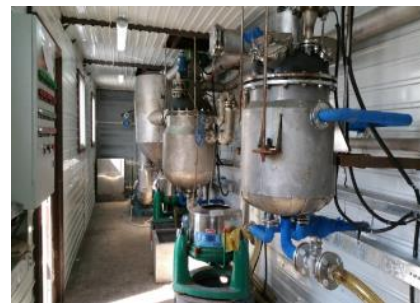
1m 3 /h超重力萃取脱酚中试 1m 3 / h super gravity extraction phenol removal test
