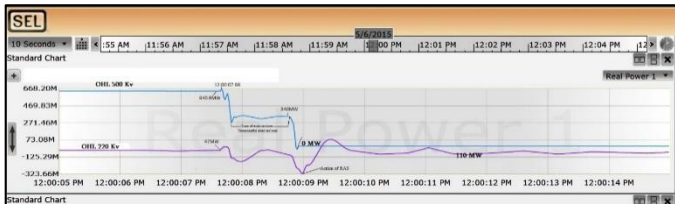
Fig. 9 Phase Failure Over the 500 kV Imereti OHL Example.
