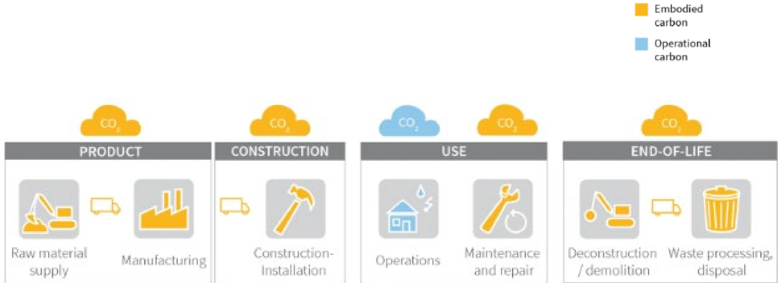
**Figure 1.** Embodied carbon (yellow) and operational carbon (blue) across the key life cycle stages of a building.
