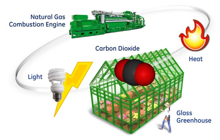
Greenhouse CHP combines the production of heat and power to enrich the greenhouse atmosphere with CO<sub>2</sub>, keep the temperature on a constant level and provide dispatchable power for lighting so that harvest yield can be significantly increased.
