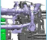
Two-stage turbochargers have a higher charging pressure enabling better heat recovery
