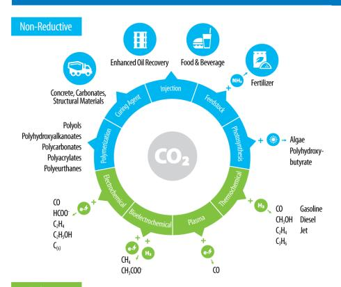
CO<sub>2</sub> can be utilized directly (nonreductive utilization) or undergo chemical transformation (reductive utilization) as precursor to other products
