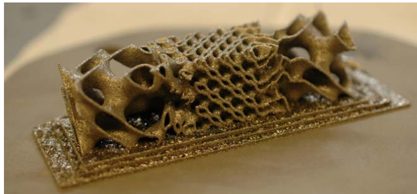
Heat exchanger internals printed in Inconel 625.
