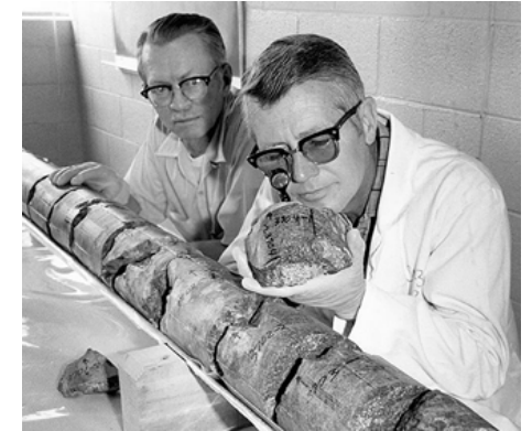
Los Alamos scientists examine a core sample taken from a depth of 13,700 feet at the Fenton Hill geothermal test site.
