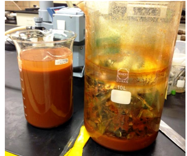
Figure 1: Images of: iron(III) hydroxide (as hydrolysis product, left) and resulted unreacted HDD parts (right) after reaction with copper(II) chloride
