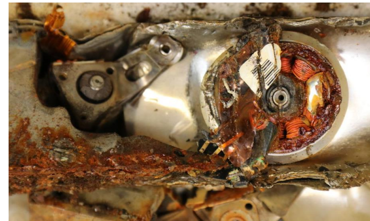
Figure 2: Image of some parts of shredded hard disk drives after acid-free dissolution reaction
