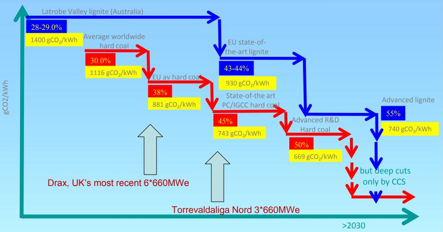
Data for hard coal-fired power plants from VGB 2007; data for lignite plants from C Henderson, IEA Clean Coal Centre; efficiencies are LHV,net Energy Efficiency makes big change but deep cuts of CO<sub>2</sub> emission can be done only by Carbon Capture and Storage (CCS)
