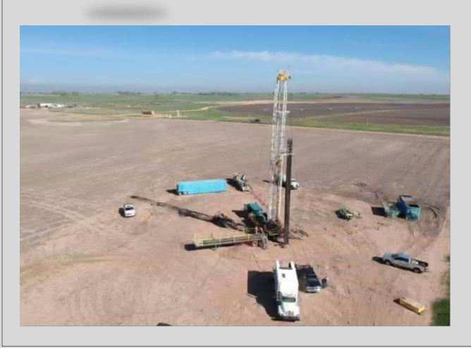
Rig 7 - Rig, Pump Truck, Wireline Truck, Tank, Pit
