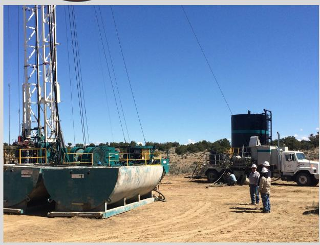
Rig 6 - Rig, Pump Truck, Wireline Truck, Tank, Pit
