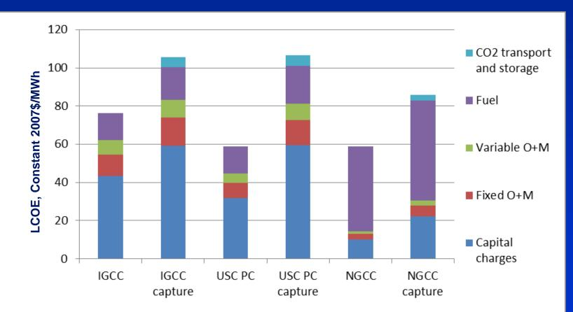
Bituminous coal: \$1.6/GJ (LHV), Gas: \$7/GJ (LHV), Annual capital charge factor: 0.11 CO2 transport + storage: \$6/t, 90% load factor
