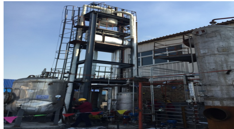
Pilot plant test for hetero-oxo-synthesis of methanol and syngas and its hydrogenation to ethanol
