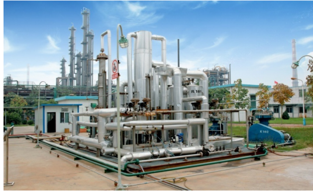
Demonstrate device in Yima, Henan Province, with a capacity of 200 Nm 3 /h syngas
