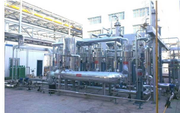
Demonstrate device in Guanghui Ltd., Xinjiang Region, with a capacity of 6000 Nm 3 /d SNG
