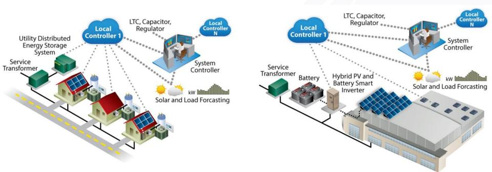
Through its SHINES project, EPRI is working with several utilities to design, develop, and demonstrate technology for end-to-end grid integration of energy storage and load management with PV generation. The technology is a simple, two-level, optimized control architecture.
