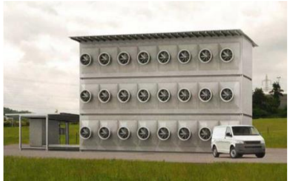
Impression of a 'dry' amine-based sorbent CO 2 air capture system; Credit: Climeworks
