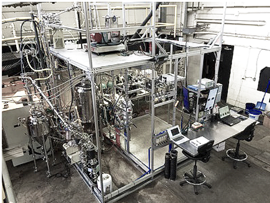
H Quest's engineering-scale Wave Liquefaction™ pilot system in the high bay of the U-PARC facility
