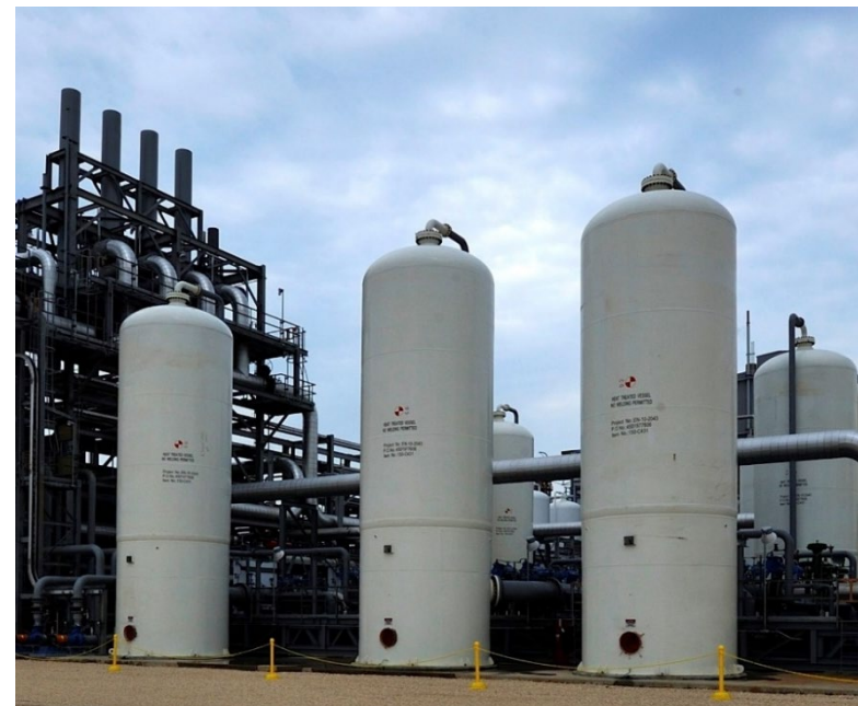
Air Products and Chemicals, Inc. (APCI) Port Arthur, TX Industrial Carbon Capture and Storage (ICCS) project is demonstrating CO 2 capture and storage of steam methane reforming process gas used for large-scale hydrogen production
