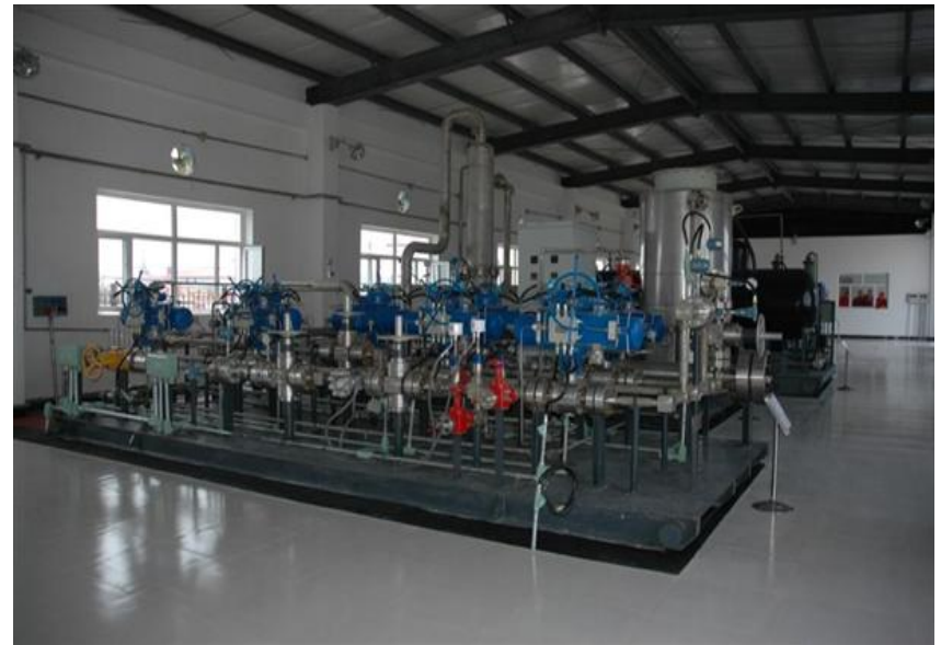
The First Real-time Corrosion Testing System in China 中国首套中试腐蚀在线检测装置 (Jilin Oilfield 吉林油田, 2010)
