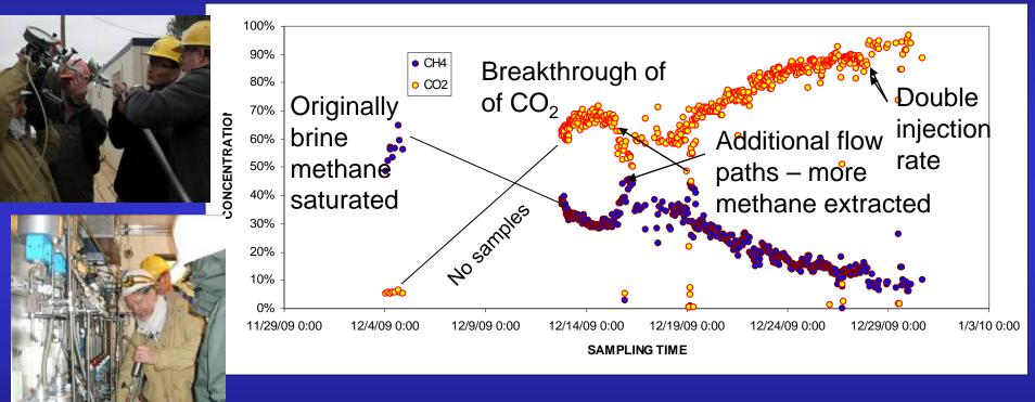
Small diameter sampler with N<sub>2</sub> drive brings fluids quickly to surface with tracers intact CO<sub>2</sub> dissolution into brine liberates dissolved CH<sub>4</sub> BEG, LBNL, USGS, ORNL, UTDoG, data compiled by Changbing Yang BEG
