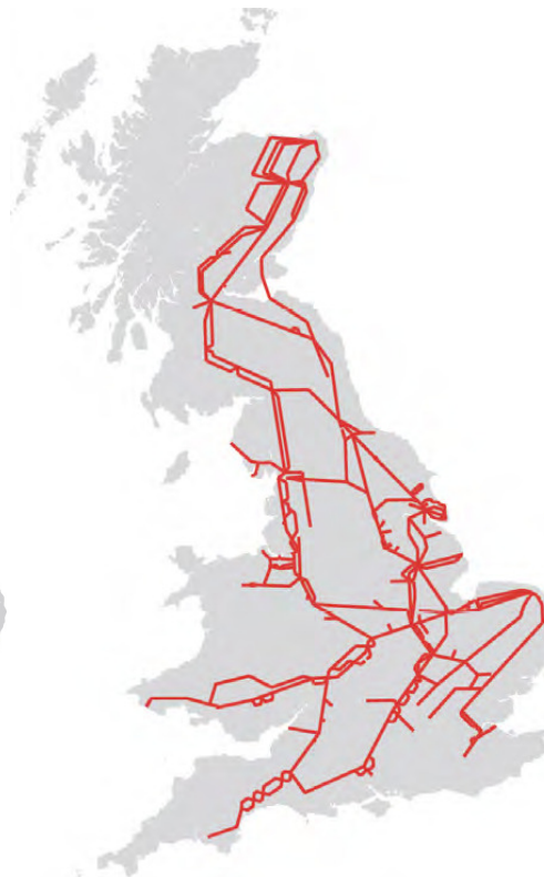
Transmission UK – gas system
