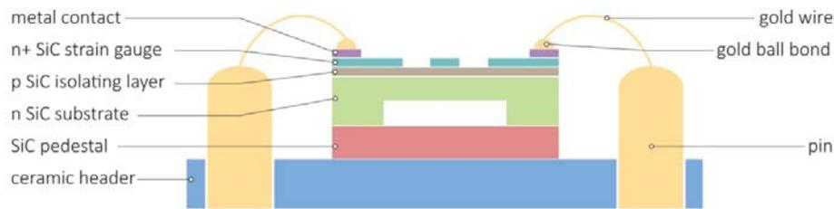
**Figure 31** A schematic of a SiC-based diaphragm pressure sensor (Hunter and others, 2006)
