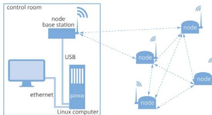
**Figure 32** A wireless mesh network (Taft, 2010)
