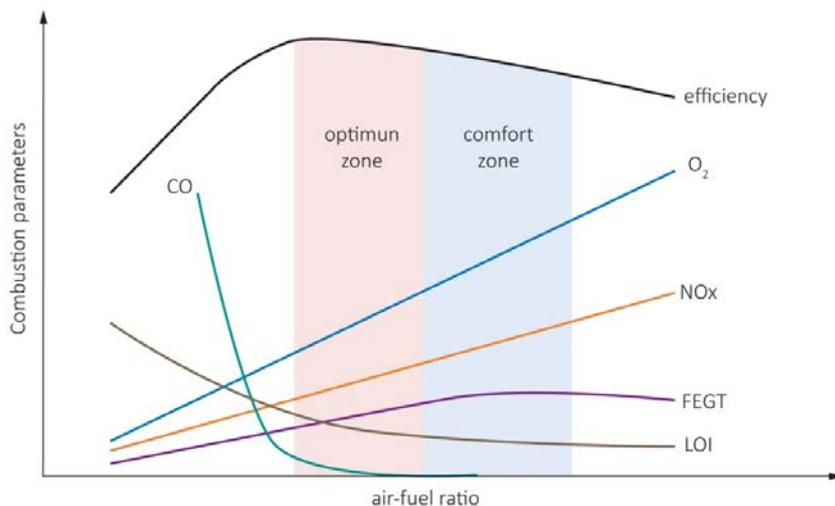
Figure 9 The variation of key combustion parameters with air-fuel ratio, showing the potential efficiency and emissions improvements achievable with optimised combustion (Widmer and Marquez, 2012)
