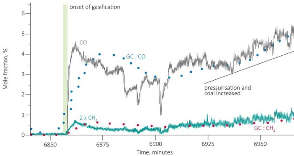
**Figure 26** Improved detection of the onset of gasification using TDLAS compared to gas chromatography (GC) (Hanson and others, 2014)
