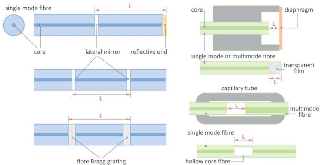
**Figure 19** Examples of intrinsic (left) and extrinsic (right) Fabry-Perot cavities
