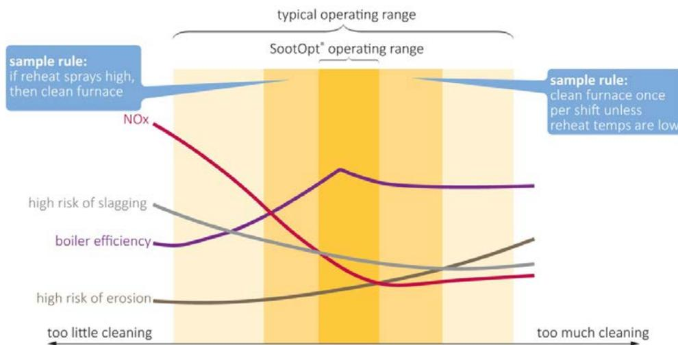
Figure 18 A graphic depiction of how optimised sootblowing can benefit several boiler parameters
