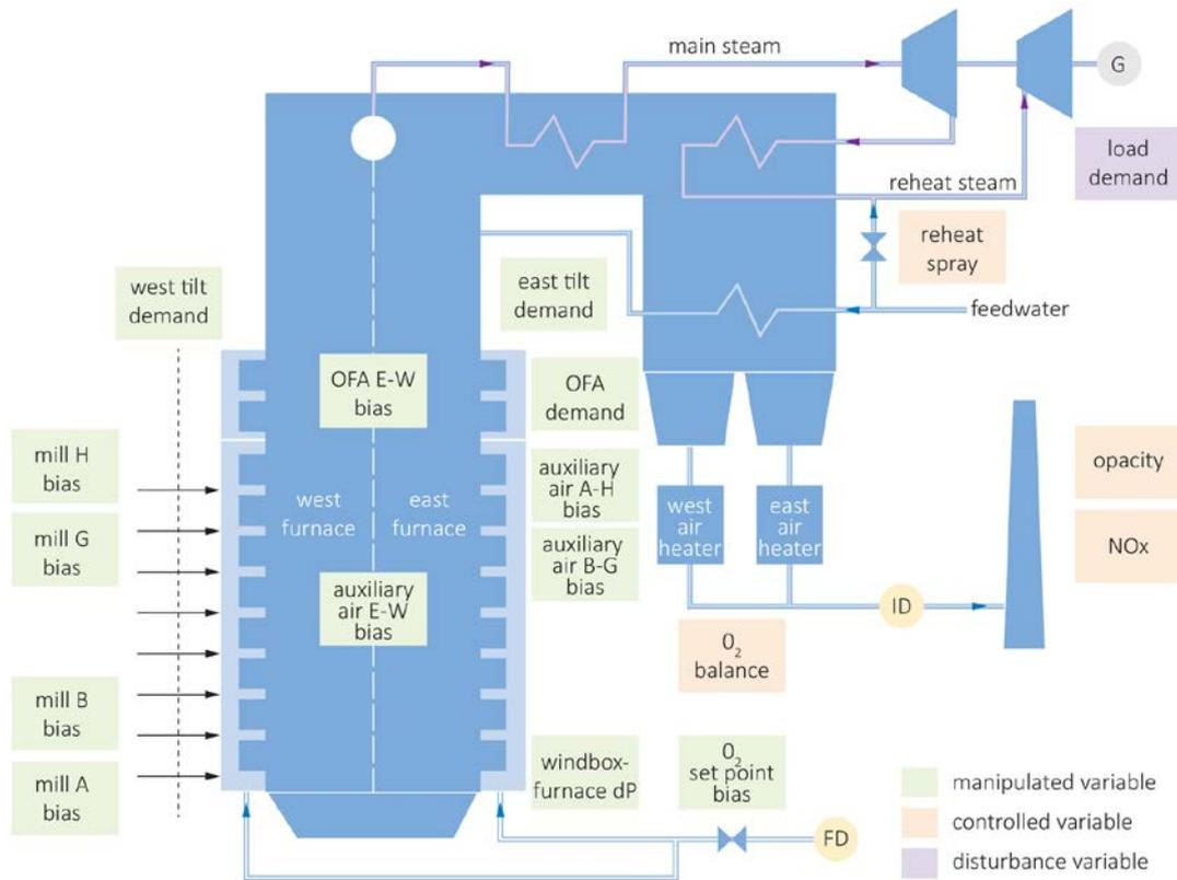
**Figure 15** A schematic of a coal boiler indicating key manipulated and controlled variables used by combustion optimisation systems, and the disturbance variable of unit load demand (Immonen and others, 2007)
