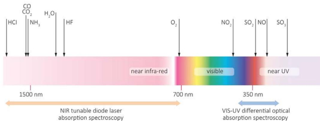
**Figure 12 Spectral regions for the detection of various combustion gases, including the near IR region addressed by tunable diode laser absorption spectroscopy (Hanson, 2014)**
