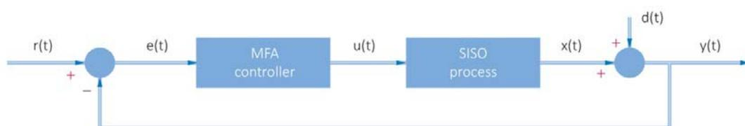
Figure 8 A single loop model-free adaptive control system, where  $y(t)$  is the process variable,  $r(t)$  the set point,  $e(t)$  the set point error,  $u(t)$  the control action generated by the MFA neural network, and  $d(t)$  are system disturbances (Cheng, 2005)
