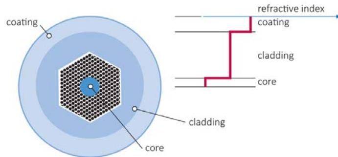
**Figure 23 Photonic crystal structure with a hollow core** (NKT Photonics, 2014)
