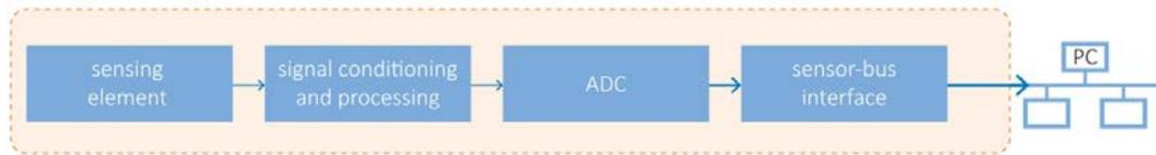
**Figure 1** A smart sensor integrated with signal processing and digital networking capability (ADC, analogue to digital converter)
