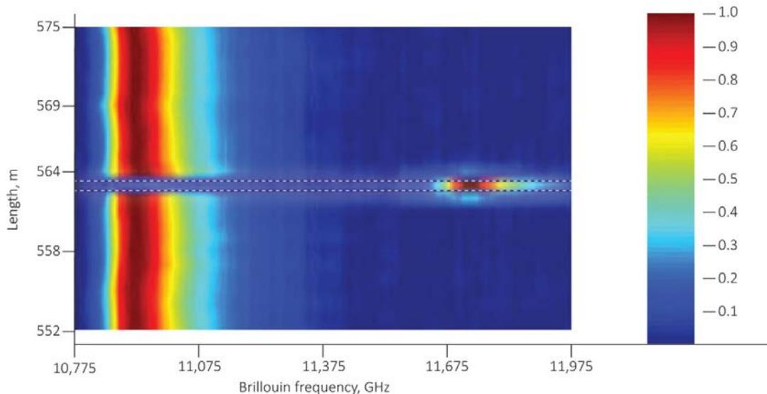
**Figure 25** Frequency shift of the reflected light corresponds to temperatures along the fibre, making it possible to detect a short heated section (Yu and Wang, 2014)
