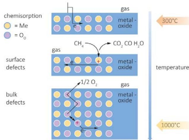
**Figure 30** Change in sensing mechanism of conductometric gas sensors with increasing temperature (Liu and others, 2014b)
