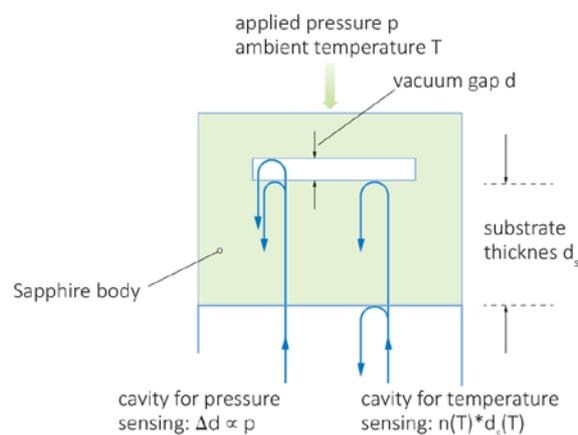
**Figure 20** An optical fibre capped with a micromachined sapphire tip acts as a high-temperature Fabry-Pérot interferometer sensor for temperature and pressure (Oxsensis, ND)
