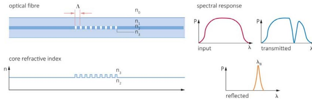
**Figure 21 Fibre Bragg gratings ( $n$ , refractive indices;  $\lambda$ , wavelength;  $P$ , power)**
