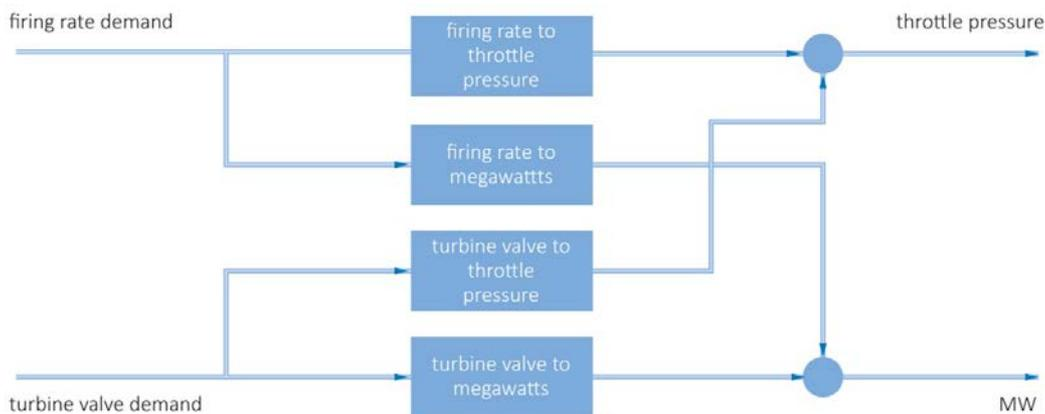
Figure 4 An example of two interacting control loops (EPRI, 1998)
