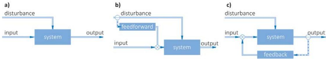
**Figure 2 a) Open loop, b) feedforward and c) closed loop (feedback) control**
