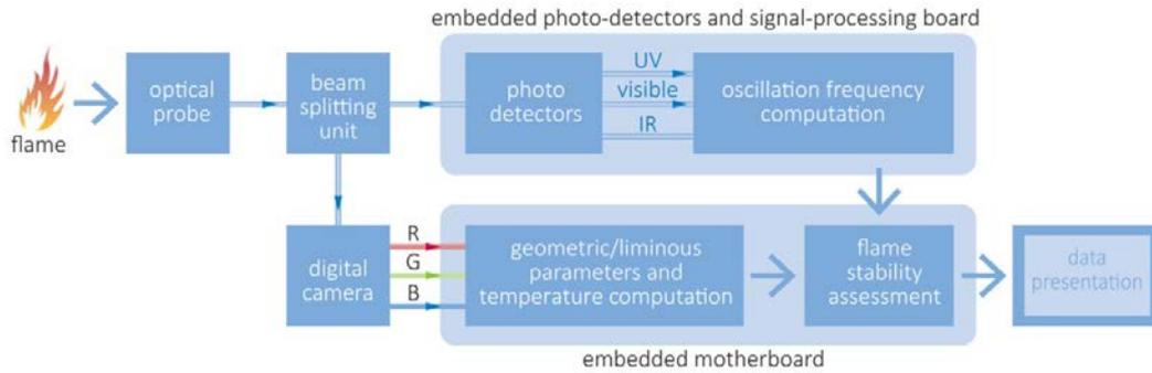
**Figure 27 A flame monitoring system combining both digital imaging and single point spectral measurements** (Sun and others, 2011)
