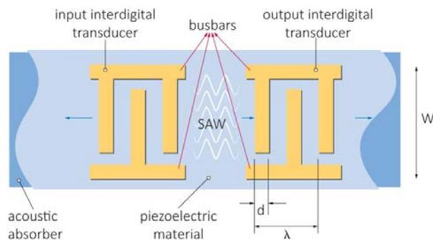
**Figure 33** Design of a wirelessly powered surface acoustic wave temperature sensor (Perreira and Maskay, 2014)
