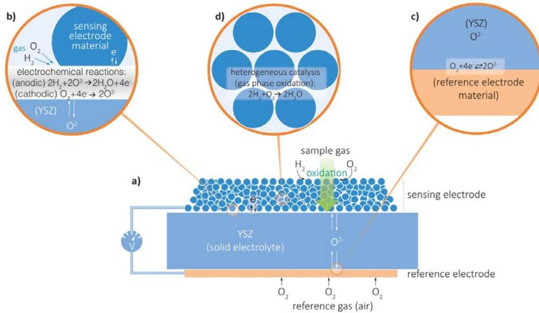
**Figure 29 Schematic of the basic structure and principle of a mixed potential YSZ sensor, showing  $\text{H}_2$  sensing** (Miura and others, 2014)
