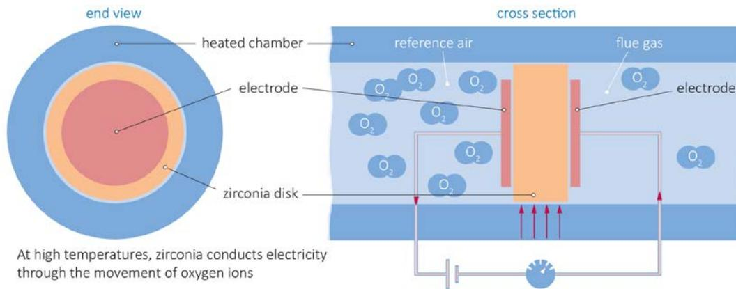
**Figure 10** A schematic of a typical zirconia-based oxygen sensor (Servomex, 2006)
