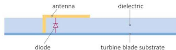
**Figure 34** wireless thin film temperature sensor from Wireless Sensor Technologies (Gregory and others, 2010)
