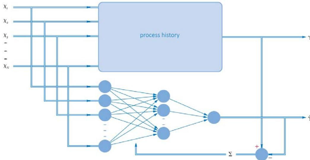
**Figure 6 Training a neural network by backpropagation. Weights are adjusted to minimise model error (Piche and Bartlett, 2008)**
