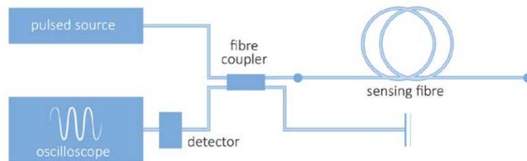
**Figure 24** A schematic of an OTDR arrangement
