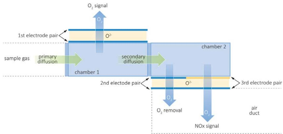
**Figure 28** A commercial NO<sub>x</sub> sensor based on amperometric cells and oxygen pumping (DeBarber and Mizutani, 2011)
