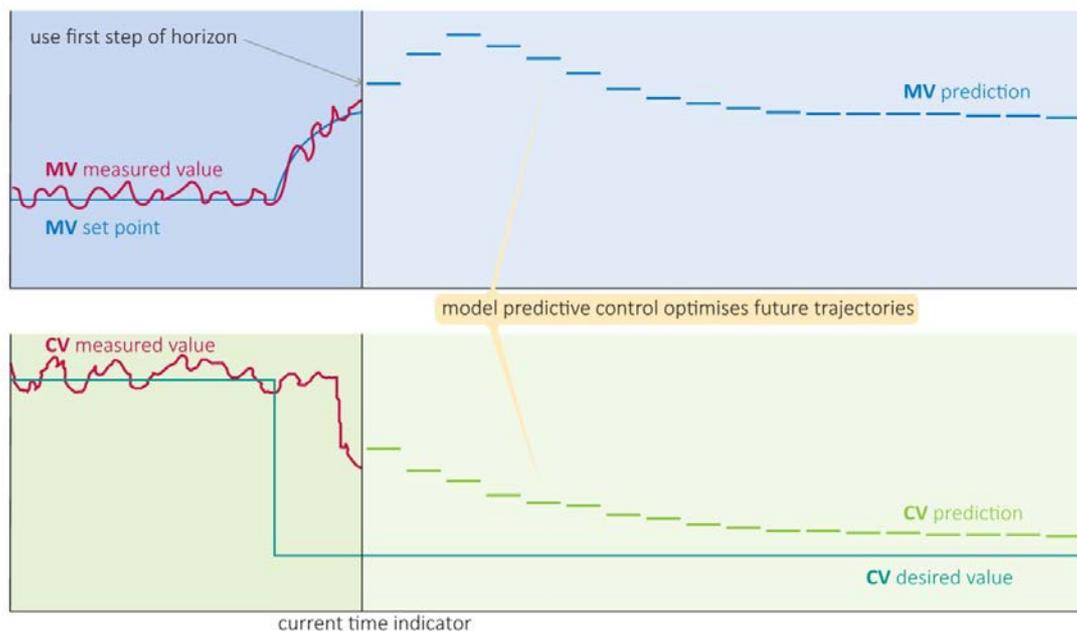
**Figure 7** Illustration of model predictive control (MV, manipulated variable; CV, controlled variable) (James, 2011)
