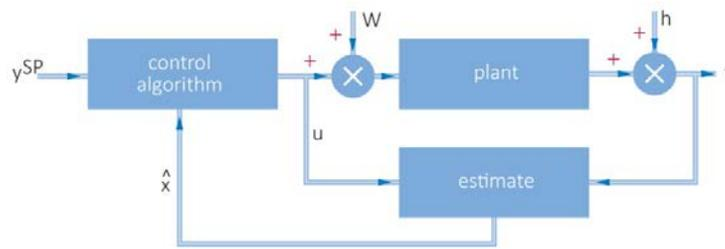
Figure 17 The controller model used by Predict & Control (ABB, 2006c)
