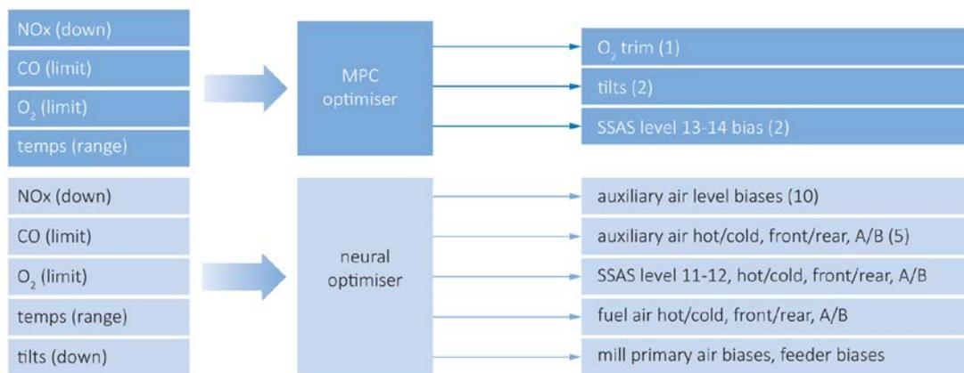
**Figure 16** Division of control tasks between the MPC and neural network components of CombustionOpt (SSAS, superheat steam attemperation spray) (James and Spinney, 2011)
