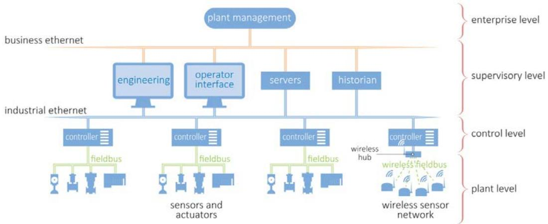
Figure 3 A typical DCS architecture
