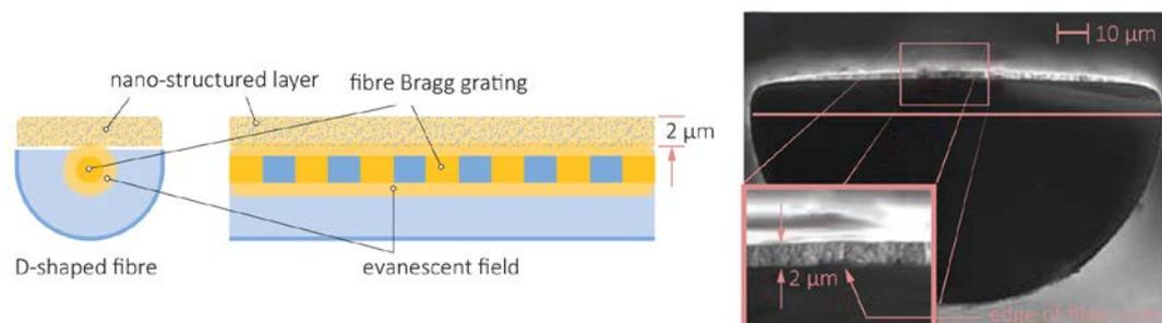
Figure 22 A D-shaped fibre modified with a gas-sensitive ceramic film (Chen, 2014)
