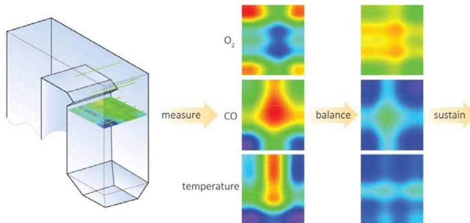
**Figure 13** 2D profiles of the boiler parameters generated by the ZoloBOSS system are used to balance combustion across the furnace (Stewart and others, 2012)
