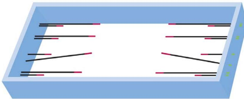
Figure 11 The grid placement of O<sub>2</sub>/CO sensors in Delta CCM (Ferri, 2015)
