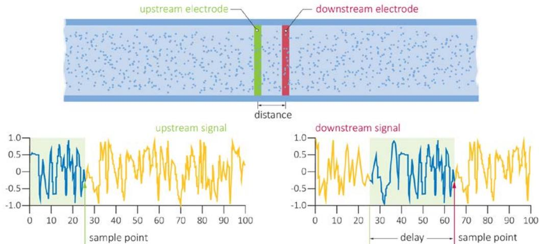
**Figure 14** Measurement of coal flow by cross-correlation of electrostatic charge signals (Coombes, 2014)
