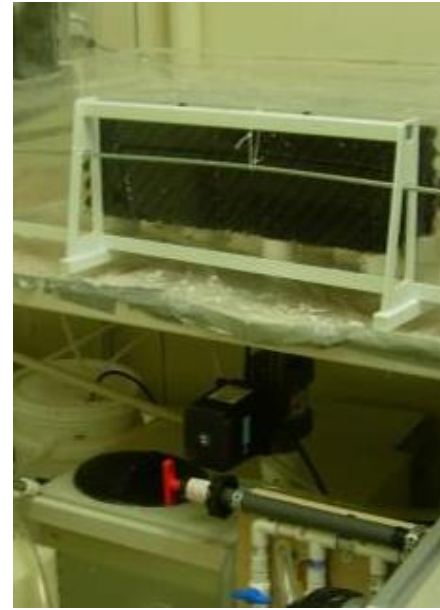
2010: Lab air contactor
