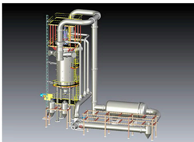
Figure 20 Schematic showing part of the 50 MWth large pilot engineering package developed for Sotacarbo's CO 2 Technology Centre Sulcis for Zero Emission (photograph courtesy of ITEA)
