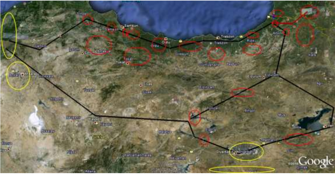
Figure 2: The basic transmission routes related to Georgia Interconnection (blue line: Muratli – Batumi line representation; red line: Borcka – Akhaltsikhe line representation, black lines: expected transmission highways in 2013, red circles: major generating facilities, yellow circles: major load centers).
