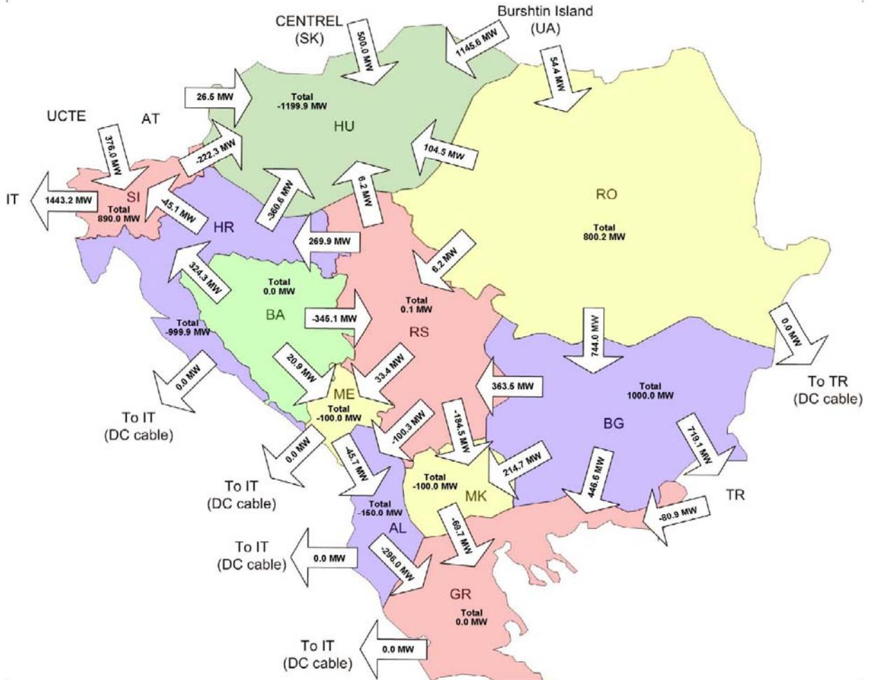
Figure 13.16.2: Aggregated border flows in area of SEE in winter maximum 2020, scenario when power system of Serbia is self-balanced
