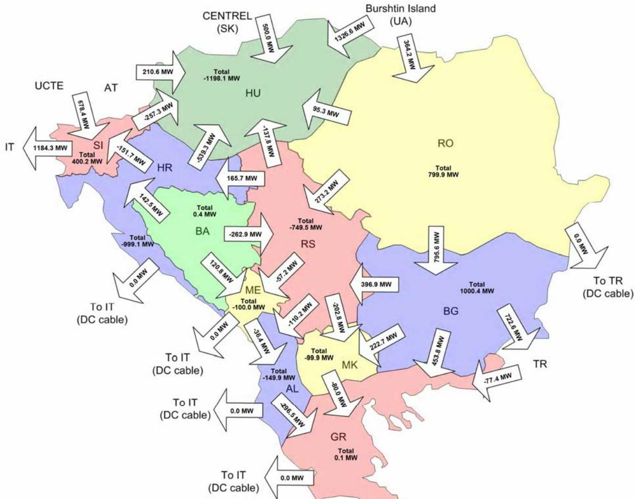
Figure 13.17.2: Aggregated border flows in area of SEE in winter maximum 2020, scenario when power system of Slovenia exports 400 MW
