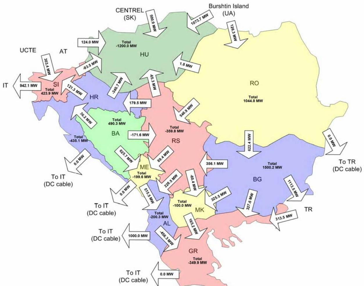
Figure 13.5.1: Aggregated border flows in area of SEE in winter maximum 2015, scenario Bulgaria and Romania export 1000 MW to Italy via HVDC link Albania–Italy
