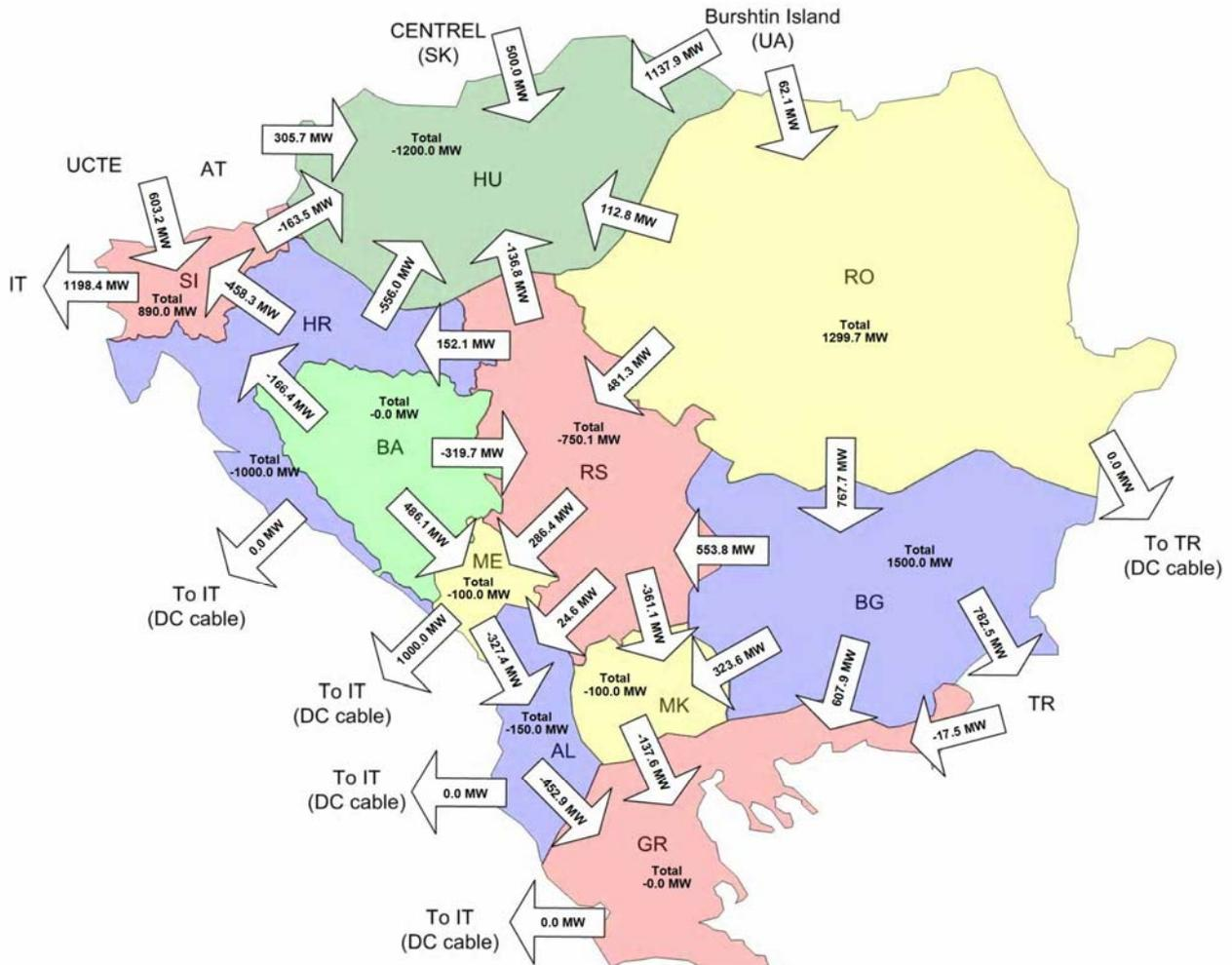
Figure 13.6.2: Aggregated border flows in area of SEE in winter maximum 2015, scenario Bulgaria and Romania export 1000 MW to Italy via HVDC link Montenegro –Italy
