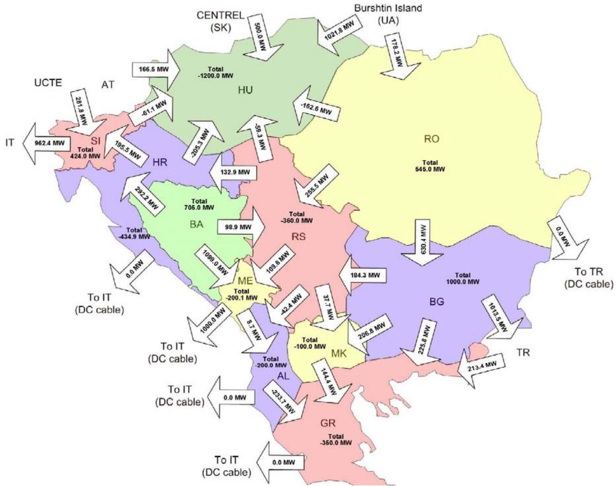
Figure 13.6.3: Aggregated border flows in area of SEE in winter maximum 2015, scenario export of 1000 MW from BiH to Italy via HVDC link Montenegro – Italy
