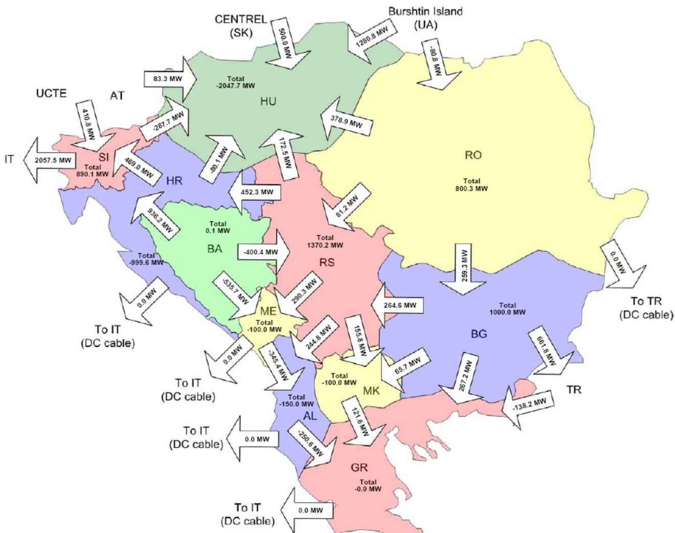
Figure 13.1.2: Aggregated border flows in area of SEE in winter maximum 2015, scenario TPP Kosovo C exports 2120 MW to Italy and CENTREL
