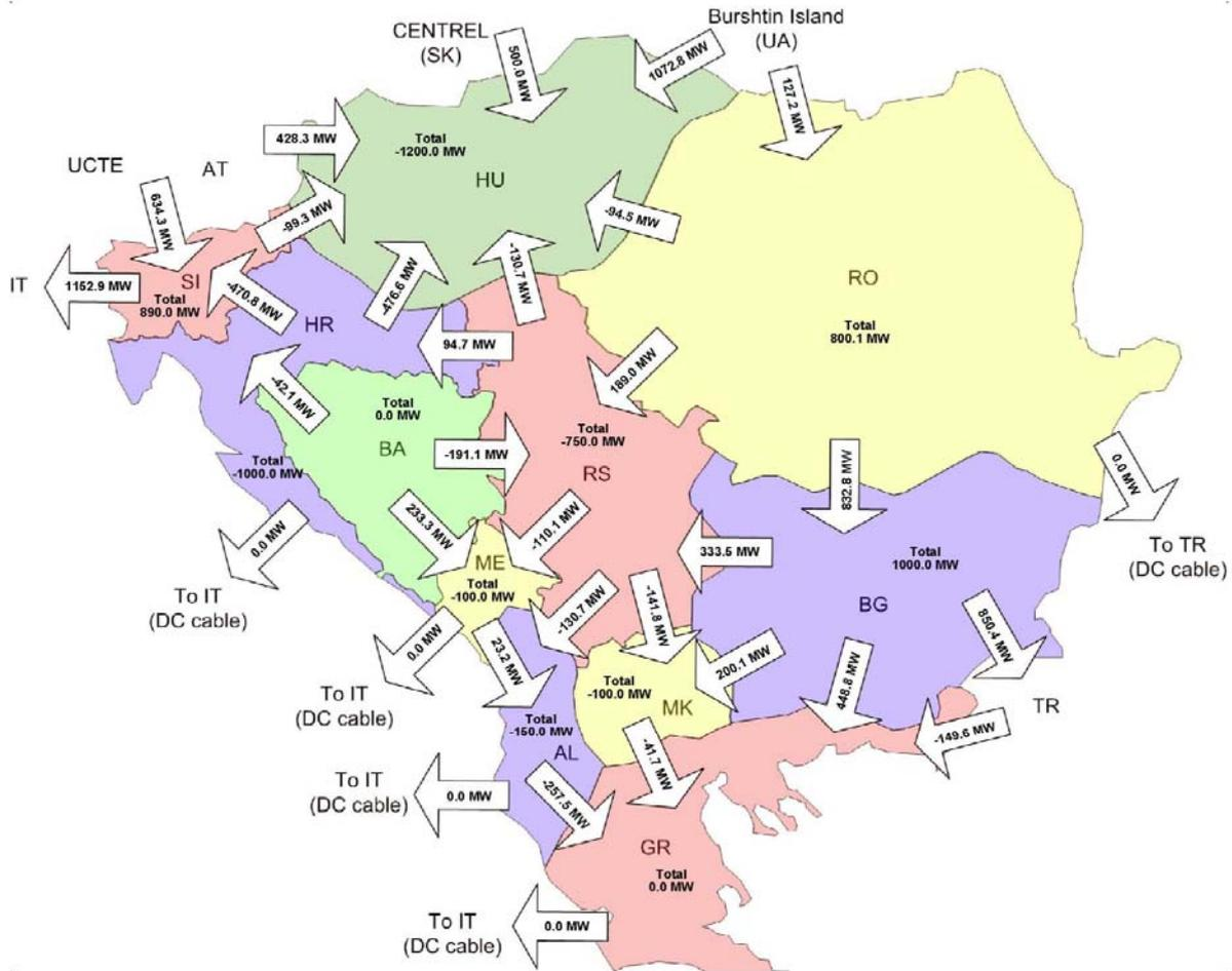
Figure 13.18.4: Aggregated border flows in area of SEE in winter maximum 2020, scenario when power system of Turkey imports 1000 MW
