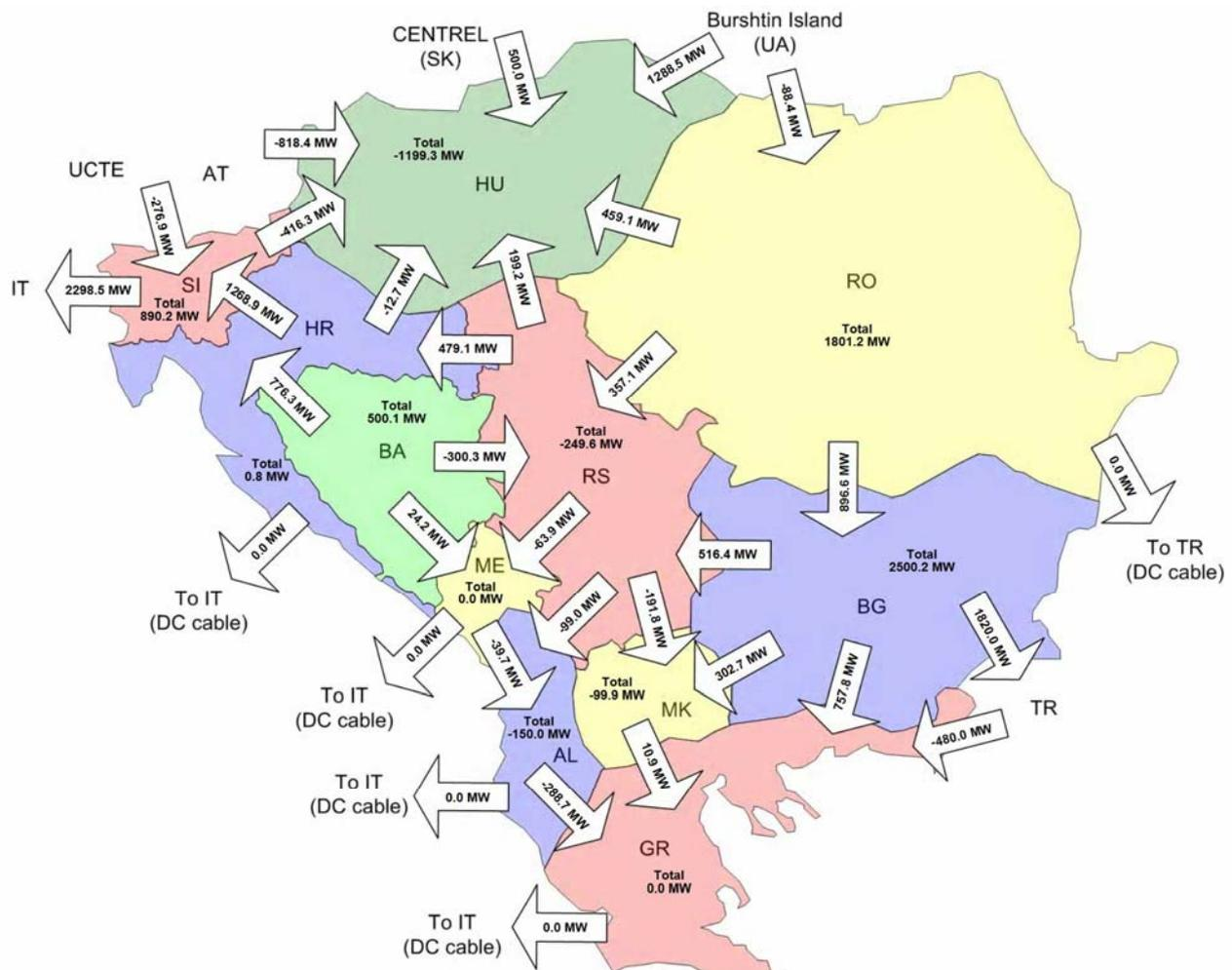
Figure 13.4.2: Aggregated border flows in area of SEE in winter maximum 2020, scenario WPPs export 4600 MW to Italy, Turkey and CENTREL
