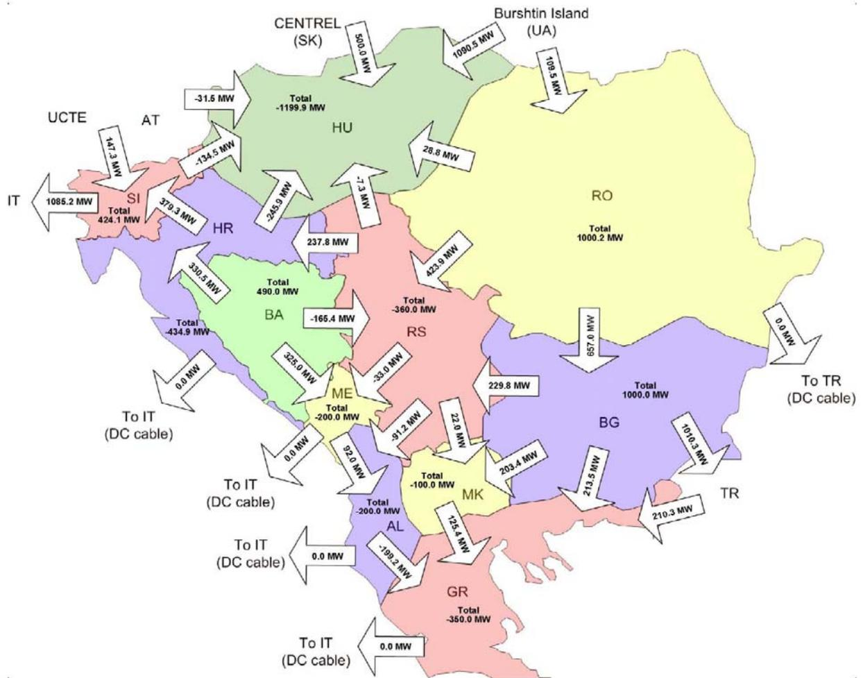
Figure 13.15.3: Aggregated border flows in area of SEE in winter maximum 2015, scenario when power system of Romania exports 1000 MW
