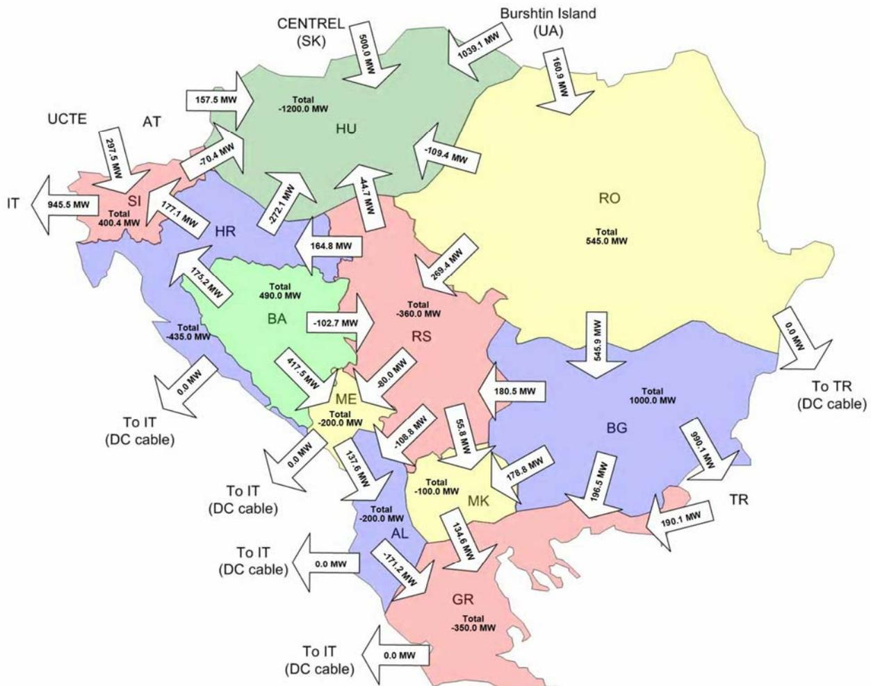
Figure 13.17.2: Aggregated border flows in area of SEE in winter maximum 2015, scenario when power system of Slovenia exports 400 MW
