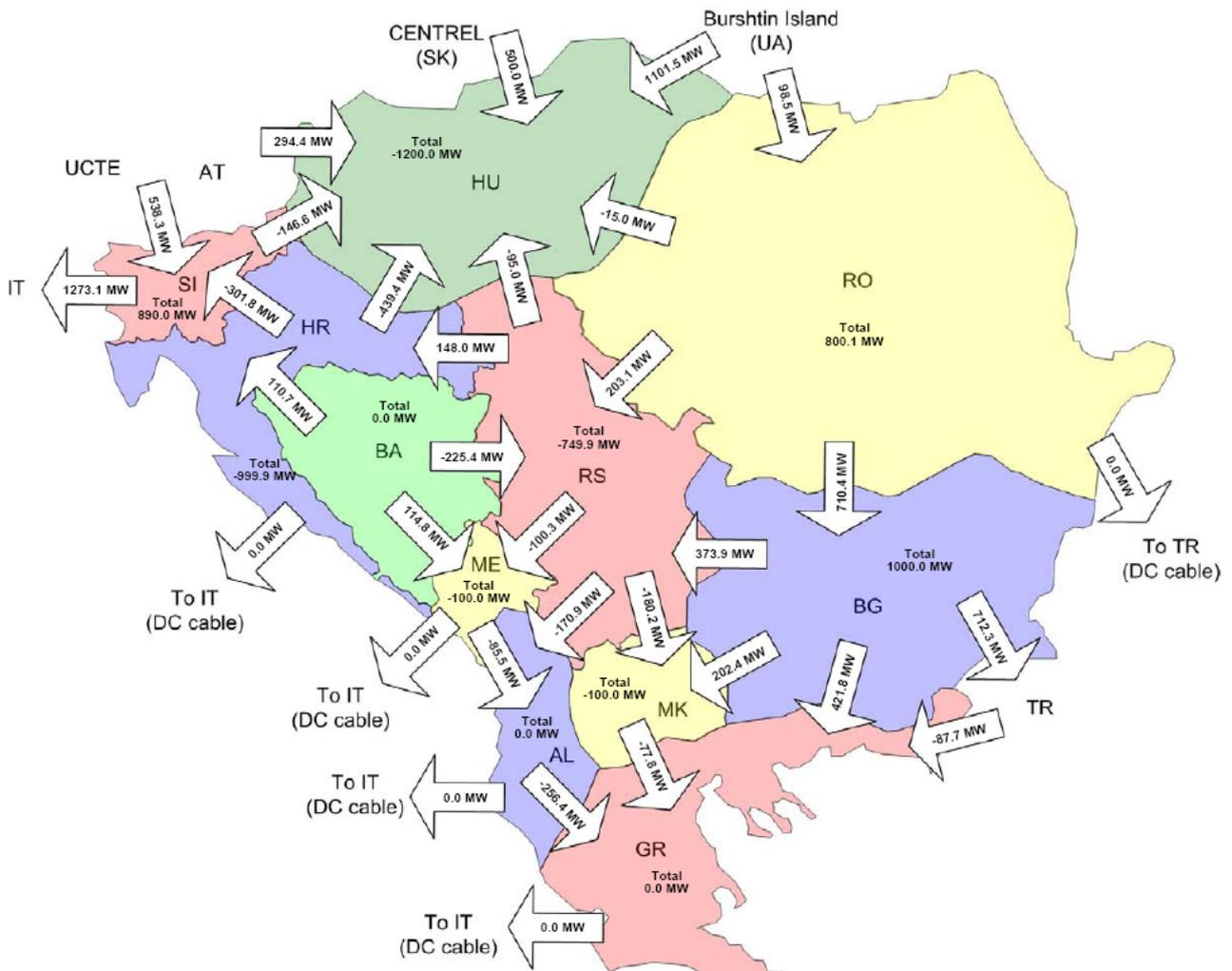
Figure 13.9.2: Aggregated border flows in area of SEE in winter maximum 2020, scenario when power system of Albania is self-balanced
