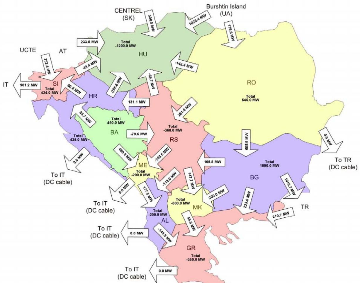
Figure 13.13.3: Aggregated border flows in area of SEE in winter maximum 2015, scenario when power system of Macedonia imports 300MW
