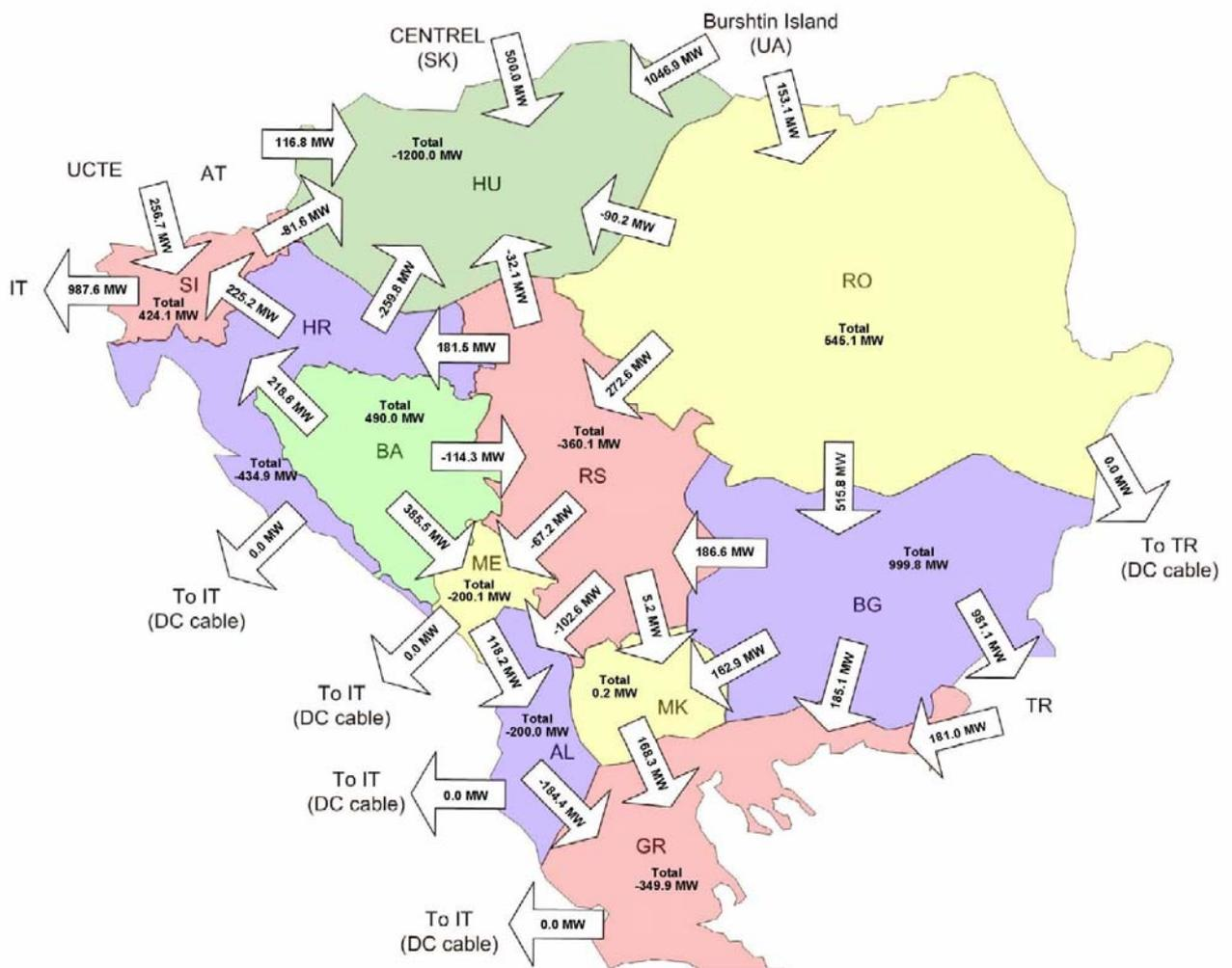
Figure 13.13.1: Aggregated border flows in area of SEE in winter maximum 2015, scenario when power system of Macedonia is self-balanced
