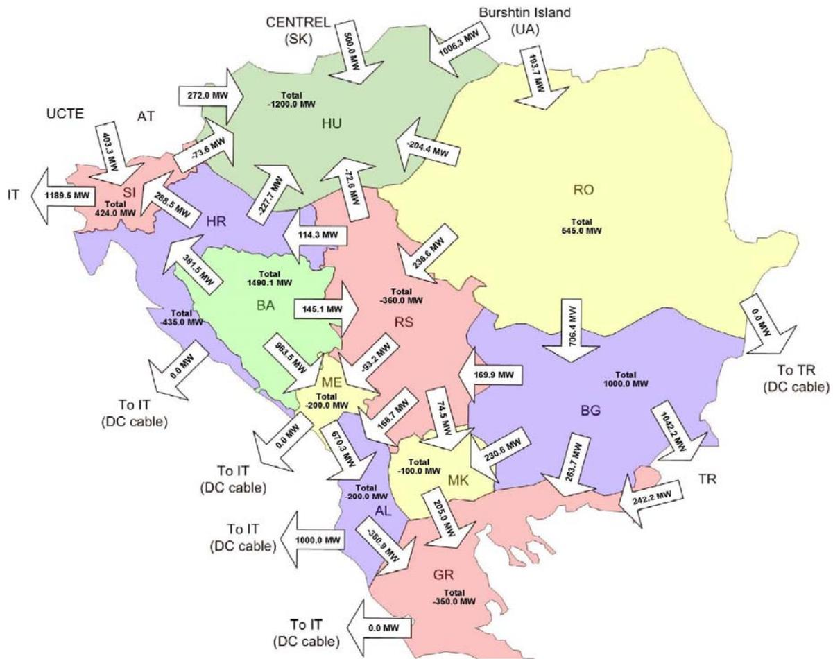
Figure 13.5.3: Aggregated border flows in area of SEE in winter maximum 2015, scenario export of 1000 MW from BiH to Italy via HVDC link Albania – Italy
