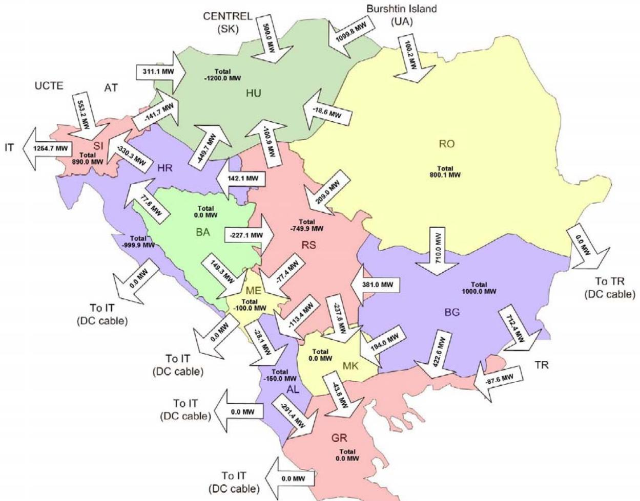
Figure 13.13.2: Aggregated border flows in area of SEE in winter maximum 2020, scenario when power system of Macedonia is self-balanced
