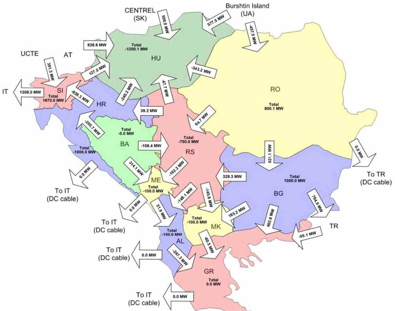
Figure 13.2.2: Aggregated border flows in area of SEE in winter maximum 2020, scenario NPP Krsko 2 exports 1080 MW to Italy
