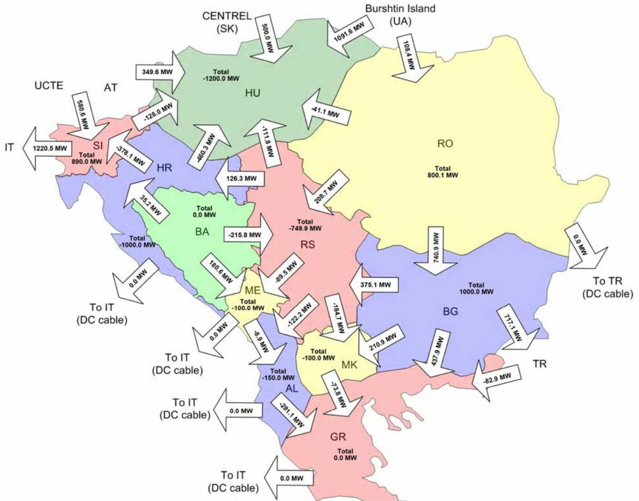
Figure 13.11.2: Aggregated border flows in area of SEE in winter maximum 2020, scenario when power system of BiH is self-balanced
