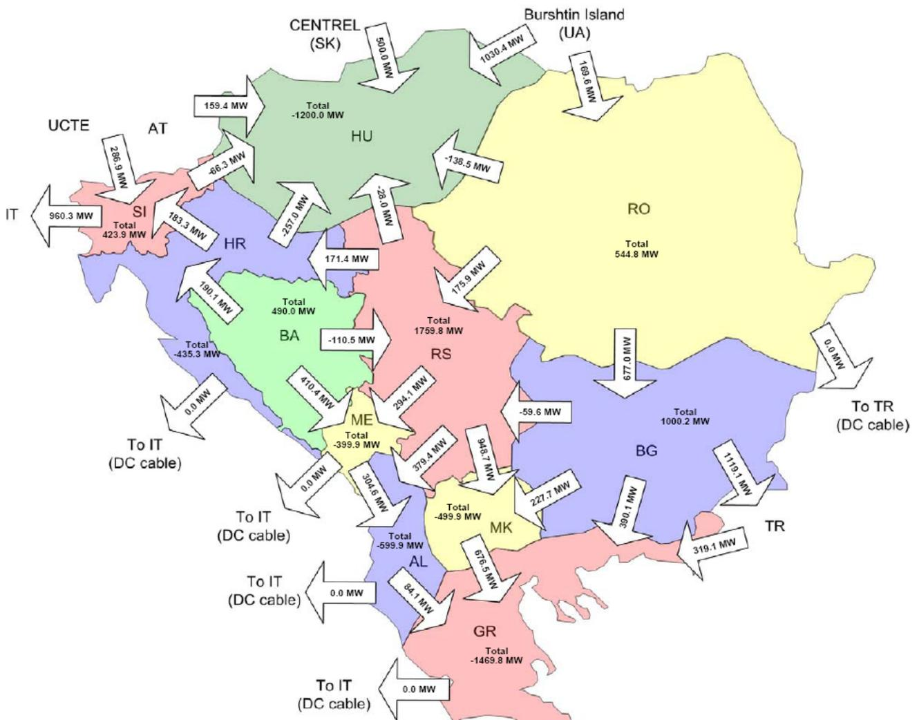
Figure 13.1.3: Aggregated border flows in area of SEE in winter maximum 2015, scenario TPP Kosovo C exports 2120 MW to Montenegro, Albania, Macedonia and Greece
