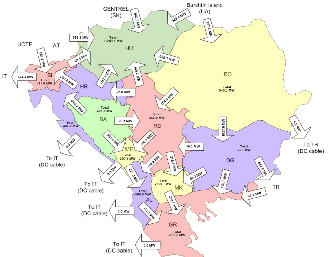
Figure 13.10.1: Aggregated border flows in area of SEE in winter maximum 2015, scenario when power system of Bulgaria is self-balanced
