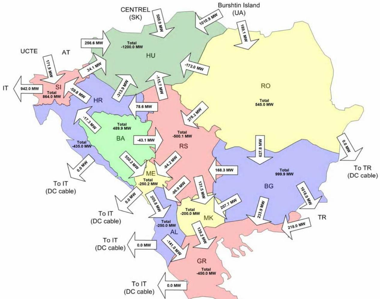
Figure 13.3.3: Aggregated border flows in area of SEE in winter maximum 2015, scenario PSHP Kozjak exports 440 MW to Montenegro, Albania, Macedonia, Serbia, UNMIK and Greece
