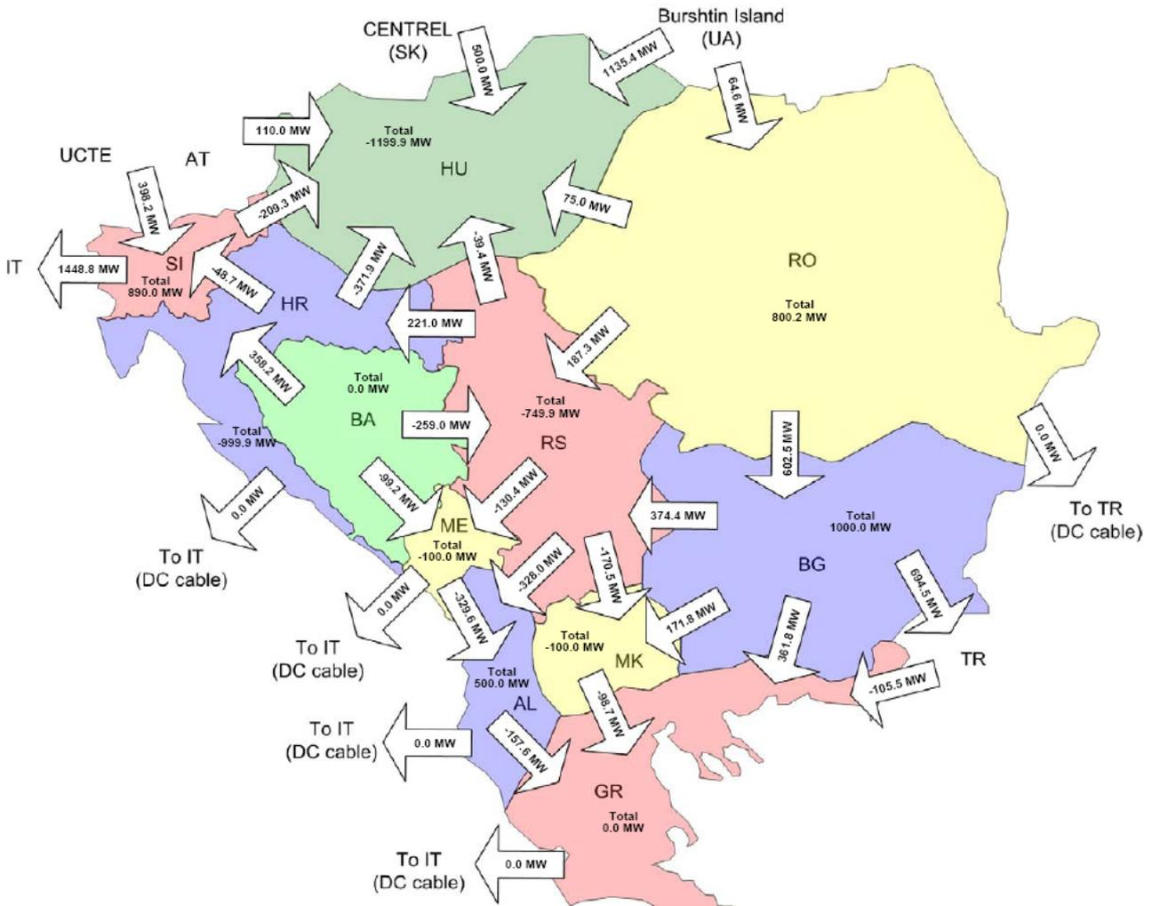
Figure 13.9.4: Aggregated border flows in area of SEE in winter maximum 2020, scenario when power system of Albania exports 500 MW
