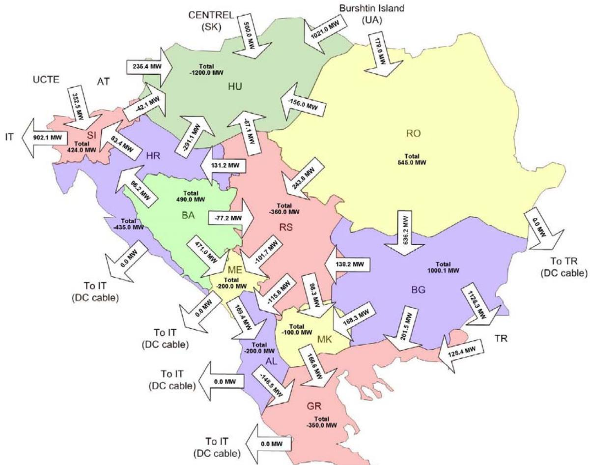
Figure 13.18.3: Aggregated border flows in area of SEE in winter maximum 2015, scenario when power system of Turkey imports 1000 MW
