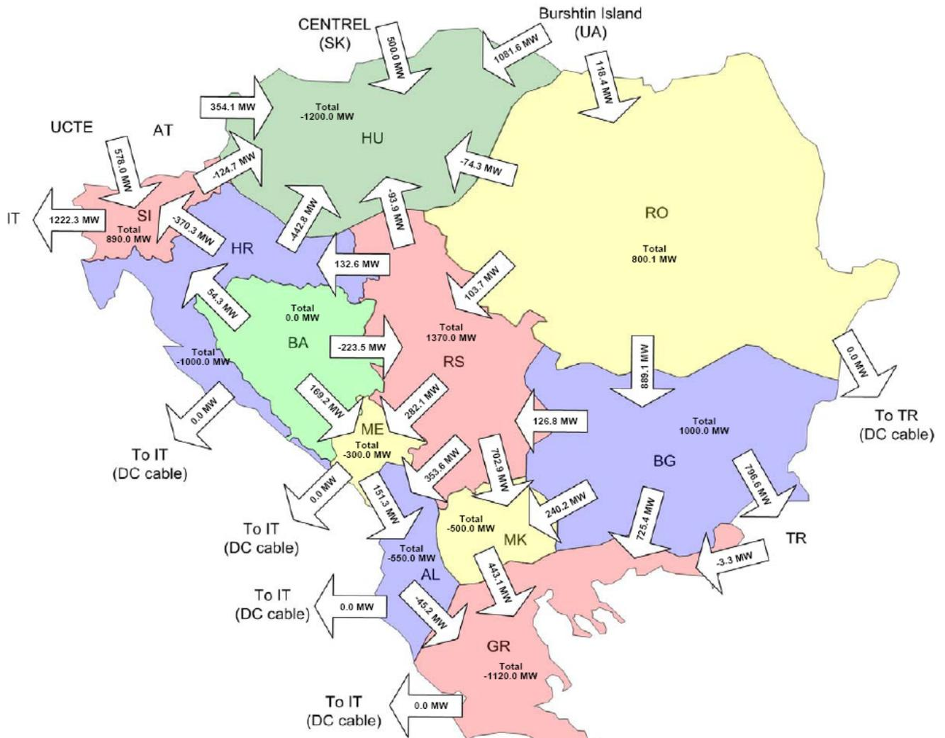
Figure 13.1.4: Aggregated border flows in area of SEE in winter maximum 2015, scenario TPP Kosovo C exports 2120 MW to Montenegro, Albania, Macedonia and Greece
