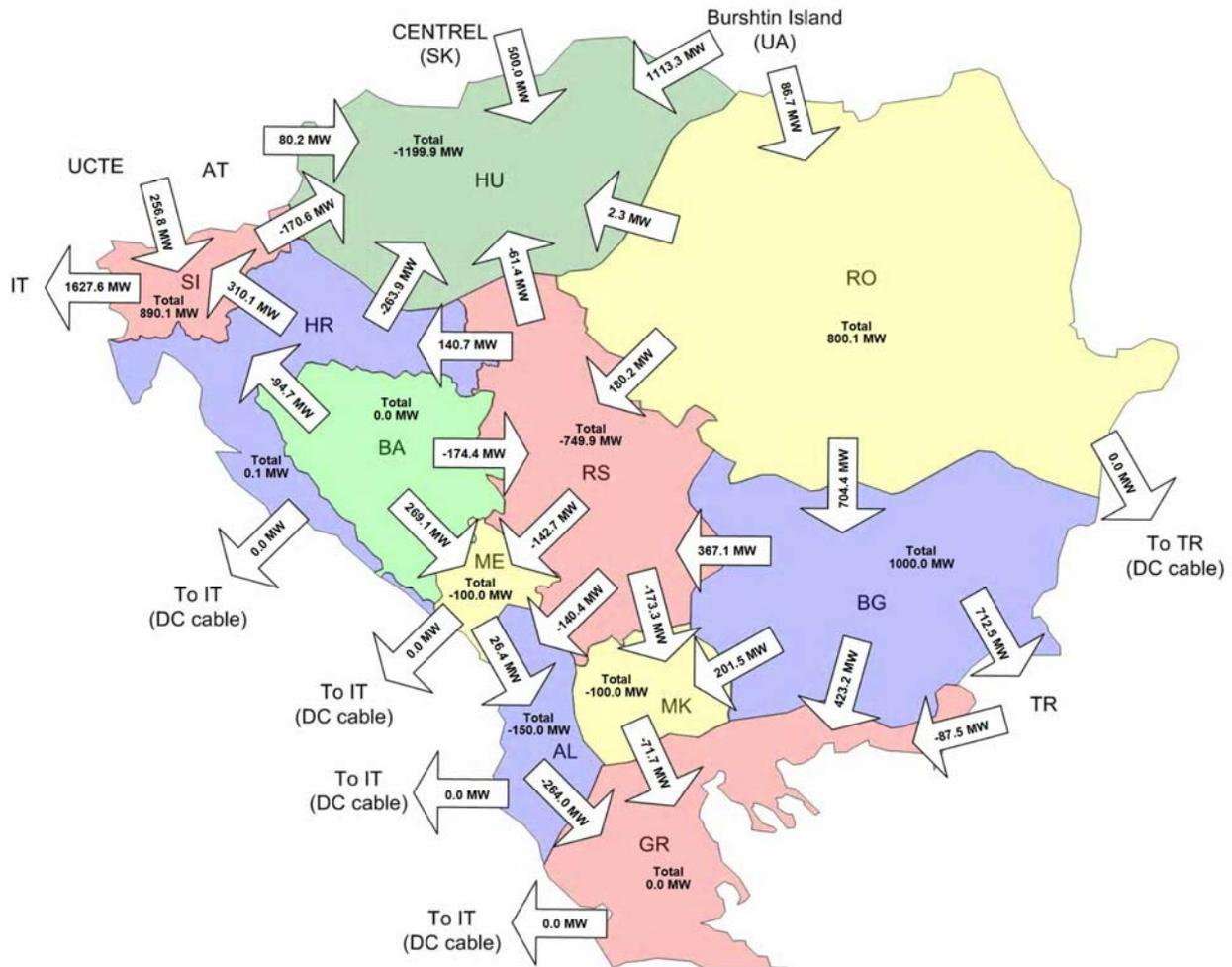
Figure 13.12.2: Aggregated border flows in area of SEE in winter maximum 2020, scenario when power system of Croatia is self-balanced
