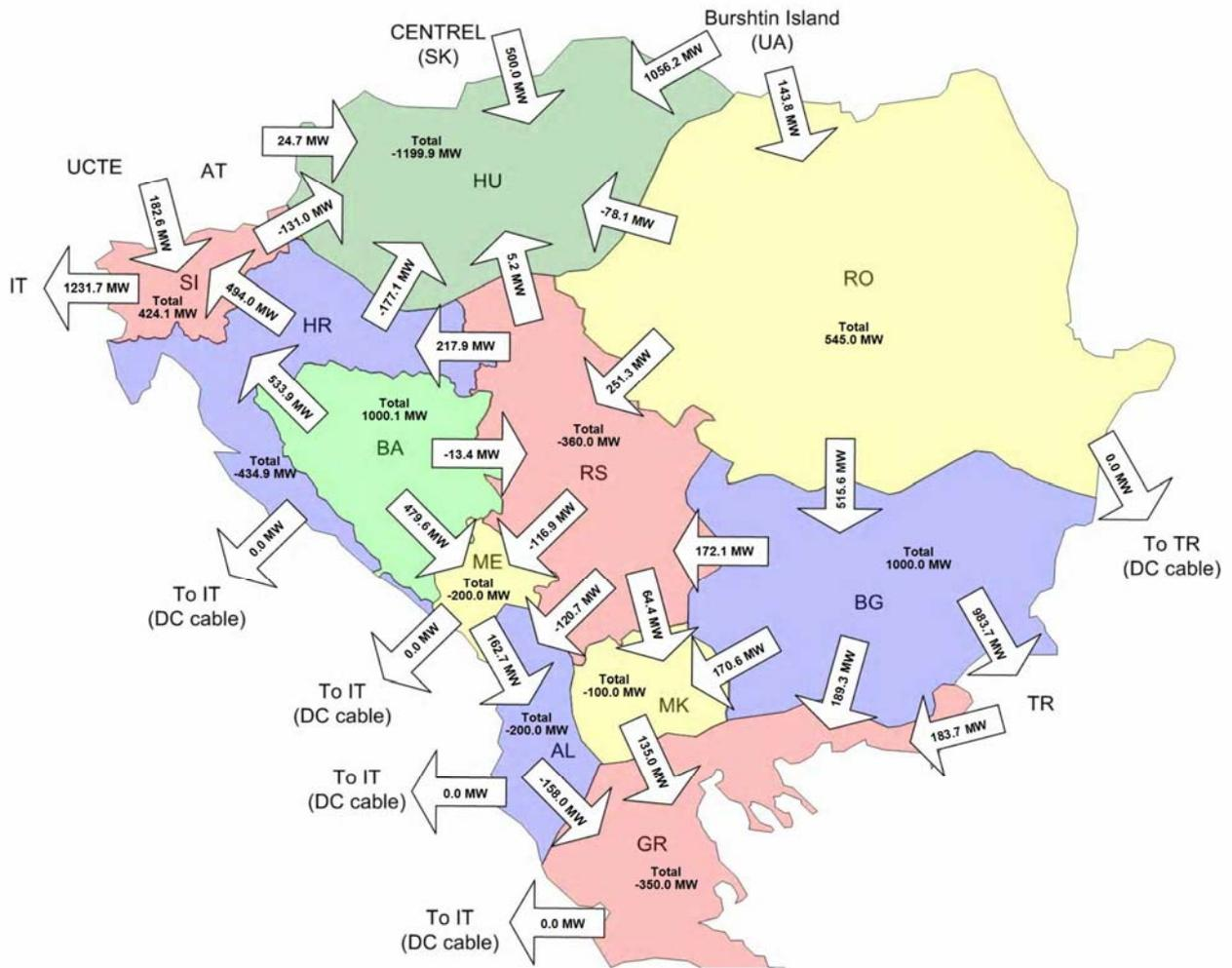
Figure 13.11.3: Aggregated border flows in area of SEE in winter maximum 2015, scenario when power system of BiH exports 1000 MW
