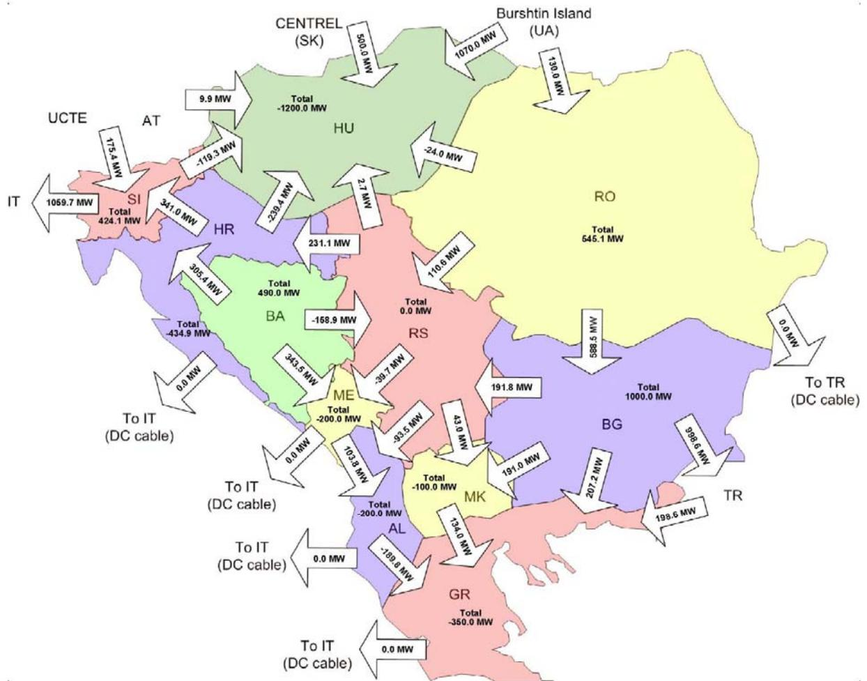
Figure 13.16.1: Aggregated border flows in area of SEE in winter maximum 2015, scenario when power system of Serbia is self-balanced
