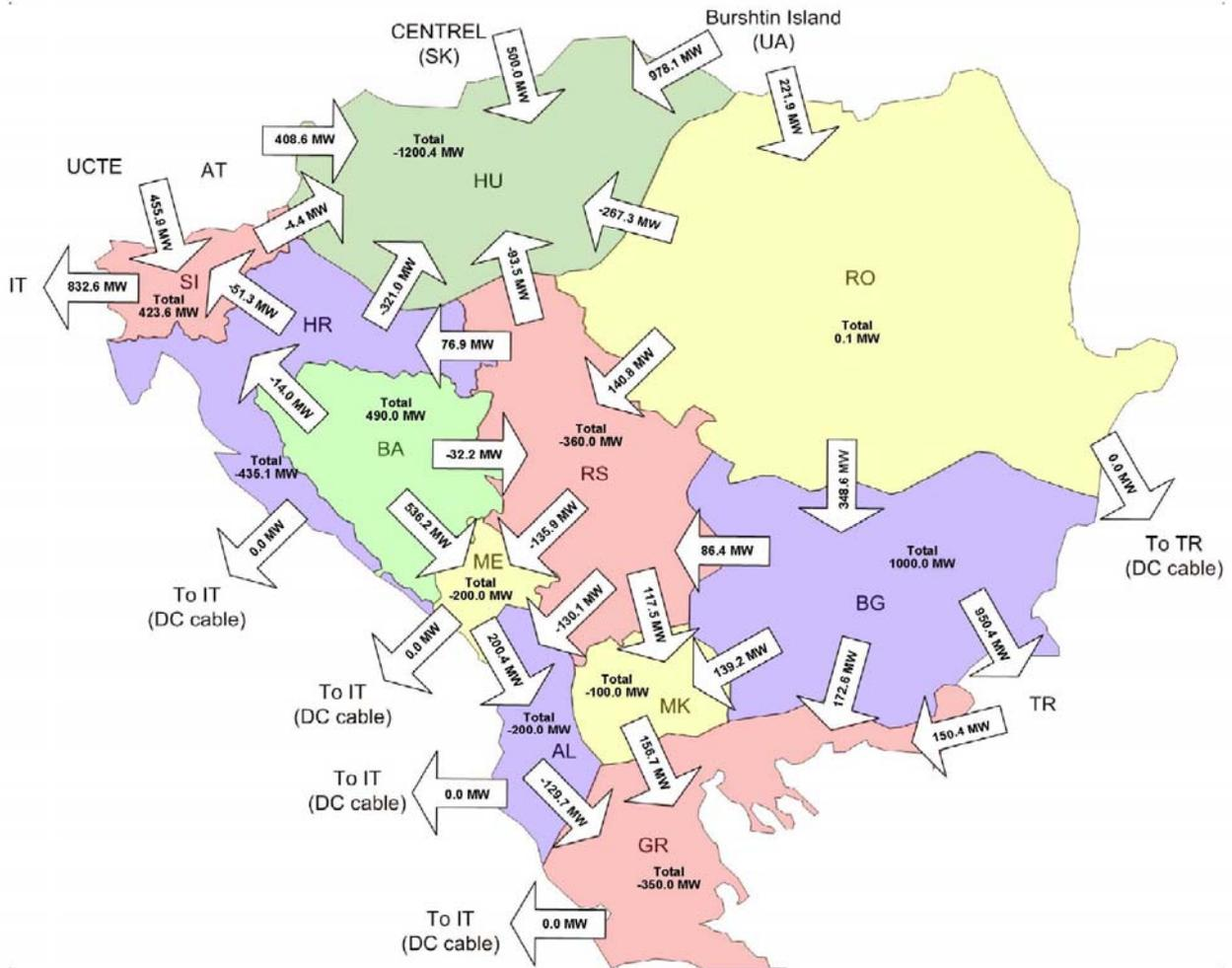
Figure 13.15.1: Aggregated border flows in area of SEE in winter maximum 2015, scenario when power system of Romania is self-balanced
