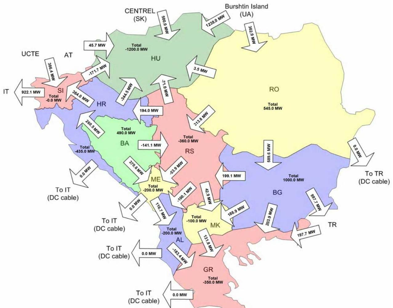
Figure 13.17.1: Aggregated border flows in area of SEE in winter maximum 2015, scenario when power system of Slovenia is self-balanced
