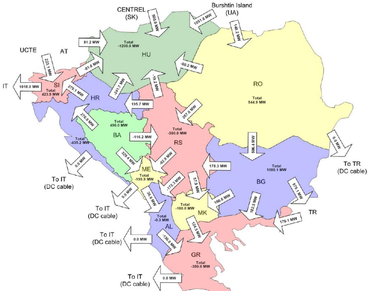
Figure 13.9.1: Aggregated border flows in area of SEE in winter maximum 2015, scenario when power system of Albania is self-balanced
