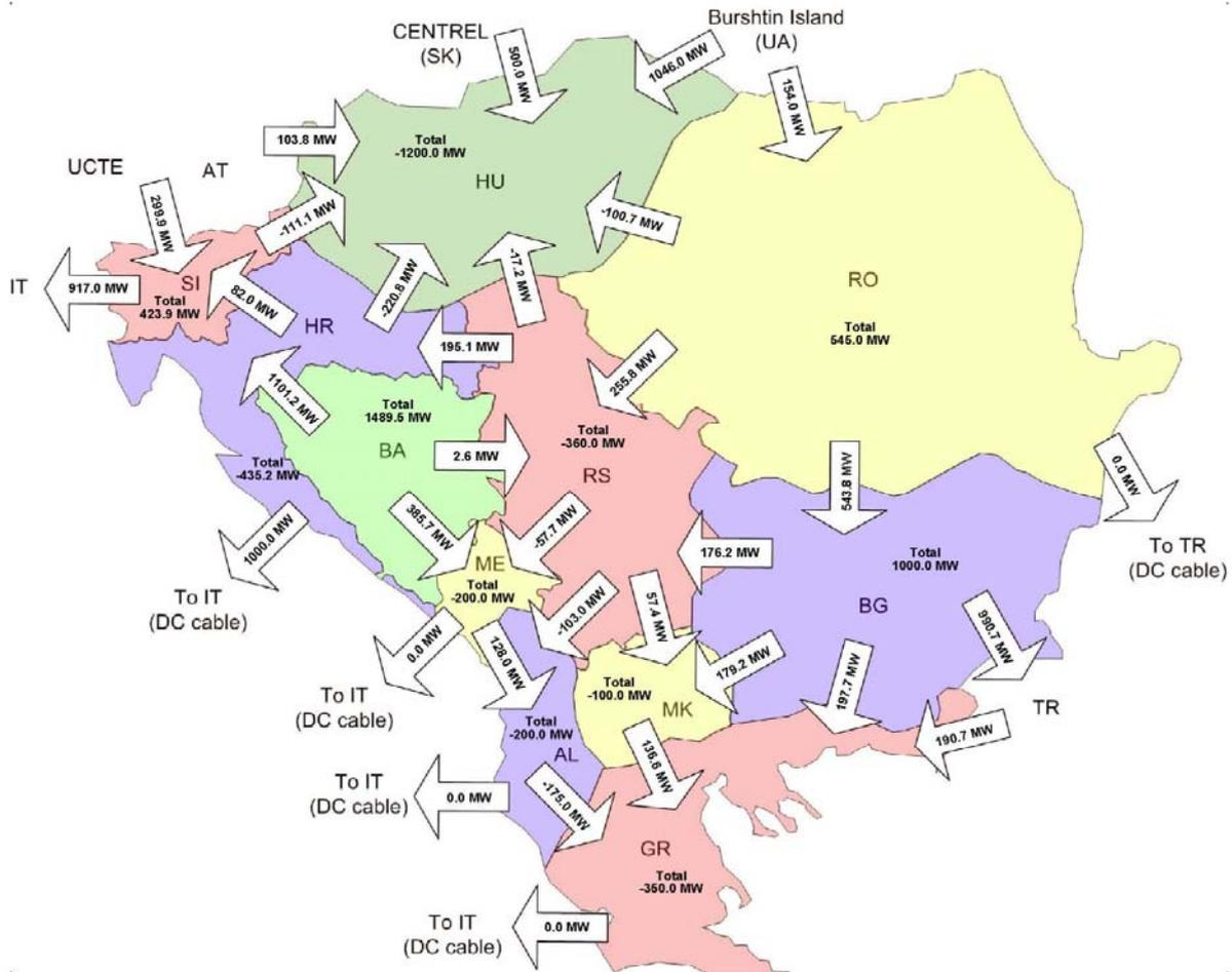
Figure 13.7.3: Aggregated border flows in area of SEE in winter maximum 2015, scenario export of 1000 MW from BiH to Italy via HVDC link Croatia – Italy
