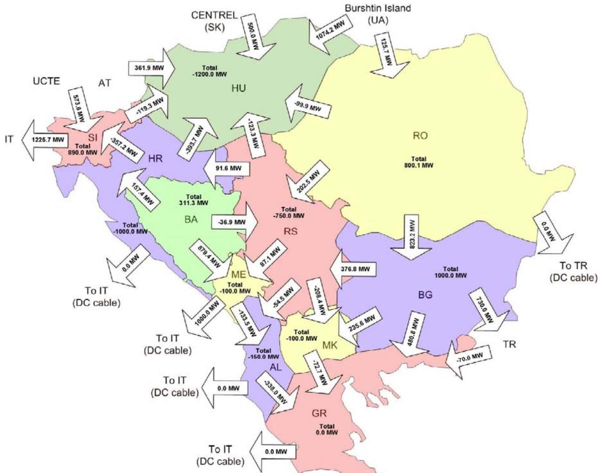
Figure 13.6.4: Aggregated border flows in area of SEE in winter maximum 2020, scenario export of 1000 MW from BiH to Italy via HVDC link Montenegro – Italy
