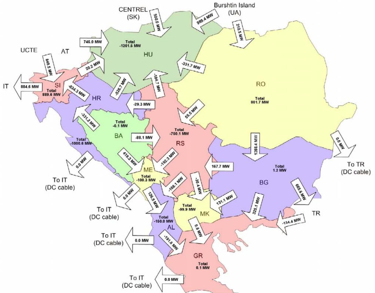
Figure 13.10.2: Aggregated border flows in area of SEE in winter maximum 2020, scenario when power system of Bulgaria is self-balanced
