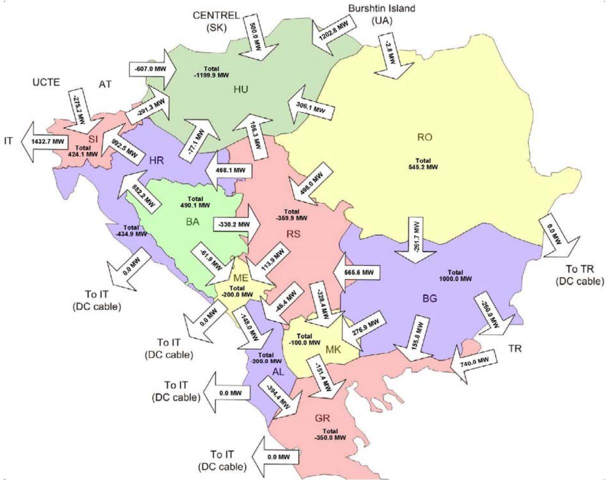
Figure 13.18.1: Aggregated border flows in area of SEE in winter maximum 2015, scenario when power system of Turkey exports 1000 MW
