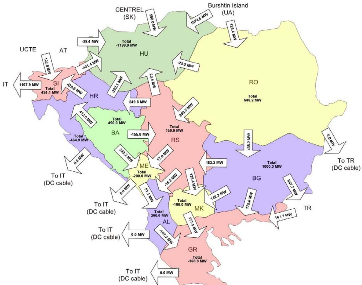
Figure 13.19.1: Aggregated border flows in area of SEE in winter maximum 2015, scenario when power system of UNMIK zone is self-balanced
