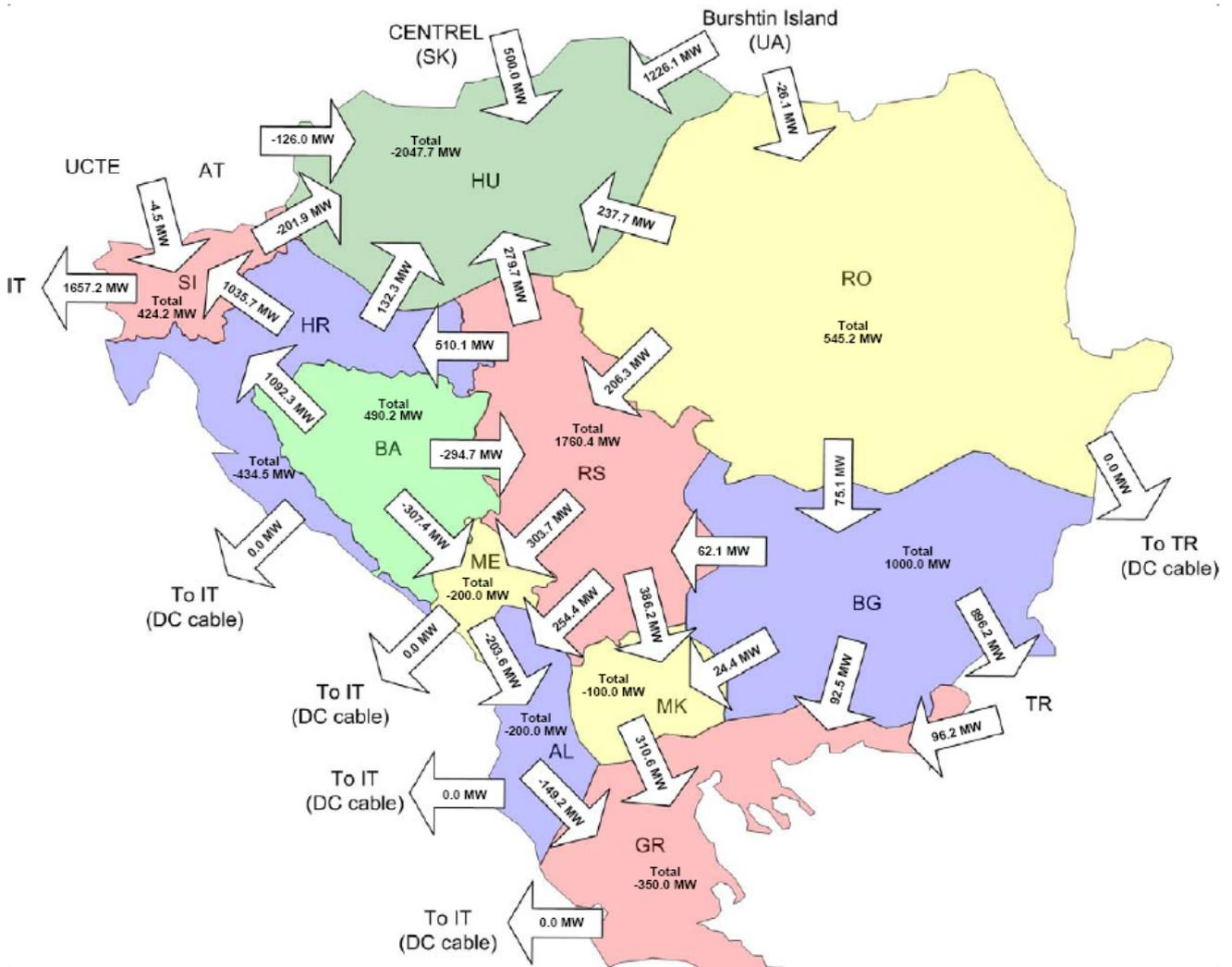
Figure 13.1.1: Aggregated border flows in area of SEE in winter maximum 2015, scenario TPP Kosovo C exports 2120 MW to Italy and CENTREL
