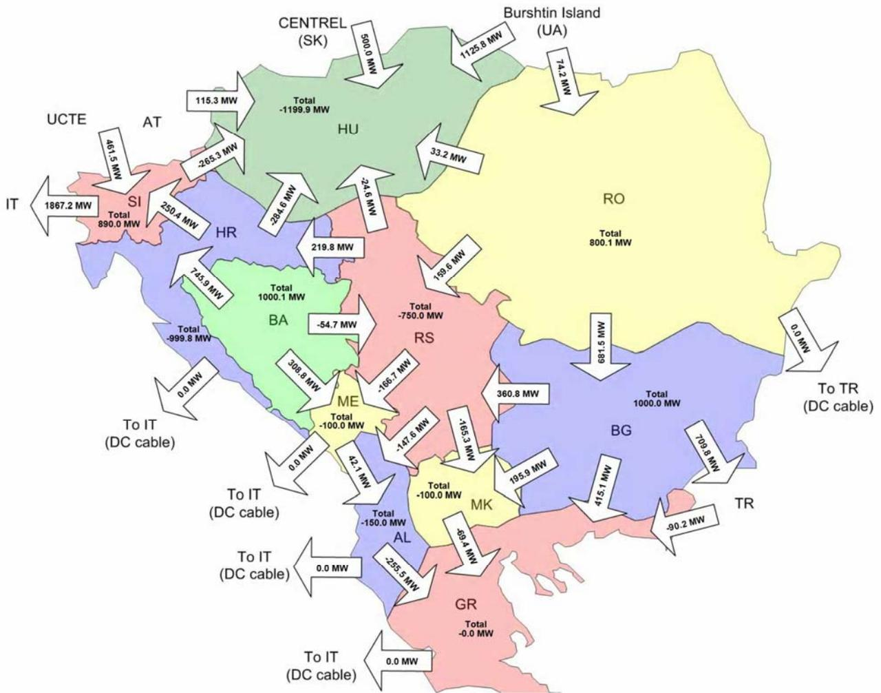
Figure 13.11.4: Aggregated border flows in area of SEE in winter maximum 2020, scenario when power system of BiH exports 1000 MW
